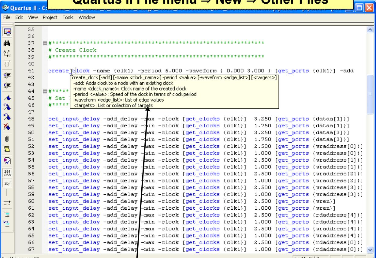
The screenshot shows the Quartus II Text Editor window with an SDC file open. The file contains various commands for creating clocks and setting input delays. A tooltip is displayed over the 'create\_clock' command, providing its definition: '# Create Clock'. The tooltip is enclosed in a yellow box with a black border. The cursor is positioned over the 'create\_clock' command. The Quartus II interface includes a toolbar on the left, a menu bar at the top, and status bars at the bottom.
