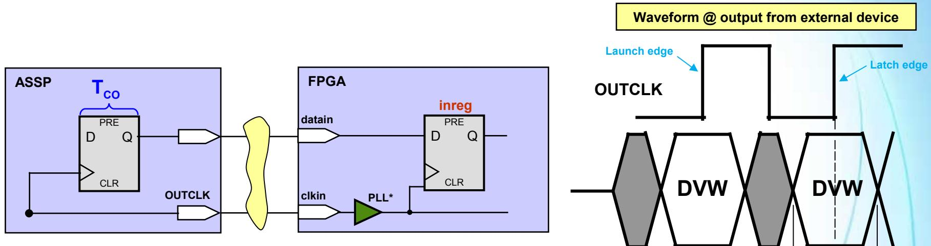
$$\begin{aligned} \text{input delay min} &= \text{board delay (min)} - \text{clock delay (max)} + T_{co(min)} \\ &= T_{co(min)} \end{aligned}$$
