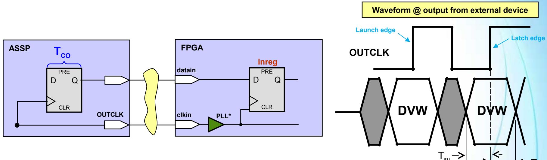
input delay max  $= \text{board delay (max)} - \text{clock delay (min)} + T_{co(\max)}$
