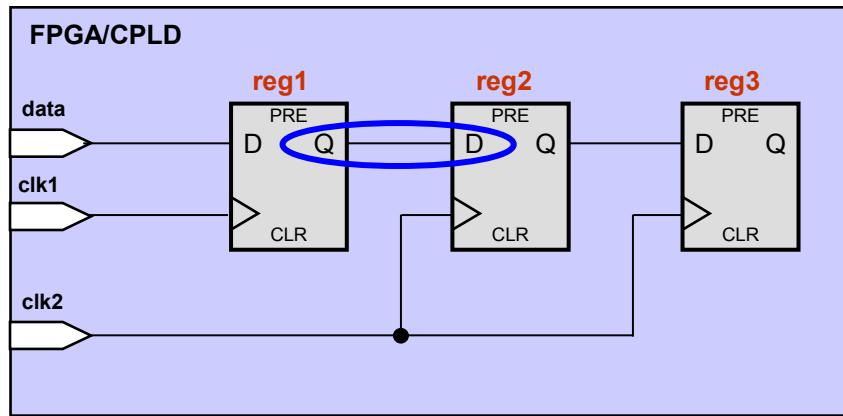
Simple synchronizer circuit between two asynchronous clock domains
