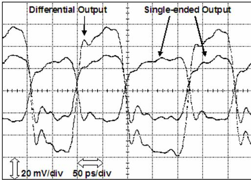
Fig. 5. Measured output waveforms of the comparator with a 5 GHz input oversampled at 32 GS/s (20 mV/div, 50 ps/div).
