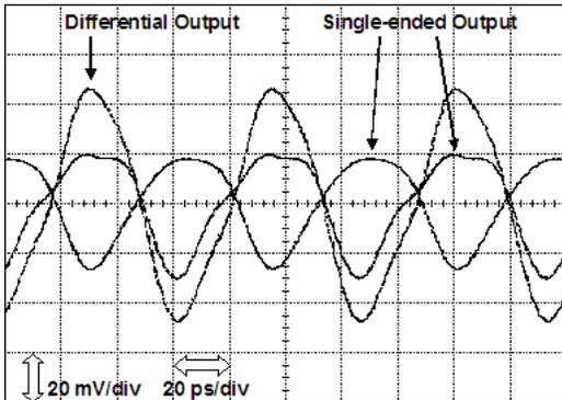
Fig. 6. Measured output waveforms of the comparator operating at Nyquist with a sampling rate of 30 GS/s (20 mV/div, 20 ps/div).
