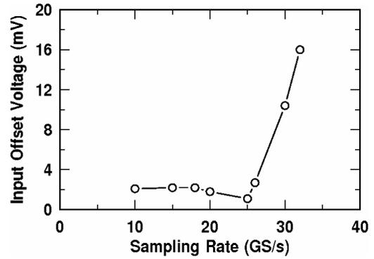
Fig. 7. Measured input offset voltage of the comparator as a function of sampling rate.
