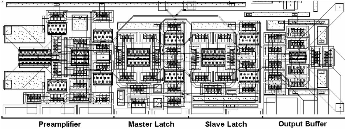
Fig. 3. Symmetrical and compact layout of the preamplifier, master latch, slave latch, and output buffer, occupying  $210 \times 62 \mu\text{m}^2$ .
