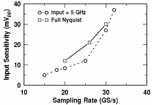
Fig. 8. Measured input sensitivity of the comparator as a function of sampling rate.
