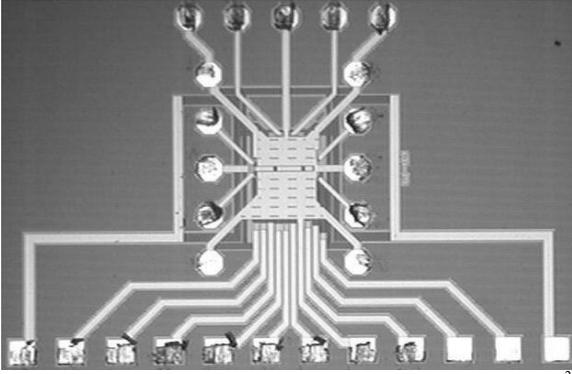
Fig. 4. Chip micrograph of the comparator, occupying  $1731 \times 1141 \mu\text{m}^2$ .
