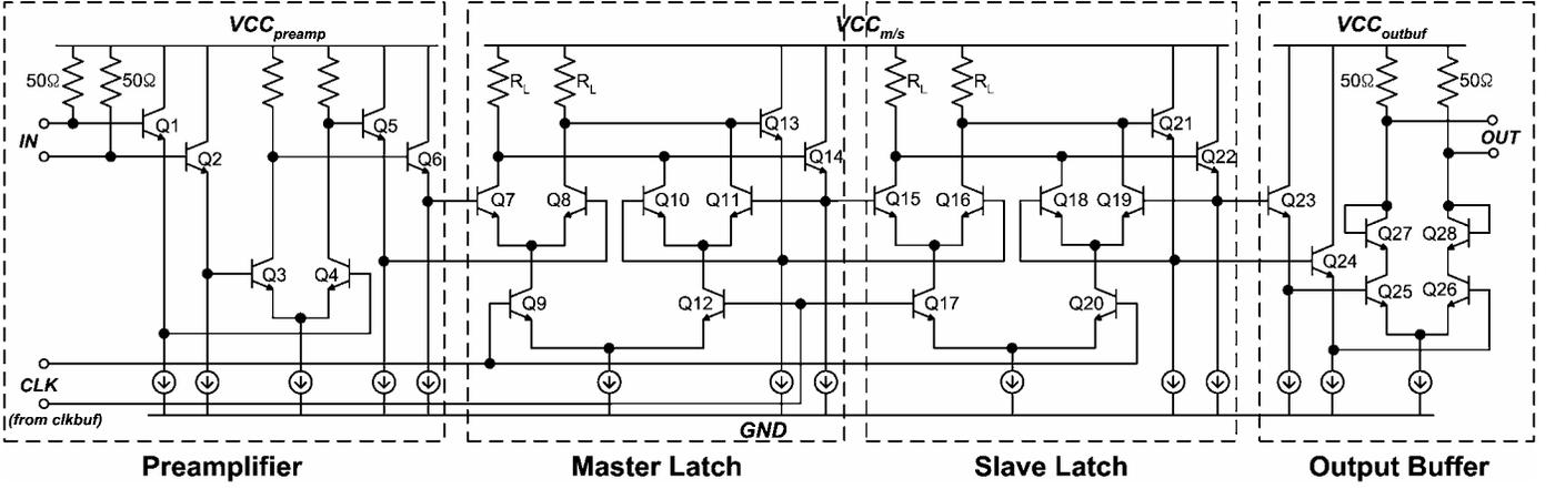
Fig. 2. Schematic of the preamplifier, master latch, slave latch, and output buffer.
