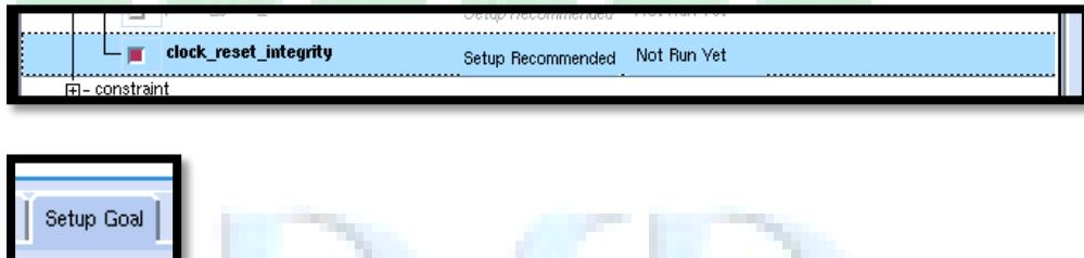
7. Run Setup Wizard for setup “clock\_reset\_integrity” goal
