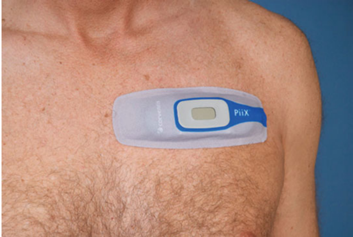
Fig. 1.5 Corventis company's wearable bandage-like ECG device [31]
