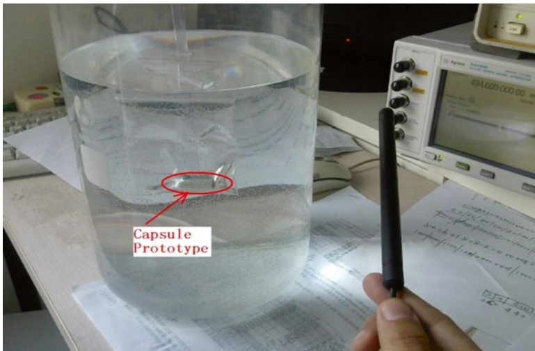
Fig. 4.16 Capsule endoscope prototype with designed 400 MHz transceiver in emulated environment
