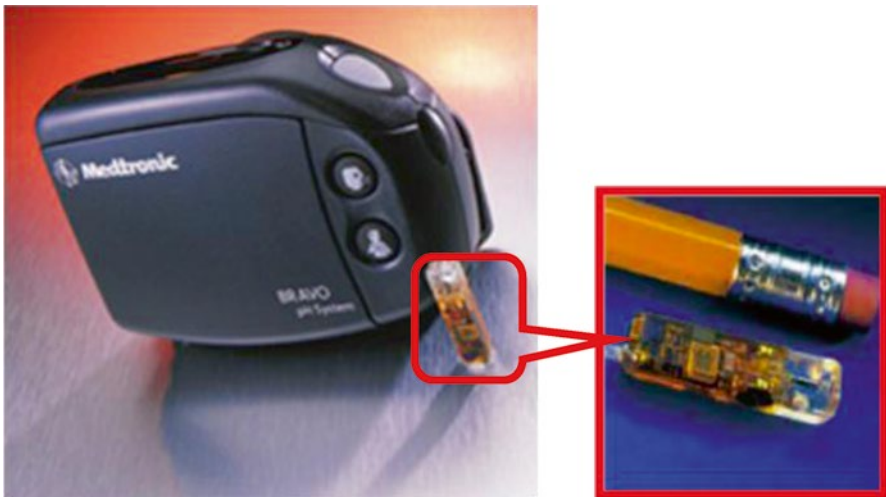
Fig. 3.3 Bravo® pH monitoring system including the pH capsule the portable data receiver, originally manufactured by Medtronic, now acquired by Given Imaging. The pH capsule containing the pH sensor is shown on the right side. The pictures are available online http://www.digestivehealthcare.com/bravo_ph.html
