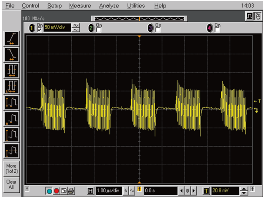
Fig. 4.9 Measured 20 MHz ASK signal with 1 Mbps data
