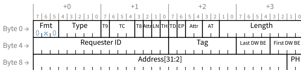
Figure 2-18 Request Header Format for 32-bit Addressing of Memory
