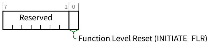
Figure 7-299 Conventional PCI Advanced Features Control Register
