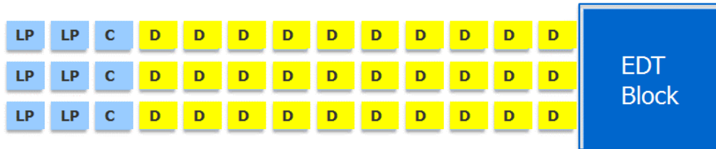
Figure 7-2. Non-Separated Control Data Input Channels
