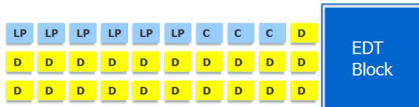
Figure 7-3. Separated Control Data Input Channels
