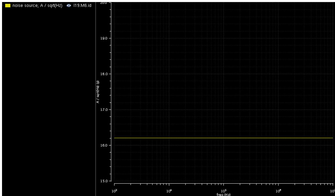
Action 6-31: In the Direct Plot Form, choose *Src. Noise Gain*. Set by *top* to 1. Click *Plot* to plot the noise gain from primary source in instance to output.
