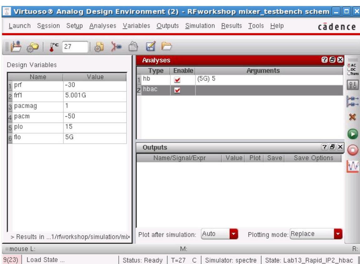
**Action 13-12:** In the Virtuoso Analog Design Environment window, choose **Simulation — Netlist and Run** or click the **Netlist and Run** icon to start the simulation.
