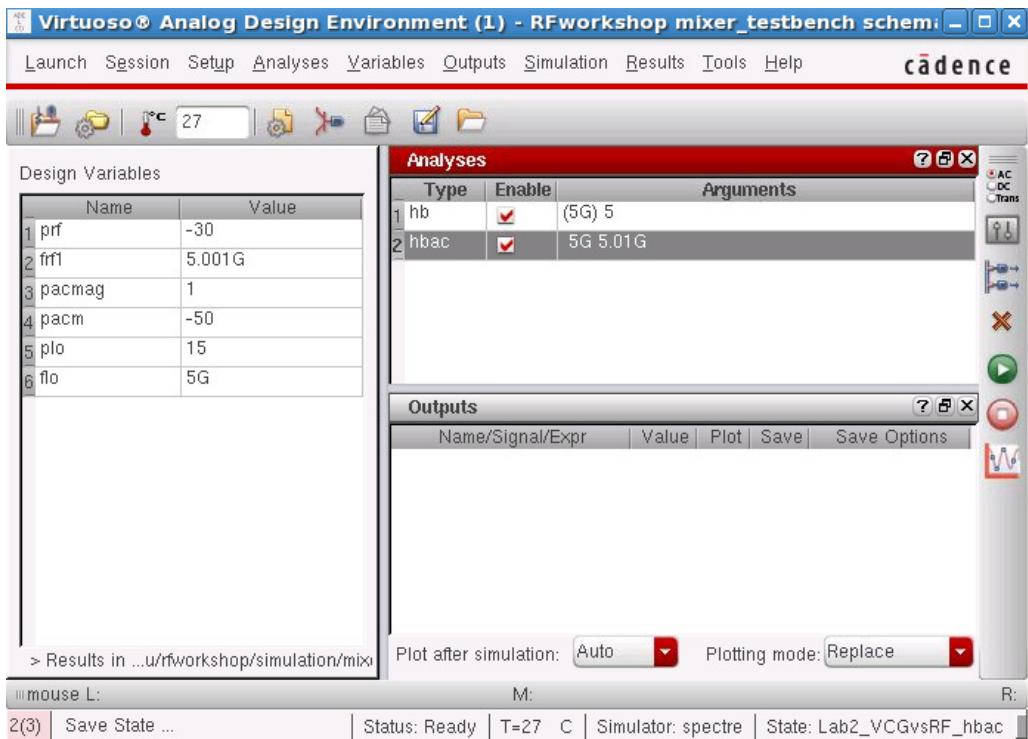
**Action 2-9:** In the Virtuoso Analog Design Environment window, choose **Simulation — Netlist and Run** or click the **Netlist and Run** icon to start the simulation.
