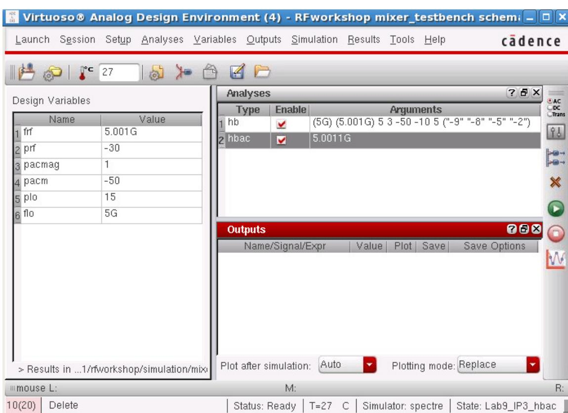
**Action 9-12:** In the Virtuoso Analog Design Environment window, choose **Simulation — Netlist and Run** or click the **Netlist and Run** icon to start the simulation.
