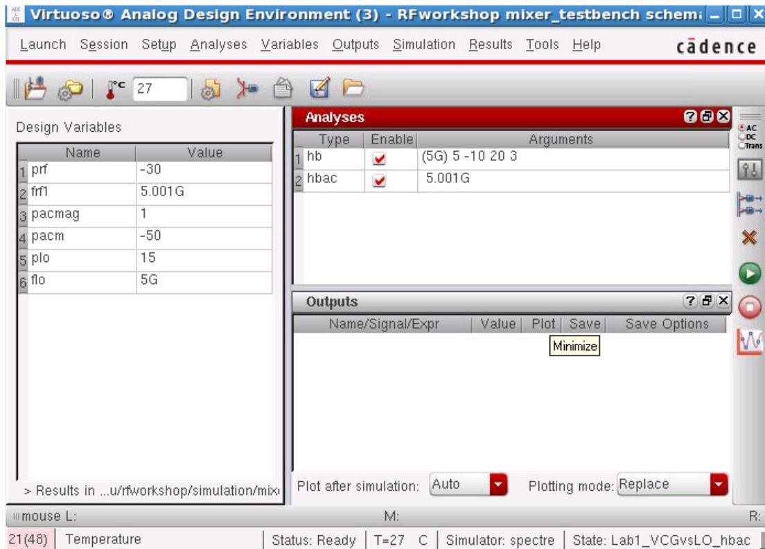
**Action 1-12:** In the Virtuoso Analog Design Environment window, choose **Simulation — Netlist and Run** or click the **Netlist and Run** icon to start the simulation.
