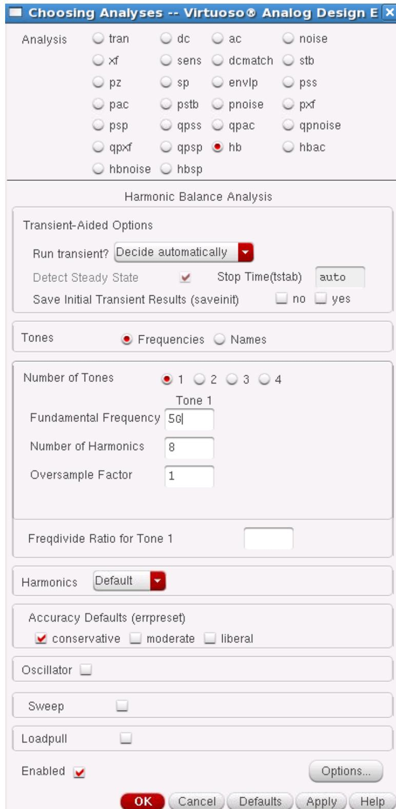
**Action 6-8:** In the Choosing Analyses window, select the *hbnoise* button in the *Analysis* field of the window and set up the form as follows:
