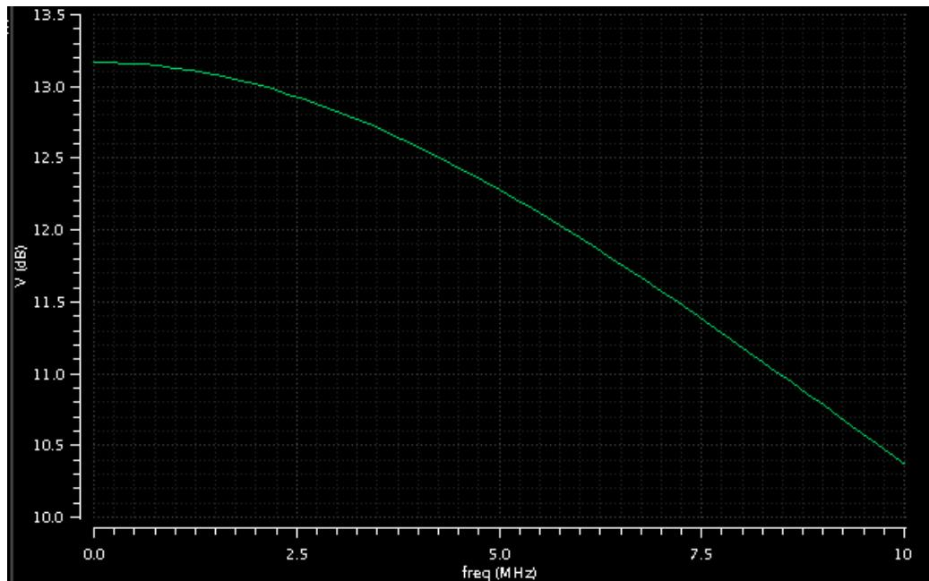
Because the sweep type in the analysis is linear by default, uniform frequency points display along the X-axis in the above plot. For a large frequency range, set the sweep type to logarithmic.
