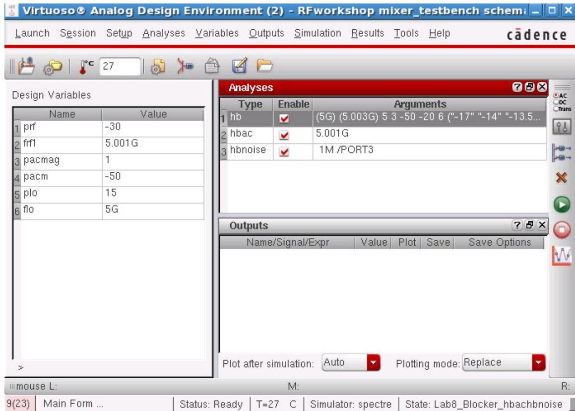
Action 8-14: In the Virtuoso Analog Design Environment, choose **Simulation — Netlist and Run** or click the **Netlist and Run** icon to start the simulation.
