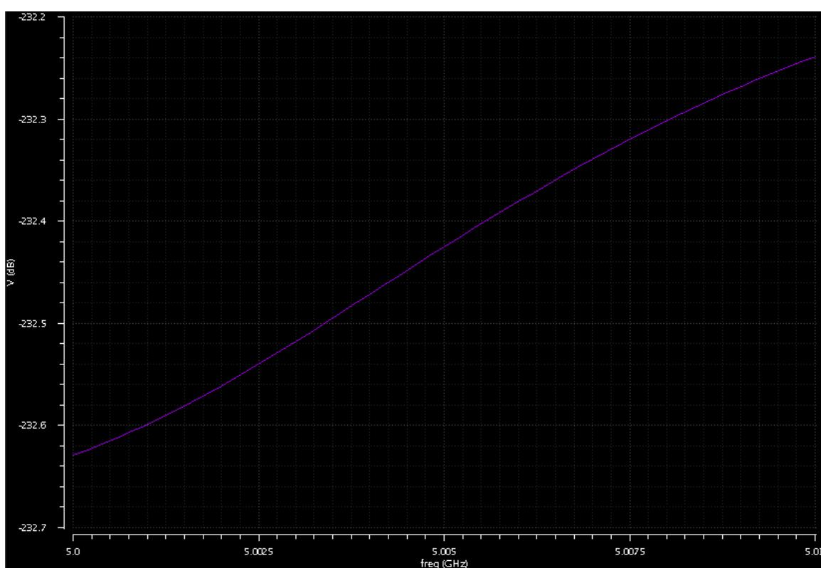
RF-to-IF feedthrough might create an even-order distortion problem for homodyne receivers. Measure RF-to-IF feedthrough using the *hbac* analysis results with two simple changes.
