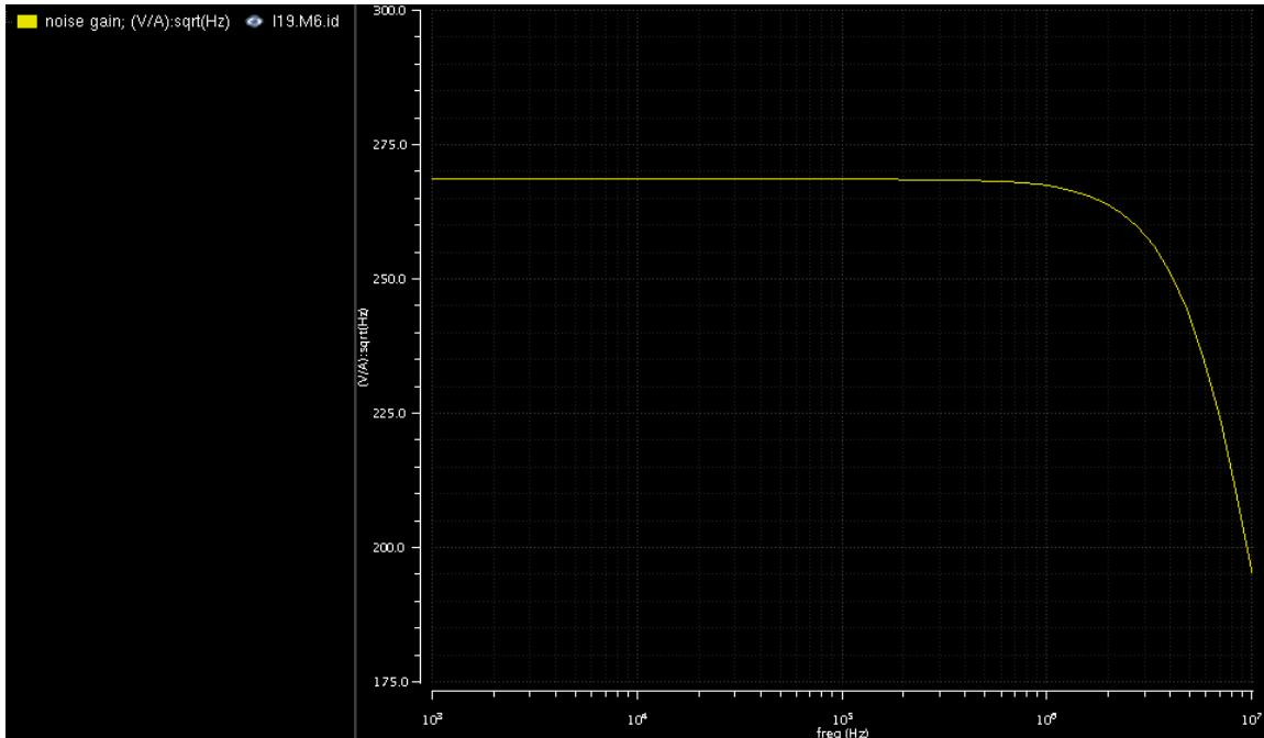
So to improve the noise performance of this circuit, decreasing the output noise of “I19.M6” is an effective solution. There are two approaches: one is decreasing the magnitude of noise source “I19.M6” by adjusting the device geometric size; the other is decreasing the transfer function of “I19.M6” by adjusting the circuit architecture.
