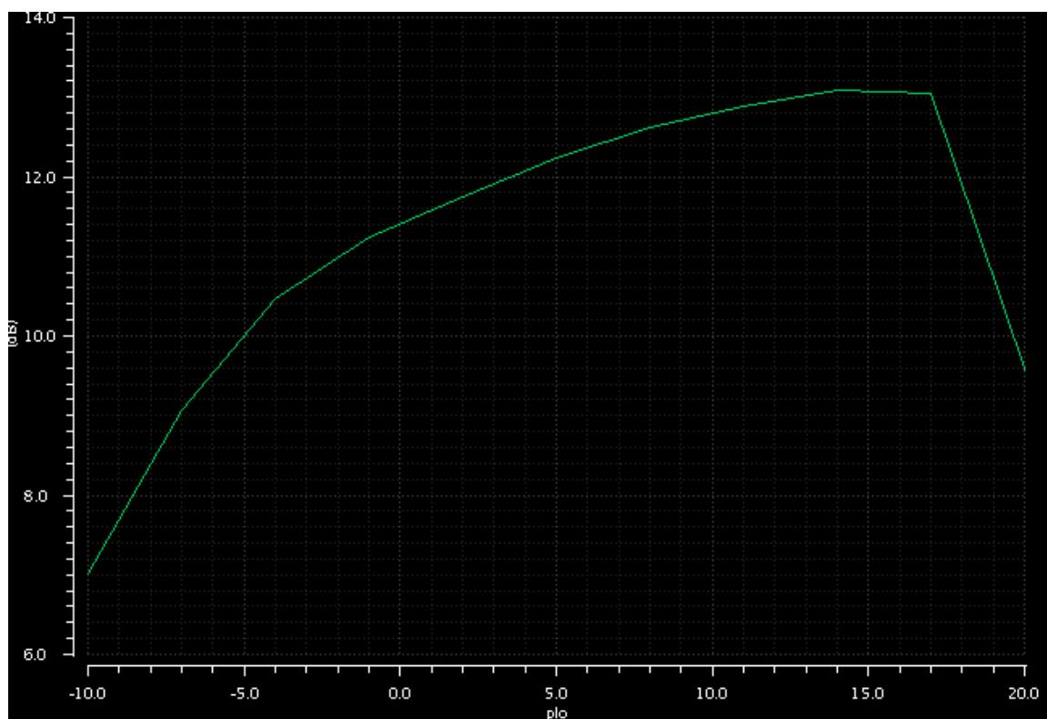
The PAC analysis computes gain directly only when you set the pacmag parameter to 1 V. Otherwise, take a ratio of the output and input. The maximum conversion gain value is reached somewhere around 15 dBm. Use this value for the plo parameter in the following measurements.
