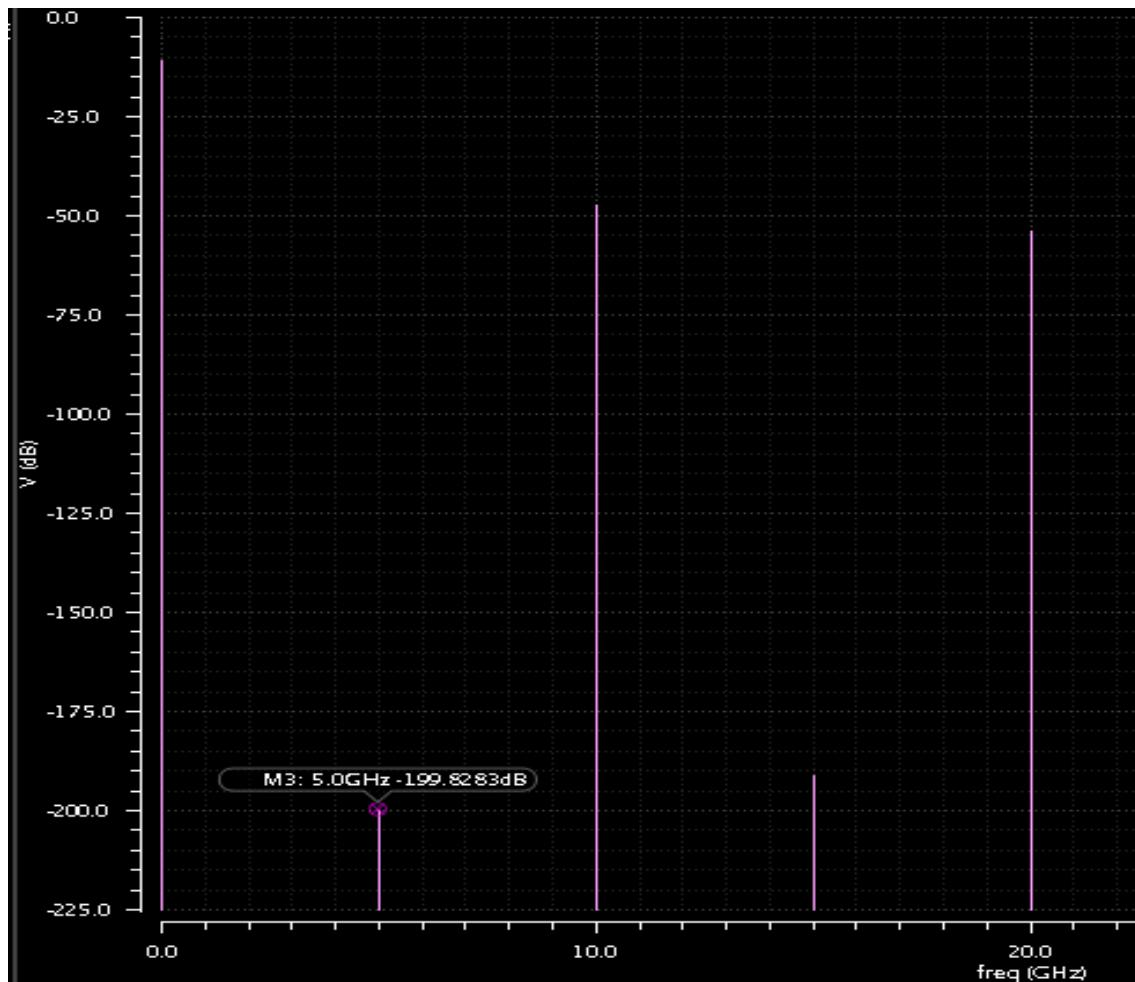
RF-to-LO feedthrough affects the local oscillator by letting strong interferers at the input pass through to the LO. Measure RF-to-LO feedthrough using the PAC analysis results.
