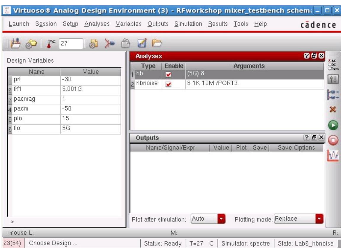
**Action 6-10:** In the Virtuoso Analog Design Environment window, choose **Simulation — Netlist and Run** or click the **Netlist and Run** icon to start the simulation.
