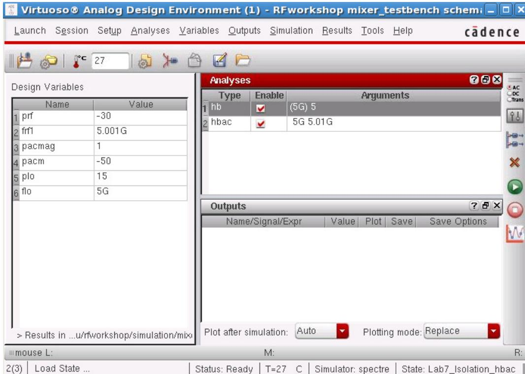
**Action 7-12:** In the Virtuoso Analog Design Environment, choose **Simulation — Netlist and Run** or click the **Netlist and Run** icon to start the simulation.
