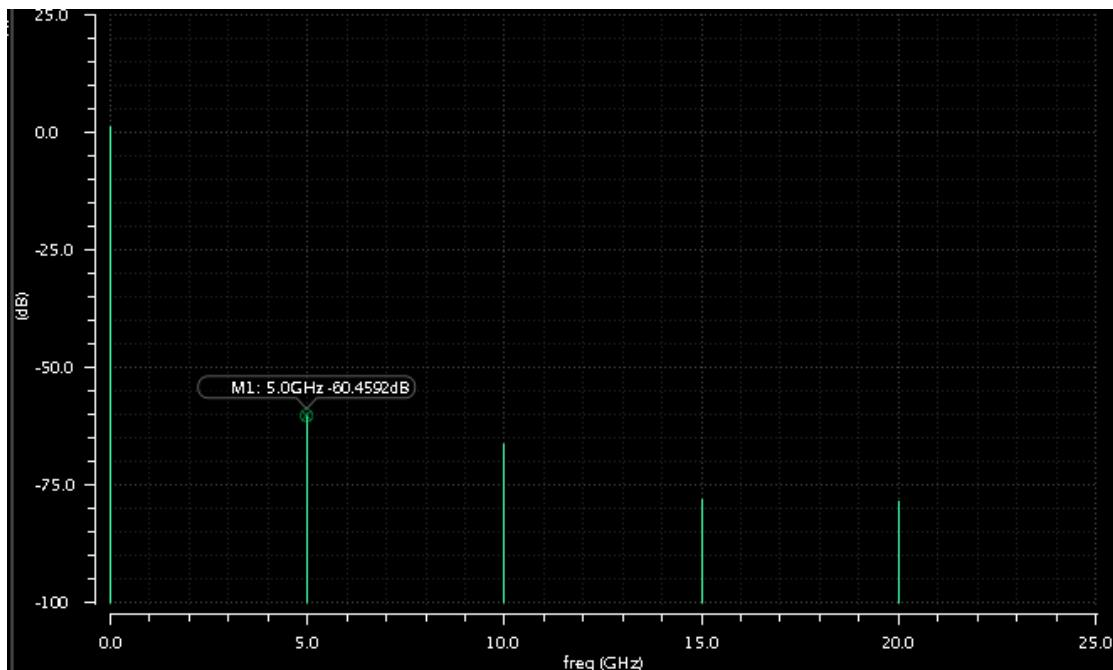
LO-to-RF feedthrough affects the functionality of LNAs and antennas and the self-mixing causes the dc offset. Use the results of the PSS analysis with the LO port as input and the RF port as output to measure the LO-to-RF feedthrough.
