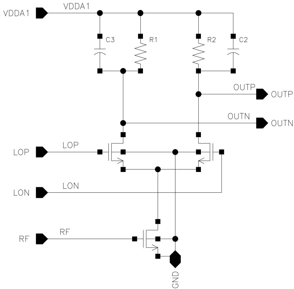
The example circuit, a single balanced differential down-converting mixer, runs with a local oscillator at  $f(LO) = 5$  GHz. The range of interest is the baseband output noise from 1 kHz to 10 MHz. The RF signal frequency used for the simulation is around 5001 MHz.
