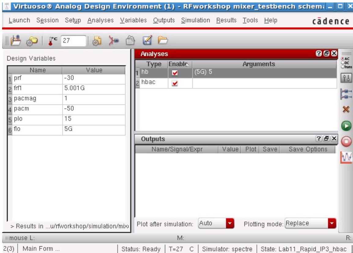
**Action 11-11:** In the Virtuoso Analog Design Environment window, choose **Simulation — Netlist and Run** or click the **Netlist and Run** icon to start the simulation.
