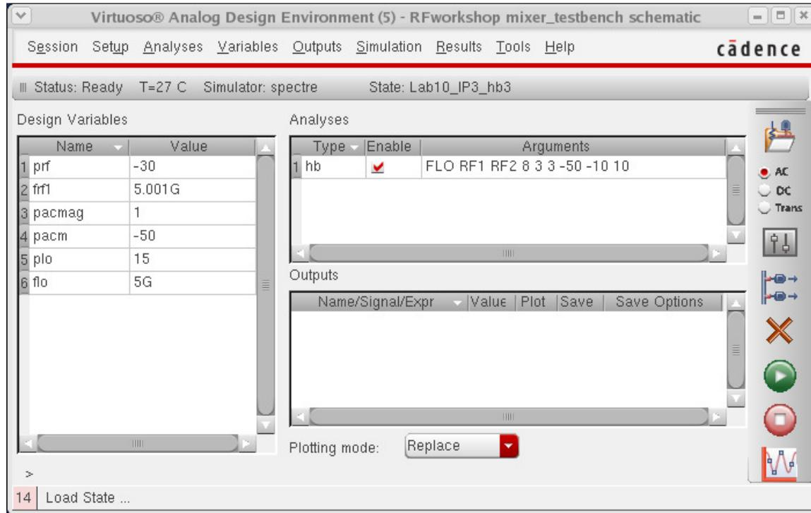
**Action 10-10:** In the Virtuoso Analog Design Environment window, choose **Simulation — Netlist and Run** or click the **Netlist and Run** icon to start the simulation.
