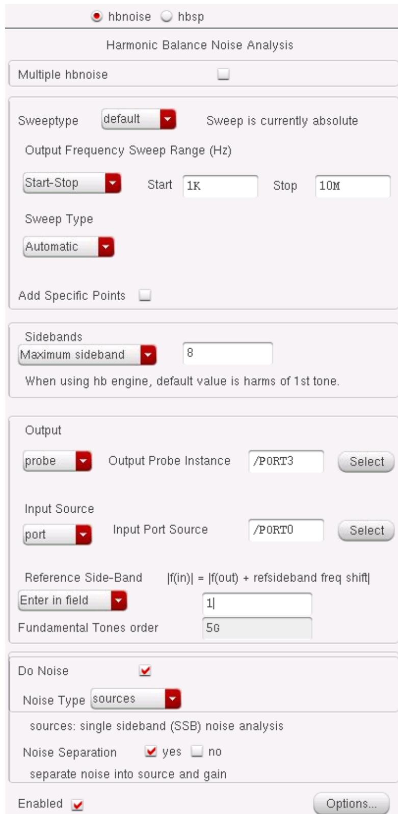
**Note:** You must specify the load as an output or probe. The load can be a resistor or a port. All noise from the source is included in the denominator
