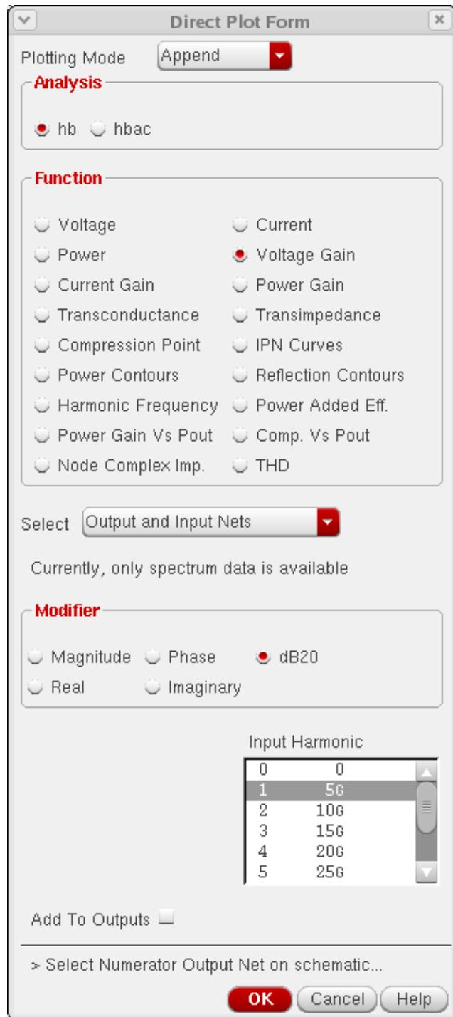
**Action 7-15:** In the schematic, select the net IFp as the output and net VLO as input.
