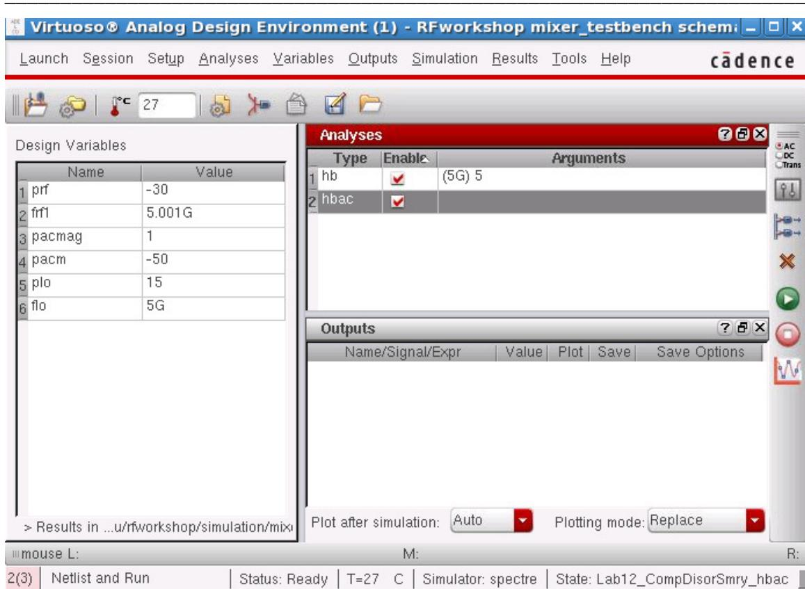
**Action 12-11:** In the Virtuoso Analog Design Environment, choose **Simulation — Netlist and Run** or click the **Netlist and Run** icon to start the simulation.
