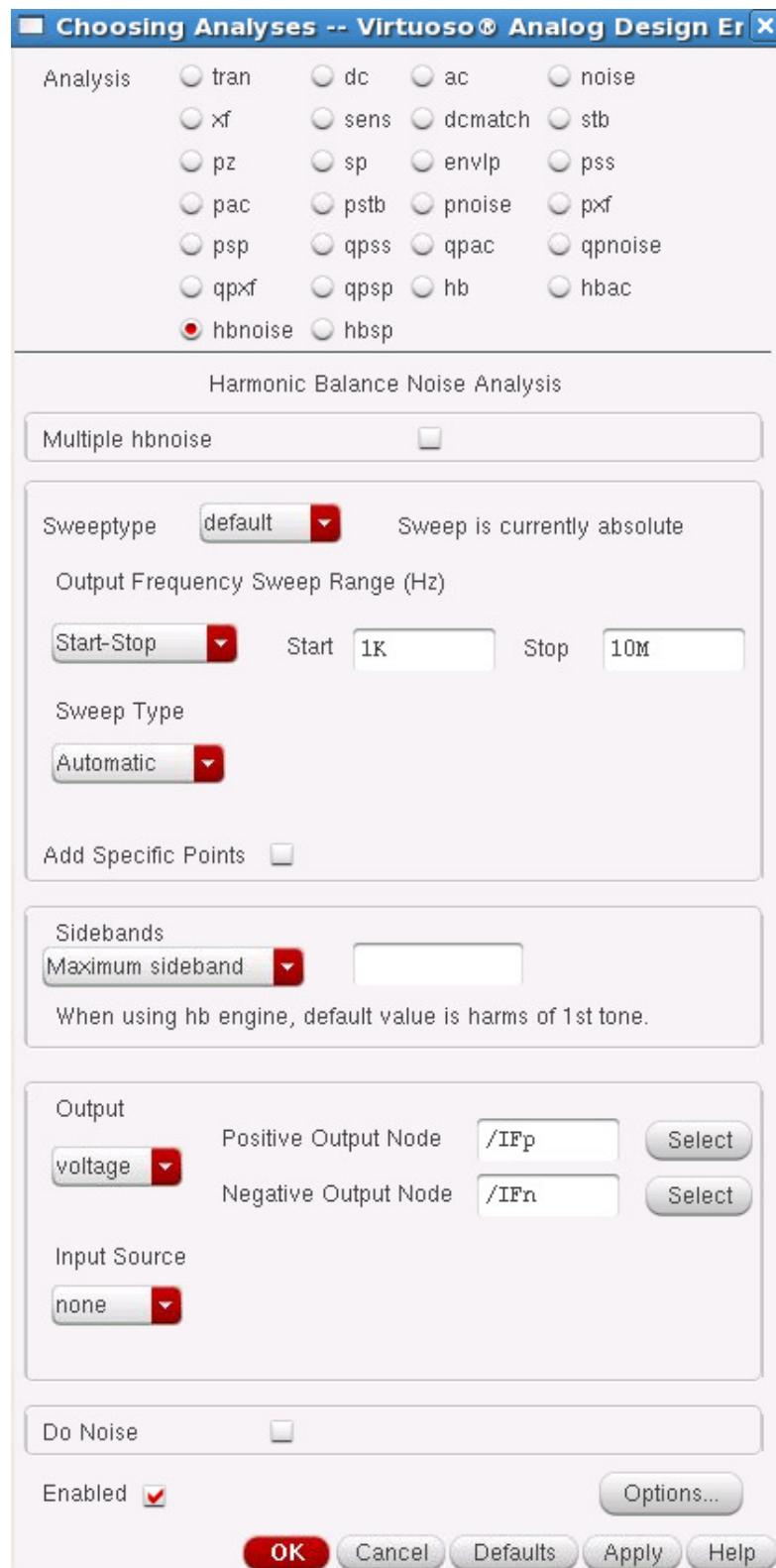
Note: When turning off the *Do Noise* button, the hbnoise analysis is actually the hbxf analysis.
