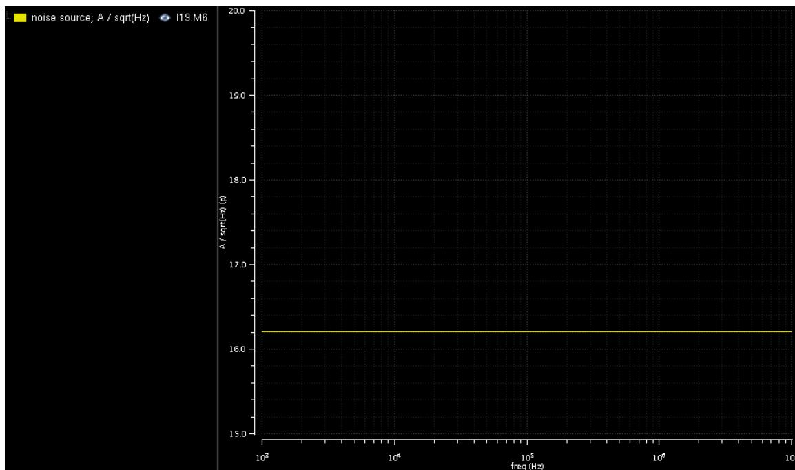
Action 6-30: In the Direct Plot Form, choose *Primary Source*. Set by *top* to 1. Click *Plot* to plot the noise source measurement of primary source in instance "I19.M6".
