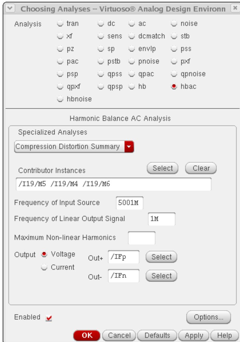
In the above form, the Maximum Non-linear Harmonics is not specified, so the default value 4 is used.
