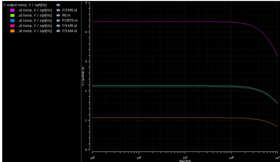
This plot shows that the thermal noise from the channel of I19.M6 is the largest noise contributor, followed by the thermal noise of the resistor R6. Note that the list order of the instances in this plot is different from that of **instance output**.
