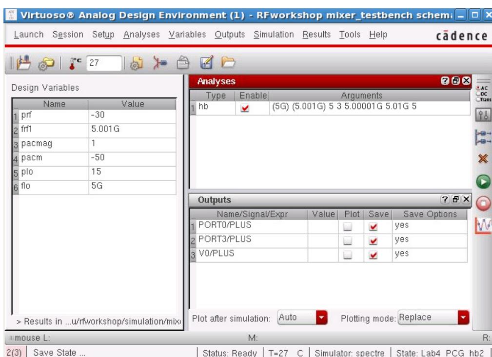
**Action 4-12:** In the Virtuoso Analog Design Environment window, choose **Simulation — Netlist and Run** or click the **Netlist and Run** icon to start the simulation.
