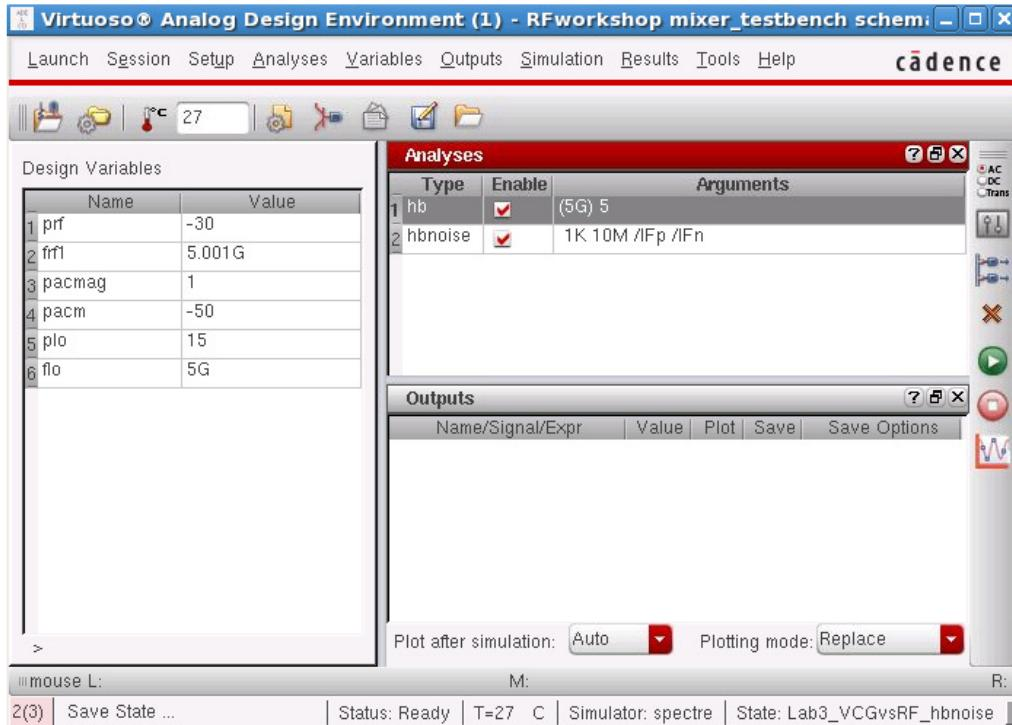
**Action 3-9:** In the Virtuoso Analog Design Environment window, choose **Simulation — Netlist and Run** or click the **Netlist and Run** icon to start the simulation.
