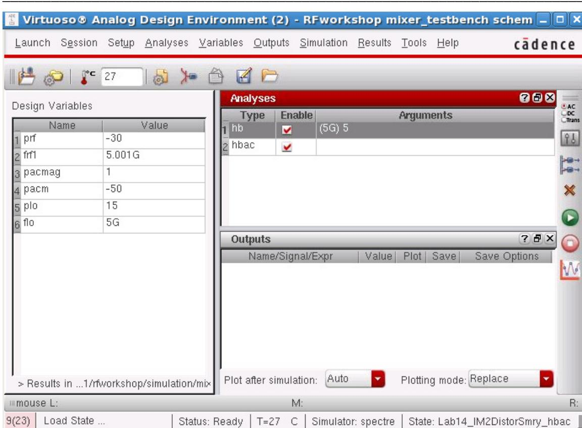
**Action 14-10:** In the Virtuoso Analog Design Environment window, choose **Simulation — Netlist and Run** or click the **Netlist and Run** icon to start the simulation.
