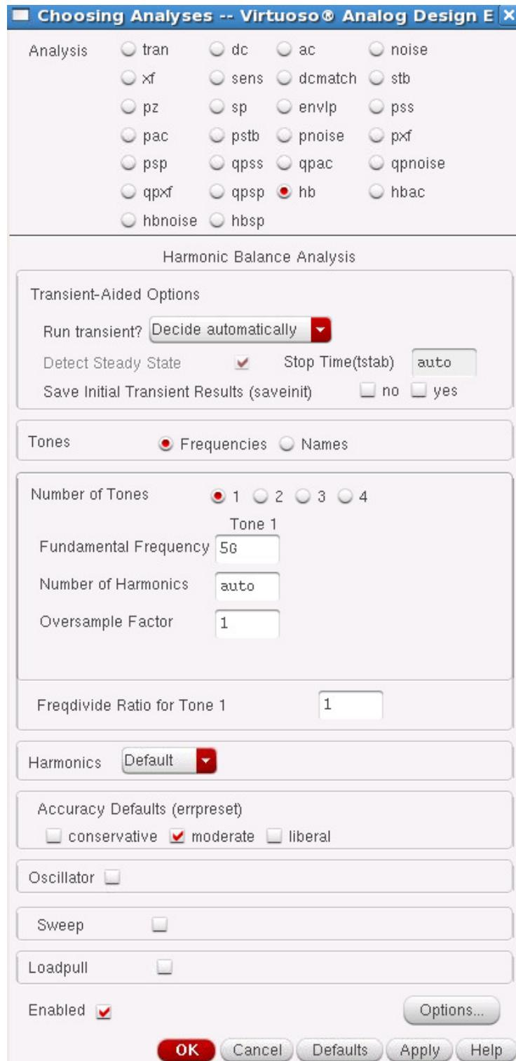
**Action 5-9:** In the Choosing Analyses window, select the *hbsp* button in the *Analysis* field of the window and set the form as follows:
