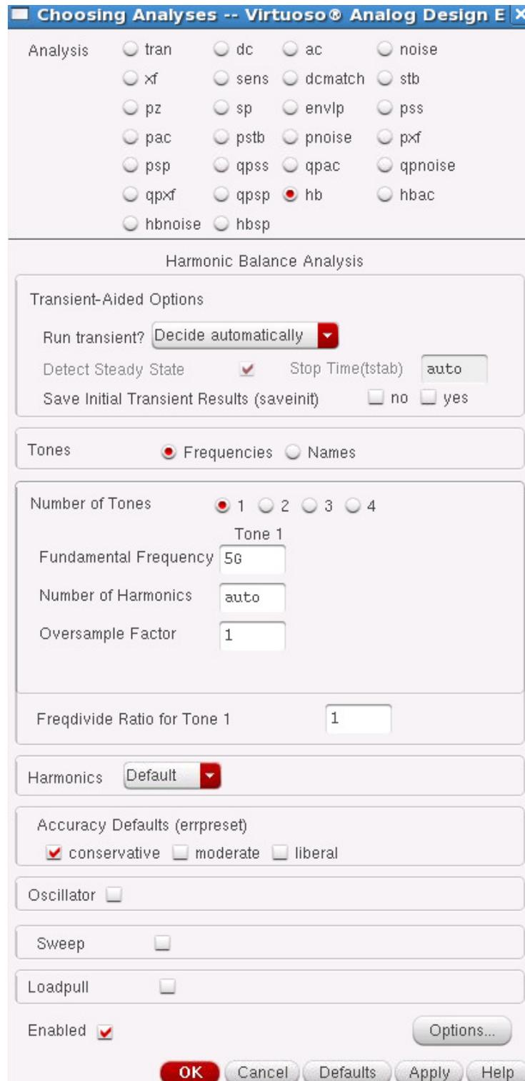
hb simulation is set up here to check the LO feedthrough. LO feedthrough is a large-signal effect and should not be measured using a small-signal
