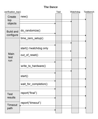
The first thing that <code>verification\_top()</code> does is build the global logging objects. These provide for logging, as well as for shutting down the simulation after a threshold number of errors have been logged. (See <code>truss\_vout.svh</code> in the index.)
