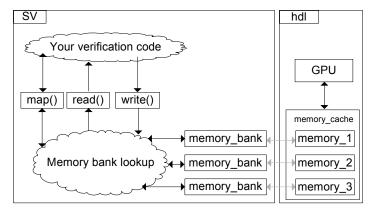
To support direct memory access you need to do a few things. First, you need to create an interface to the memory register bank. Then you need to define a subclass of teal::memory\_bank that takes in a virtual interface of that type and performs the from\_memory() and to memory() functions. After that, you need to create an instance of
