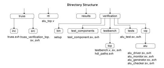
The source code for the chip is in the /rtl directory. How does the truss run script know this? The file /verification/testbench/top/hdl\_paths.vc is used to specify the paths to the RTL and the RTL include directories and all source files. This is so that the RTL files can be rooted in a place different from the verification directory.
