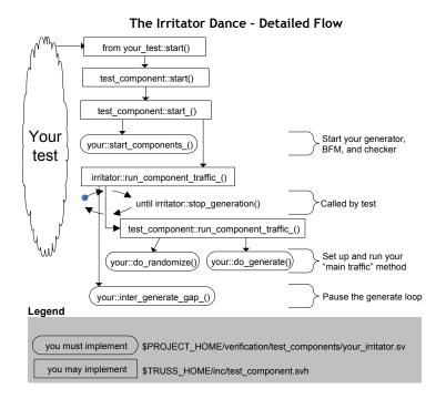
The irritator overrides the run\_component\_traffic\_() method from the test\_component base, and calls the base class run\_component\_traffic\_() method in a loop. This is the nature of an irritator: it just keeps on going until told to stop. The method that stops the loop is stop\_generation(), which is usually called by your test once the main feature or protocol has finished being tested. This will be shown in detail in the Part IV of this handbook.
