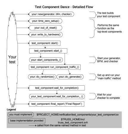
The run\_component\_traffic\_() method has a standard implementation, which calls do\_randomize() and then do\_generate(). The do\_randomize() method has the same purpose it had for the top-level components: to randomize your random variables. The next method called, do\_generate(), picks up the results of the randomization and interacts with the generator to exercise a feature or a protocol of the chip.
