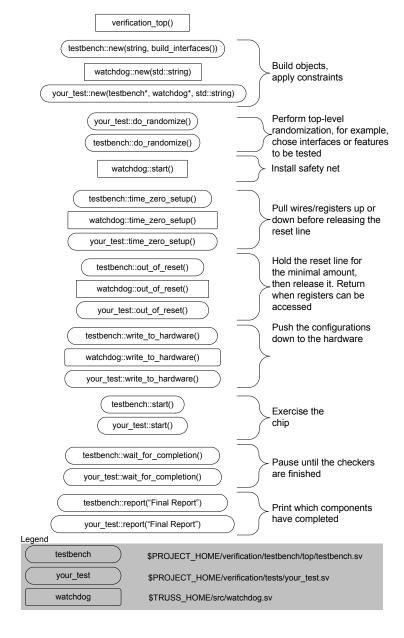
The watchdog class is already written and should be sufficient for most purposes. (We will not discuss the watchdog timer's methods, because they are relatively straightforward.) You'll have to write the test and testbench classes.
