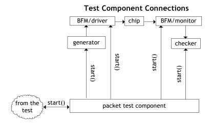
The packet test component class gets a pointer to both BFMs, a generator, and a checker. The role of the packet test component is to exercise some part of the chip by using these other components.
