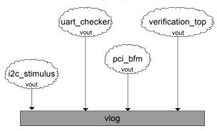
Note that vout simply takes a string. By calling the appropriate function—info(), error(), fatal(), debug()—vout can provide this information to the vlog class. This information is not just sent as a string, but is passed as metadata that can be useful for further processing. This is described more fully below.
