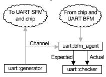
The checker\_agent provides the checker with three things: the expected, the actual, and whether or not there is more checking to do.
