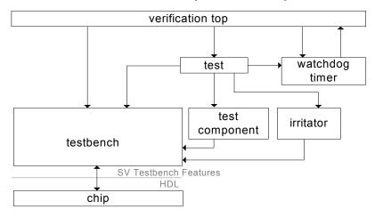
The top-most component is the verification\_top() program, whose role is to create and sequence the other components through a standard
