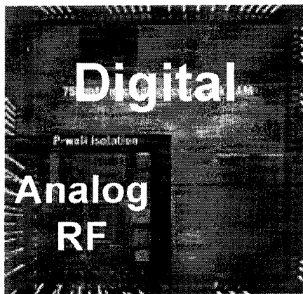
Figure 1.1 Ericsson single-chip 0.18- \mu\text{m} CMOS Bluetooth radio (2001).
