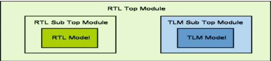
Figure 5-15. Single Top Module as Test Bench Platform
