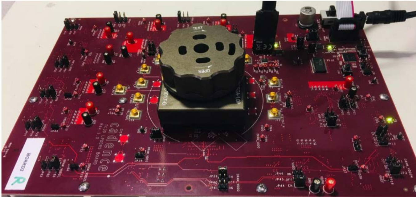
TC30 LPDDR5 test board with Test Chip and Memory soldered down
