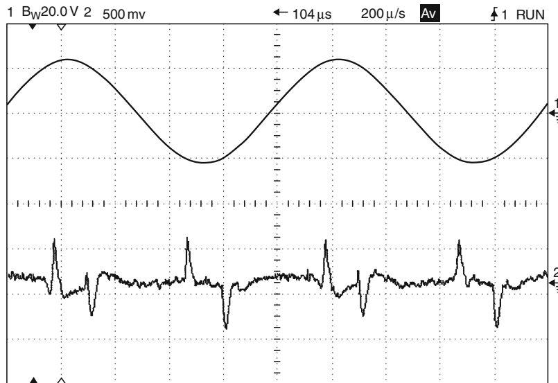
Figure 19.20. The THD residua waveform of the Class-A + C amplifier above transition, at 30 W into 8 \Omega . Switching artefacts are visible but not crossover distortion.
