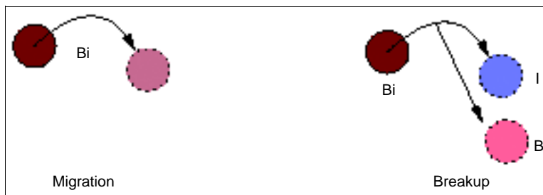
Figure 45 Impurity pairs can diffuse or break up into a substitutional plus an interstitial or a vacancy
