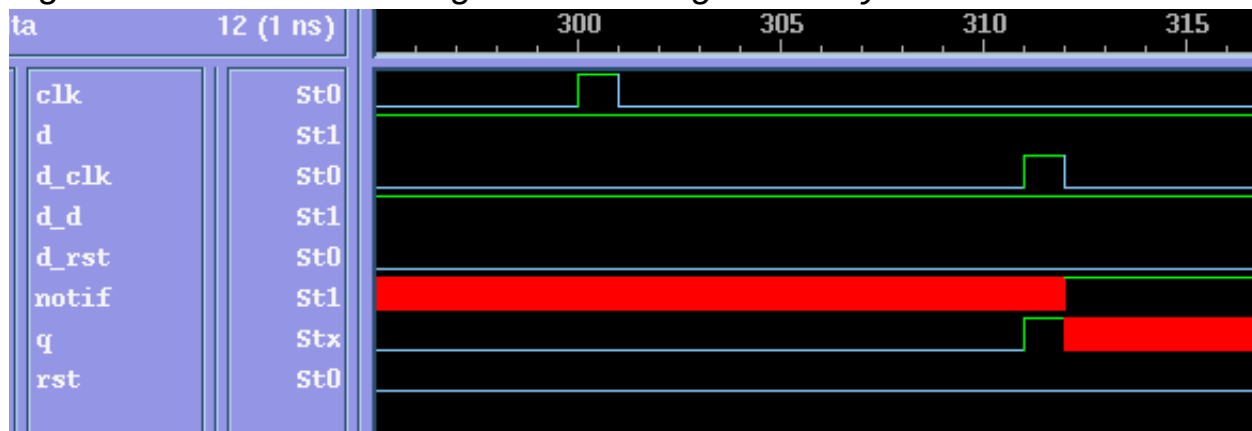
Figure 12-15 Other Timing Checks Using the Delayed Versions
