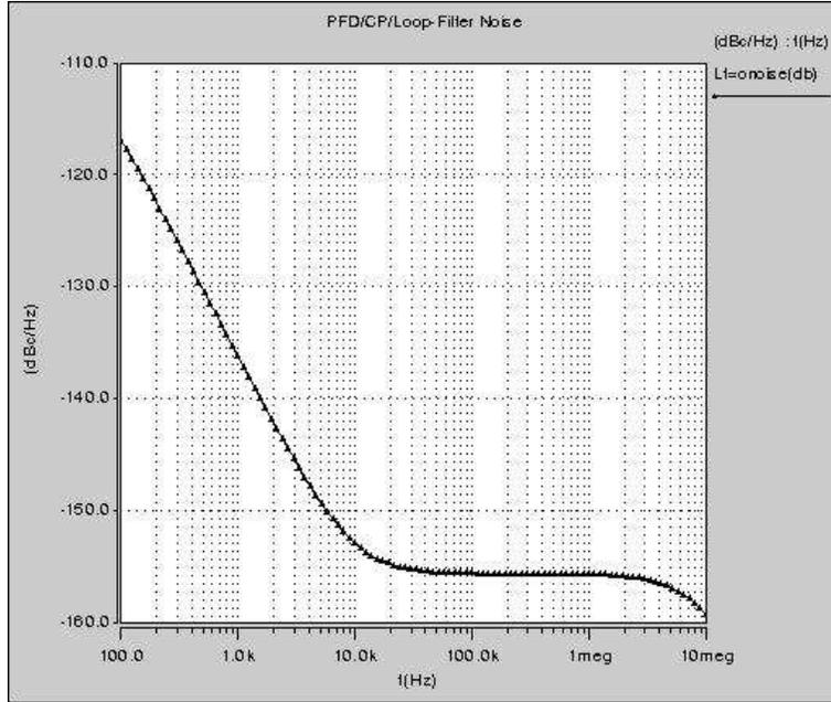
Figure 15. Simulation results from the .SNNOISE cyclostationary noise analysis for the PFD/CP/Loop-filter combination based on a Shooting Newton analysis. The onnoise measurement is taken at the loop filter output – one of the few places where the voltage domain and phase domain measurements are equivalent. When viewed in terms of noise power, it is equivalent to a phase noise response.
