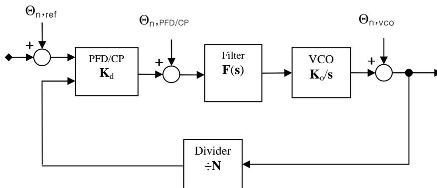
Figure 19. The locked-state phase-domain model of the PLL used for closed-loop noise analysis. The three noise sources ( $\Theta_n$ ) represent noise contributions from the reference oscillator, VCO, and the combined PFD, charge-pump, and loop filter (shown as the PFD/CP noise source). Note that the PFD/CP noise has been relocated at the input of the loop filter.
