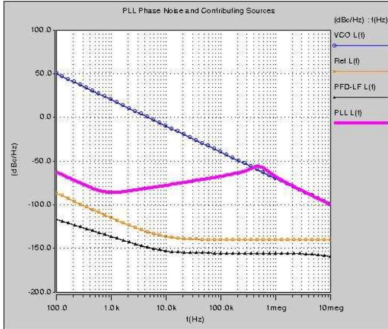
Figure 21. Noise analysis results for the phase-domain PLL. The closed-loop PLL phase noise is shown with the contributing sources. The HSPICE RF analysis performs the noise shaping calculations by computing the closed-loop response functions for how each noise source contributes to the output.
