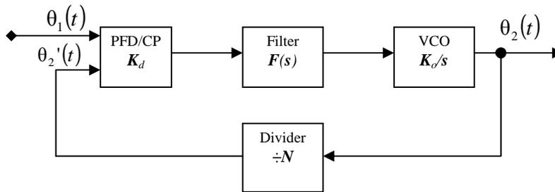
Figure 2. Block-diagram of the PLL locked-state phase-domain model.
