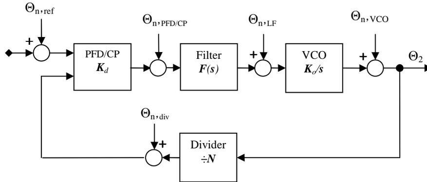
Figure 4. Noise analysis model for the locked-state phase-domain PLL. Noise source contributions ( $\Theta_n$ ) may originate from the reference oscillator, the VCO, the combined PFD/charge-pump, the loop filter, and the divider. In the phase-domain model, injected noise corresponds to *phase noise* contributed by the PLL components.
