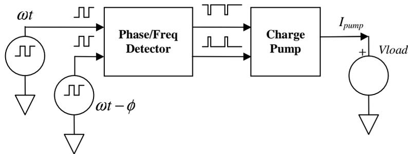
Figure 6. Simulation setup to extract the output charge pump current as a function of the phase difference at the phase/frequency detector input. Voltage source  $V_{load}$  establishes the output voltage bias and is used to measure current flow. The steady-state input sources are setup to differ in phase.
