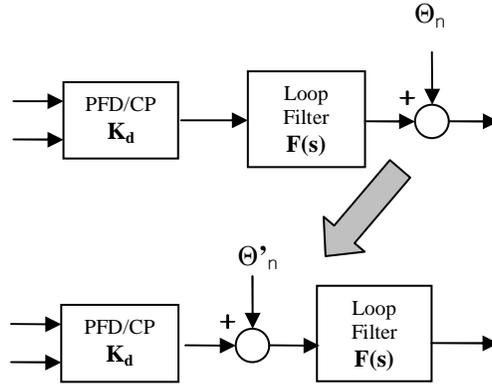
Figure 16. The noise contributions from the PFD, charge-pump, and loop-filter are best modeled by using a behavioral noise source located between the charge-pump and loop filter. This allows the noise model to have a relatively simple frequency characteristic.
