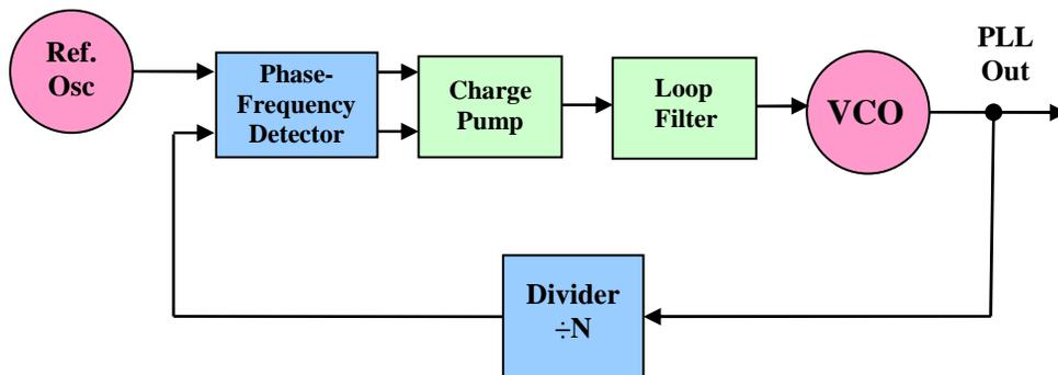
Figure 1. Prototypical PLL including VCO, PFD/CP, loop filter, divider, and reference oscillator.
