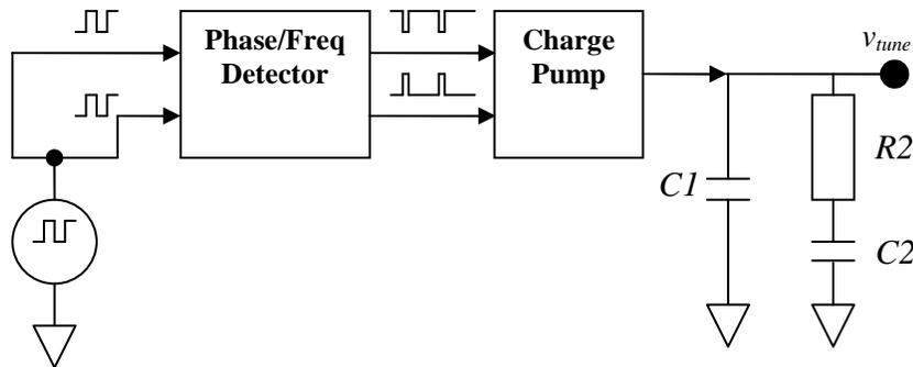
Figure 13. To extract the noise contributions from the PFD, charge-pump, and loop filter, a steady-state analysis is run with the PFD driven with in-phase signals. A cyclostationary noise analysis, using `.SNNOISE`, can then be used to extract the frequency dependent “*onoise*” at the loop filter output.
