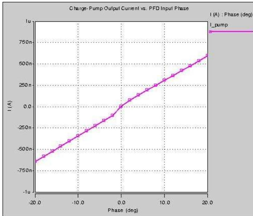
Figure 8. Results of an HSPICE RF *Shooting Newton* analysis showing the steady-state charge-pump current (DC component) as a function of input phase difference. The slope of the curve yields the PFD/CP gain  $K_d$  which here is approximately 30 nA/deg. This analysis is easily extended to include parameter sweeping over bias and Vdd levels.
