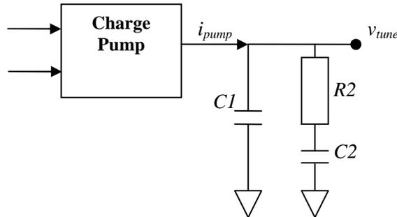
Figure 9. An example passive 2<sup>nd</sup> order loop filter. The Laplace transfer function for this loop component has the form:
