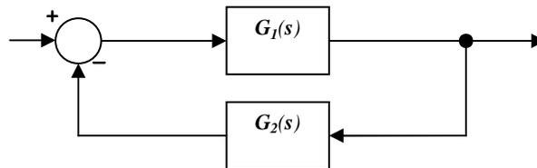
Figure 3. Convention used for frequency-domain (Laplace) forward gain and feedback transfer function calculations.
