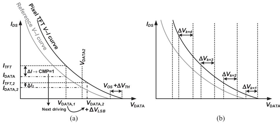
Fig. 4. (a) Reduction of TFT current error ( $\Delta I$ ) under hybrid driving. (b) Gray-level grouping for mobility compensation.
