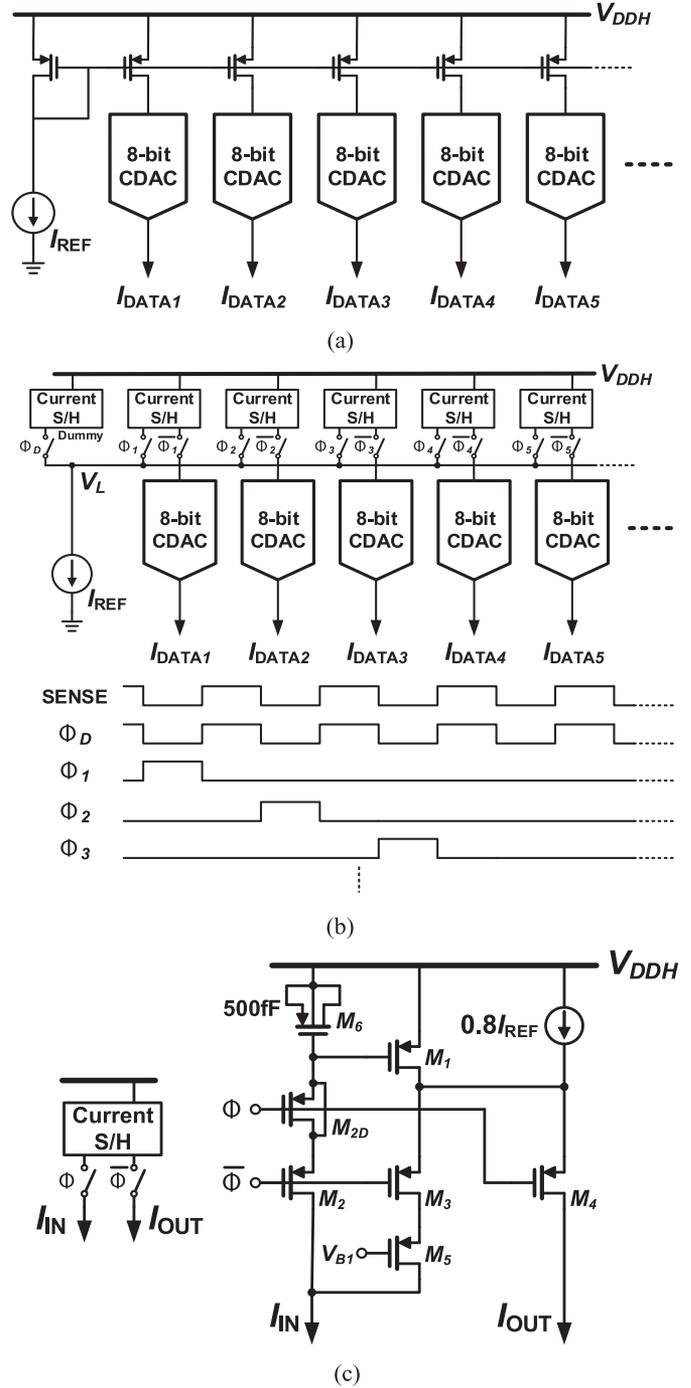
Fig. 9. (a) Conventional channel reference current distribution method. (b) Reference current calibration (RCC). (c) Current sample and hold (S/H).
