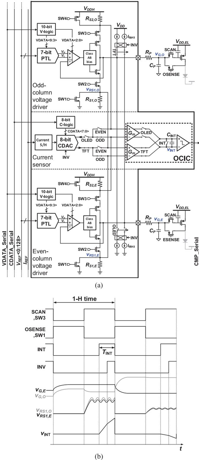
Fig. 8. (a) Entire block diagram and (b) timing diagram of the hybrid column-driver operation for odd-column TFT current-sensing (ODD = H, EVEN = L, TFT = H, OLED = L).
