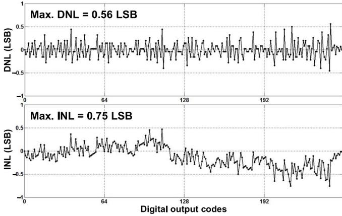
Fig. 16. DNL and INL of the 8 bit circuit-reused current-mode SAR ADC.
