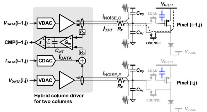
Fig. 7. Simplified block diagram of hybrid column-driver for differential sensing method.
