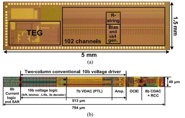
Fig. 14. (a) Chip micrograph of prototype IC and (b) layout of the hybrid column-driver for two columns.
