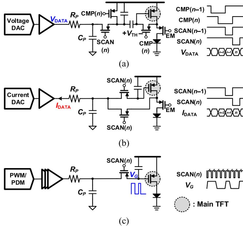
Fig. 2. AMOLED driving methods. (a) Voltage driving with in-pixel threshold voltage ( $V_{TH}$ ) compensation. (b) Current driving. (c) Digital driving.
