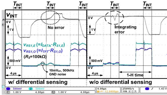
Fig. 17. Measured waveform of the hybrid-driving under emulated panel noise of 10 mV<sub>pp</sub> at 500 kHz with/without the differential sensing method when sensing the odd-column TFT current.
