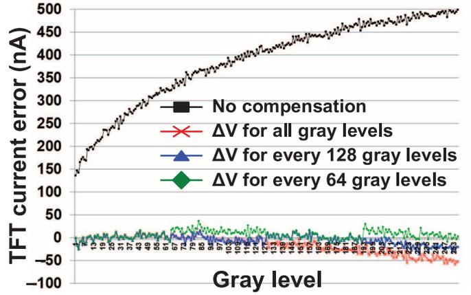
Fig. 18. Current error between two emulated TFTs with threshold voltage ( $V_{TH}$ ) difference of 60 mV before and after compensation.
