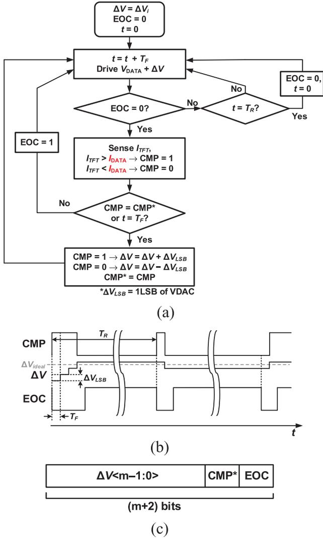
Fig. 5. Algorithm of real-time TFT current nonuniformity compensation. (a) Flowchart. (b) Timing operation example. (c) Memory cell for one gray-level group of one pixel.
