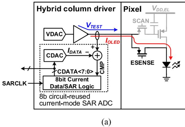
Fig. 13. (a) 8 bit circuit-reused current-mode SAR ADC and (b) its current data/SAR logic connection in data logic mode and ADC mode.
