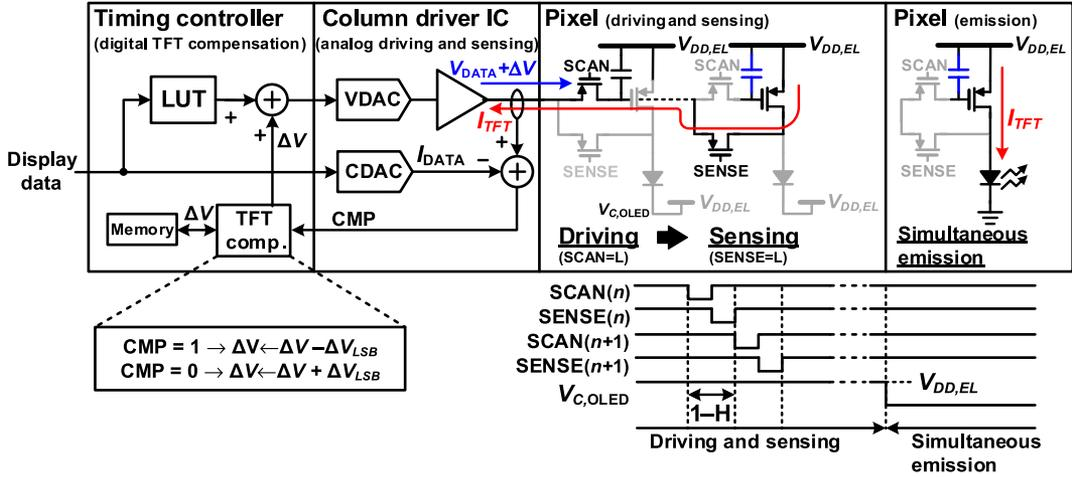
Fig. 3. Functional diagram of proposed hybrid-driving method.
