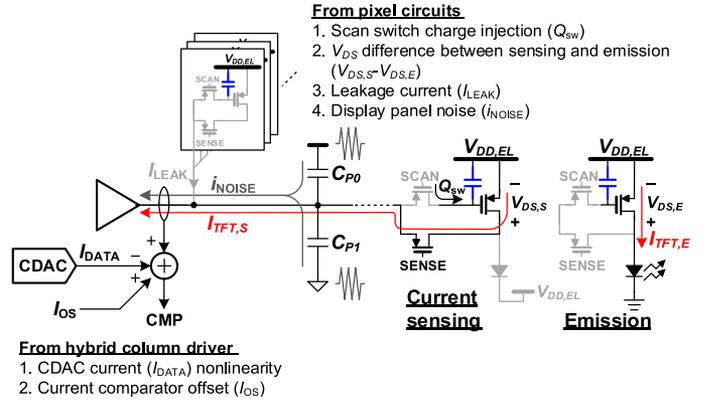
Fig. 6. Main error sources in current-sensing of hybrid-driving method.
