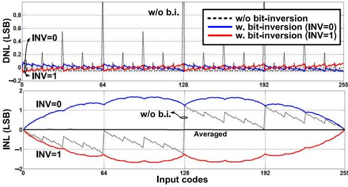
Fig. 11. DNL and INL of BICCDAC from a behavior simulation with a 1% intentional mismatch in the current divider.
