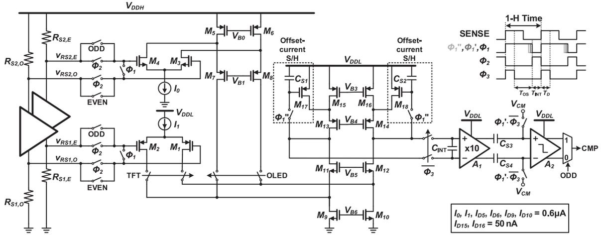
Fig. 12. Offset-compensated integrating comparator.
