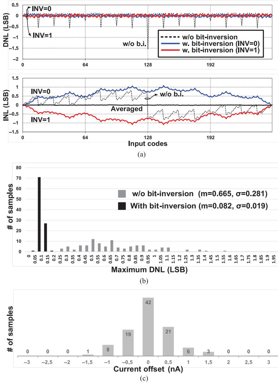
Fig. 15. Monte-Carlo simulation results from 100 samples. (a) Worst DNL and INL of the BICCDAC. (b) Histogram of the maximum DNL and INL of the BICCDAC. (c) Histogram of input-current-referred offset in the OCIC with 100 k $\Omega$  of the current-sensing resistor ( $R_S$ ).
