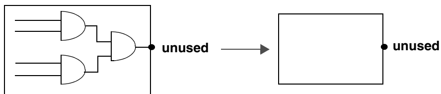
Figure 7-4 Minimizing Logic Driving an Unconnected Output Port
