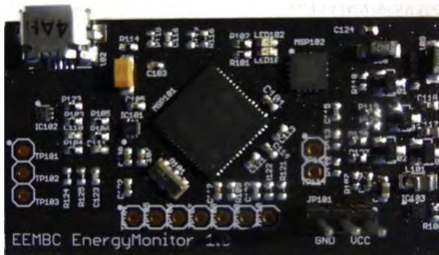
Figure 19.6 EEMBC Energy Monitor.
