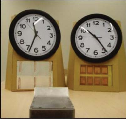
Figure 15.19 Wireless RF-powered wall clocks. Left: clock powered by an array of folded-dipole rectennas. Right: clock powered by an array of microstrip patch rectennas.
