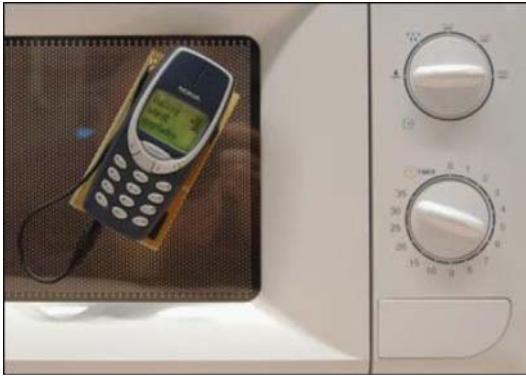
Figure 15.21 Mobile phone, powered by the 2.45-GHz signals leaking through the filter in the door of a microwave oven. The harvesting system consists of two microstrip patch antenna-based rectennas.
