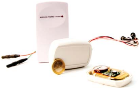
Figure 15.22 Wireless RF battery consisting of a microstrip patch antenna, conjugately matched to a voltage-doubling rectifier that is connected to a discrete, inductive boost converter, charging a 3-V Li-ion battery.
