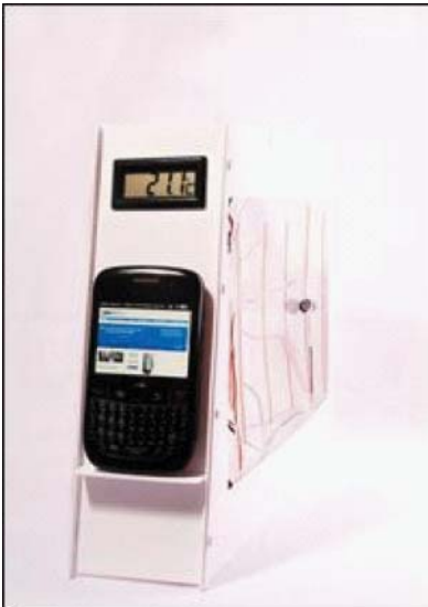
Figure 15.20 Smartphone-operated temperature sensor and display. Through a QR-code the smartphone is connecting to the Internet, thus transmitting power – either in the GSM or Wi-Fi frequency bands – that is partly intercepted by the dual-frequency rectenna.
