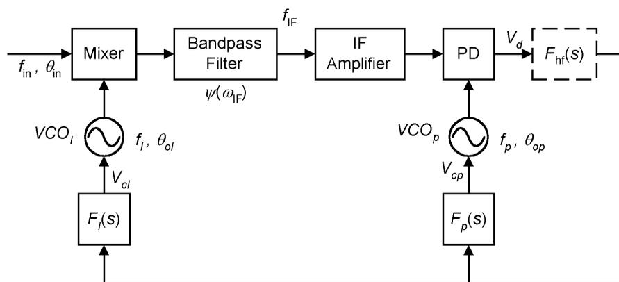
Figure 14.11 Block diagram of a split-loop PLL.
