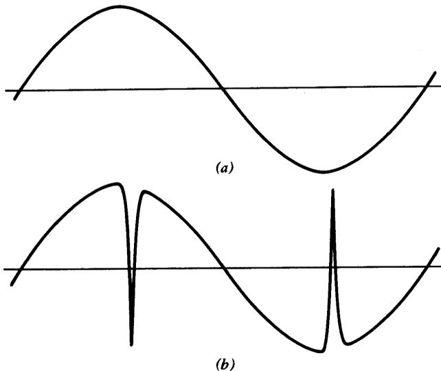
**Figure 5.18** Waveforms at the phase detector output of a first-order PLL subjected to sinusoidal angle modulation: (a) modulation peak deviation within the lock limits; (b) modulation peak deviation slightly beyond the lock limits.
