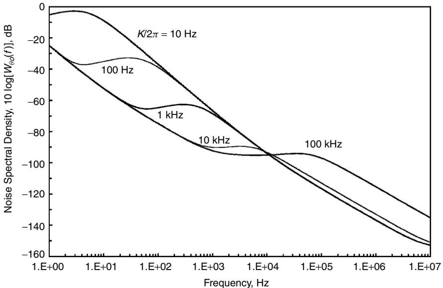
**Figure 15.10** Phase-noise spectra for various loop gains  $K$  in a PLL synthesizer ( $\zeta = 1$ ; same oscillators as in Fig. 15.9).
