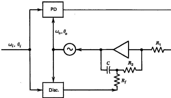
Figure 8.12 Discriminator-aided frequency acquisition in a type 2 PLL.
