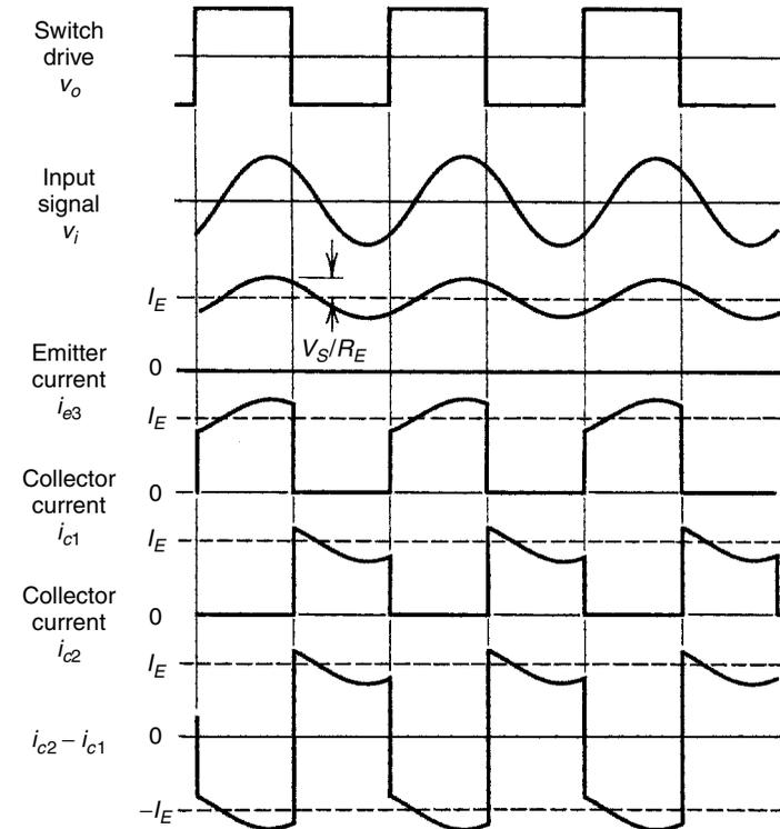
**Figure 10.3** Waveforms in an active single-balanced-modulator phase detector.
