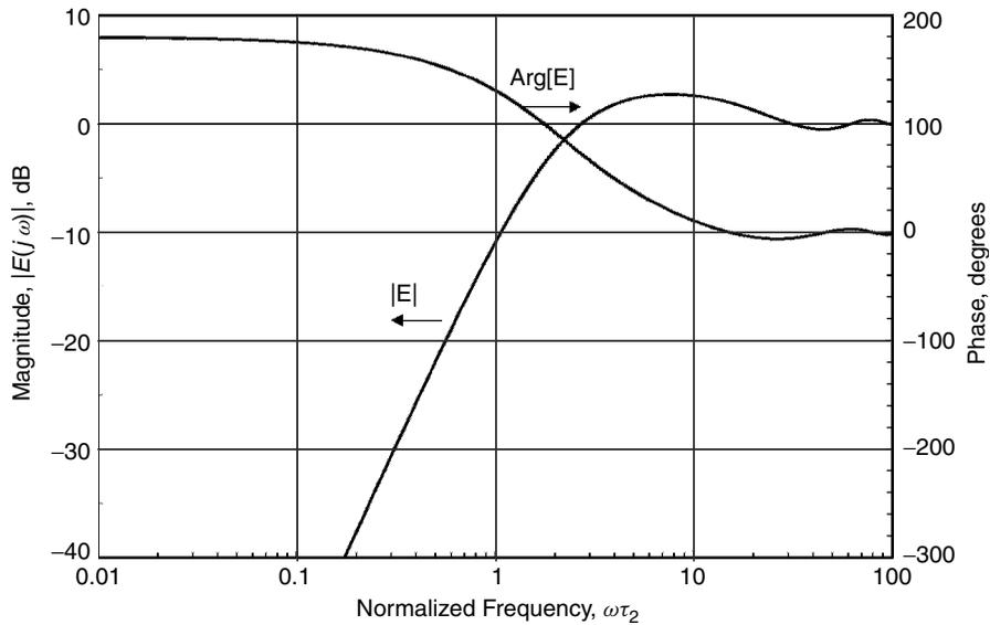
**Figure 3C.3** Frequency response of  $E(j\omega)$  for a type 2 PLL with  $K\tau_2 = 3$  and an in-loop delay of  $\tau_d = \tau_2/10$ ; the same parameters as for the Bode plot of Fig. 3.16 and the Nichols chart of Fig. 3.20.
