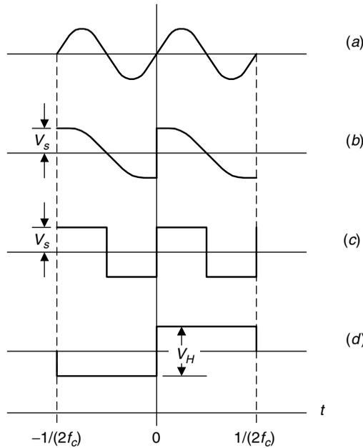
**Figure 10A.1** Ripple waveforms in example phase detectors.
