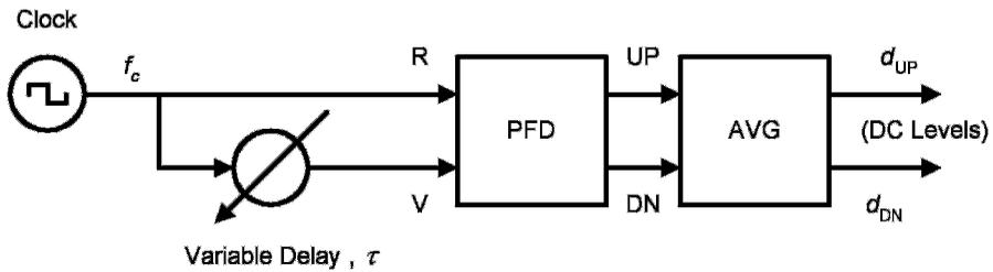
Figure 10.12 Hypothetical test setup to determine the  $s$ -curve of a PFD.
