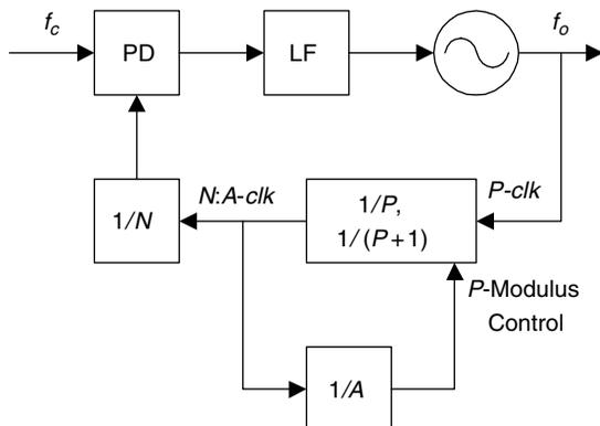
**Figure 15.4** Synthesizer with a dual-modulus divider.
