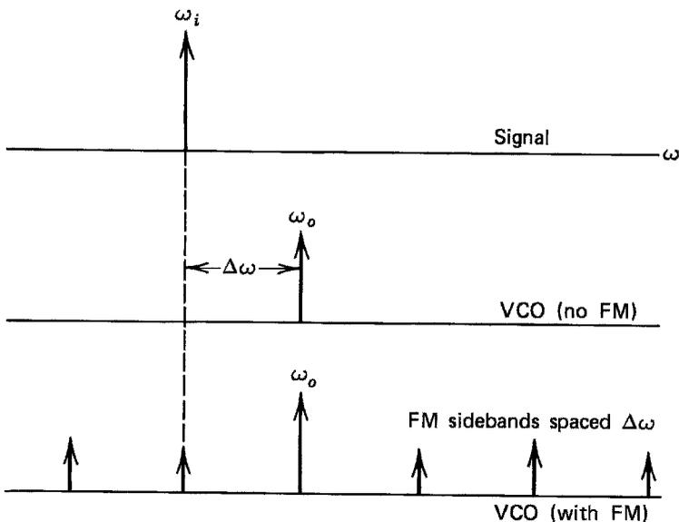
Figure 8.6 Signal and VCO spectra, illustrating pull-in.
