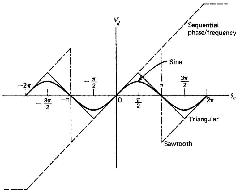
Figure 5.13 Phase detector  $s$ -curves.
