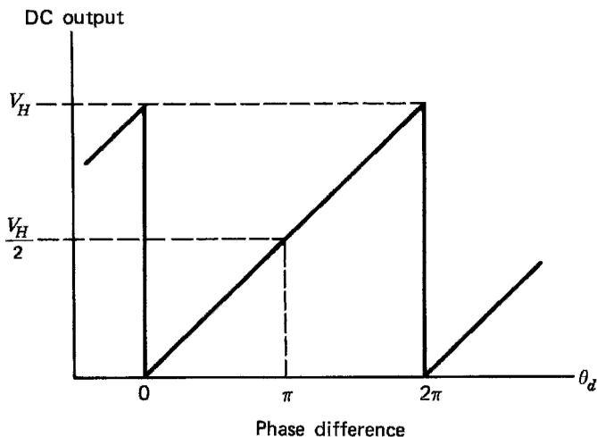
**Figure 10.7**  $s$ -Curve of a flip-flop phase detector.
