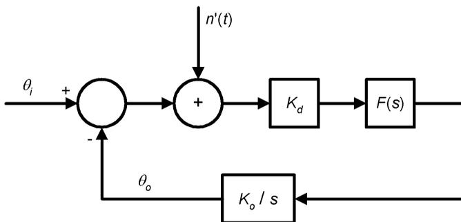
Figure 6.2 Block diagram of a linearized PLL.
