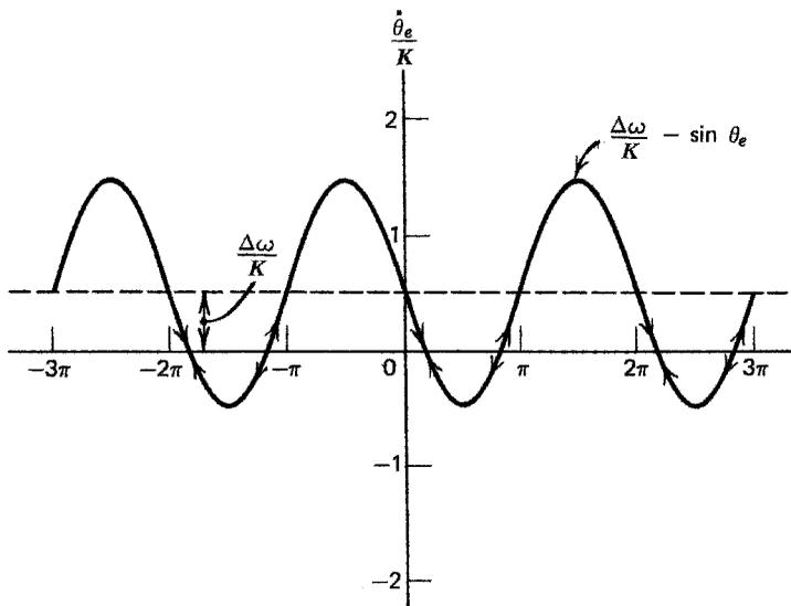
**Figure 8.1** Phase-plane plot of a first-order PLL ( $\Delta\omega/K = 0.5$ ).
