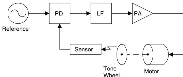
**Figure 17.7** Phaselock motor-speed control.
