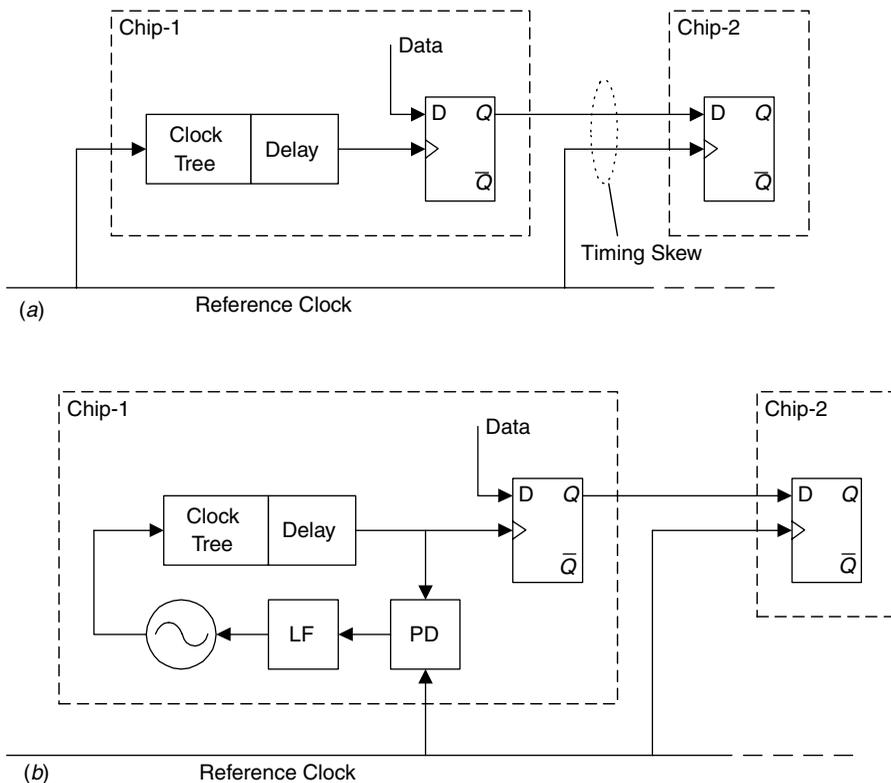
**Figure 17.5** Skew correction by a PLL: (a) origin of skew; (b) PLL correction of skew.
