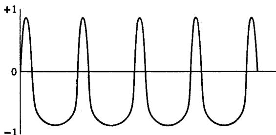
**Figure 8.5** Typical beat-note waveshape, first-order PLL,  $\Delta\omega/K = 1.10$ .
