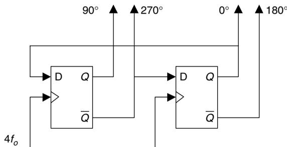
**Figure 17.4** Generation of quadrature signals by digital counters.
