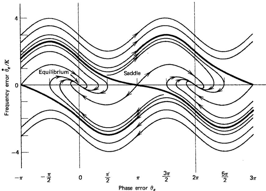
**Figure 5.14** Phase-plane portrait for a second-order type 2 PLL with  $\zeta = 1$  and a sinusoidal phase detector.
