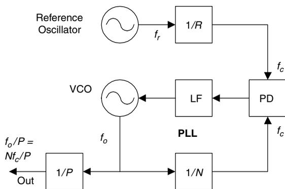
Figure 15.2 Synthesizer with a separate output divider.
