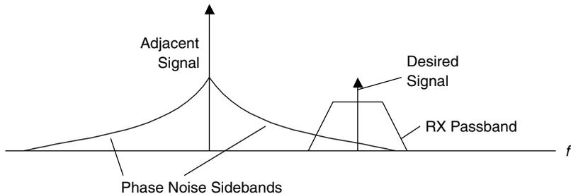
**Figure 7.5** Interference from the sidebands of an adjacent-channel signal.
