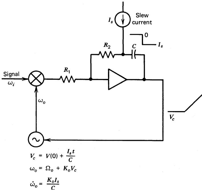
**Figure 8.10** Frequency-sweep circuit for a type 2 PLL.
