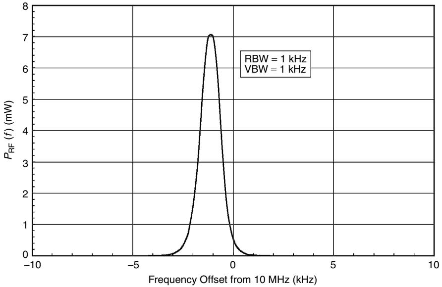
**Figure 7.3** Measured RF power spectral density  $P_{RF}(f)$  of a 10-MHz crystal oscillator (ordinate shows power in mW in a bandwidth of RBW hertz).
