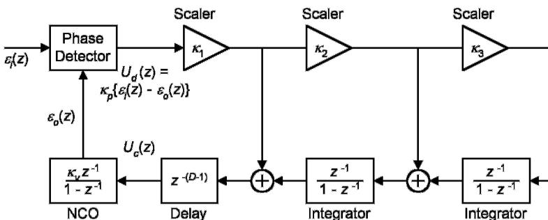
Figure 4.1 Block diagram of a type 3 DPLL.
