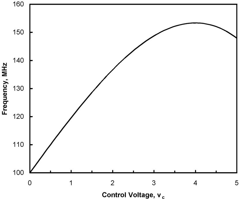
**Figure 9.5** Nonmonotonic tuning curve: beware!
