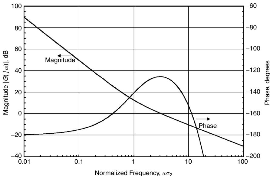
**Figure 3.16** Bode plot of a second-order type 2 PLL with an in-loop delay of  $\tau_d = \tau_2/10$ , gain  $K\tau_2 = 3$ , phase margin  $\approx 54^\circ$ , gain crossover at  $\omega\tau_2 \approx 15$ , and gain margin  $\approx 14$  dB; the same parameters as in the Nichols chart of Fig. 3.20 and the frequency-response graphs of Figs. 3C.3 and 3C.4.
