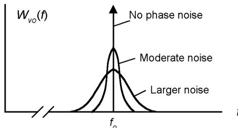
**Figure 7.1** Theoretical spectrum  $W_{v_o}(f)$  of oscillator output  $v_o(t)$ .
