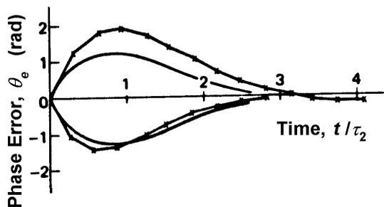
**Figure 12.3** Response of a second-order PLL to frequency steps  $\Delta\omega = \pm 2K$ . Smooth curves, response of time-continuous PLL; marked points, time-discrete response of a charge-pump PLL with  $K\tau_2 = 2$  and  $K = \omega_c/10$ . (From [12.1]; © 1980 IEEE.)
