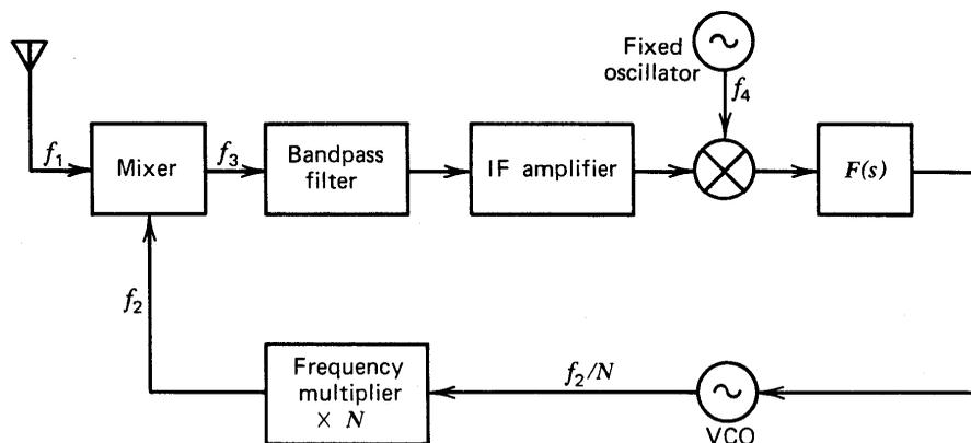
Figure 14.4 Long-loop phaselock receiver.
