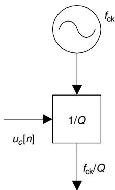
**Figure 13.1** Period DCO based on a frequency divider.
