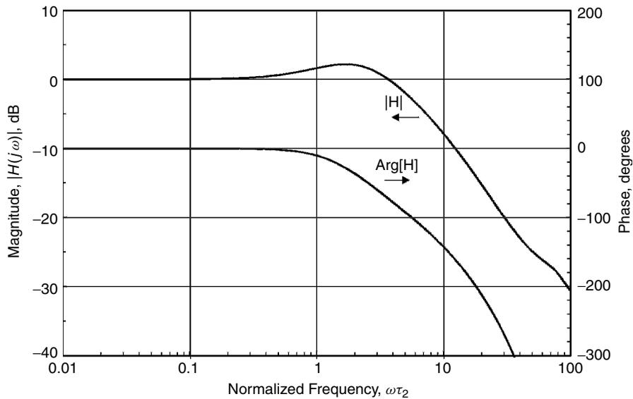
**Figure 3C.4** Frequency response of  $H(j\omega)$  for a type 2 PLL with  $K\tau_2 = 3$  and an in-loop delay of  $\tau_d = \tau_2/10$ ; the same parameters as for the Bode plot of Fig. 3.16 and the Nichols chart of Fig. 3.20.
