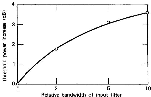
**Figure 16.9** Measured threshold increase due to the excess bandwidth of an input filter. Unity relative bandwidth corresponds to Carson's rule [eq. (16.23)]. The ordinate shows the additional signal power needed at the threshold because of a widened input bandwidth.
