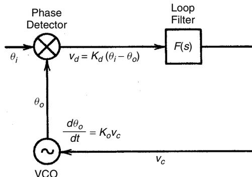
Figure 2.1 Phaselock loop: basic block diagram.
