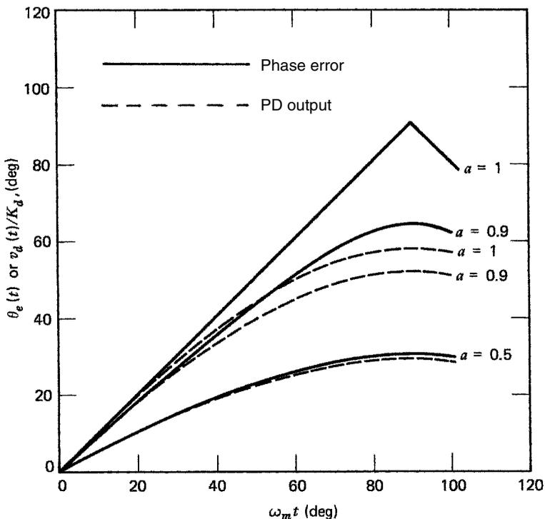
**Figure 5.17** Phase error  $\theta_e(\omega_m t)$  (solid curves) and PD output  $v_d(\omega_m t)/K_d$  (dashed curves) in a PLL with a sinusoidal phase detector in response to sinusoidal angle modulation with frequency  $\omega_m$ , based on  $v_d(t)/K_d = a \sin \omega_m t = \sin \theta_e(t)$ .
