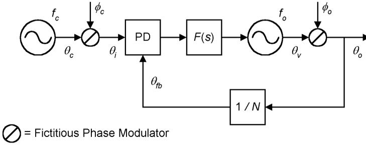
**Figure 15.8** Oscillator noise sources in a PLL synthesizer.
