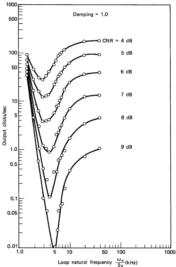
**Figure 16.10** Measured PLL click rates under the conditions of Table 16.1. Damping  $\zeta = 1$ .
