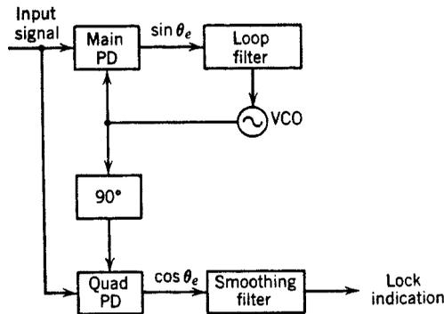
**Figure 8.14** Lock detection with a quadrature phase detector.
