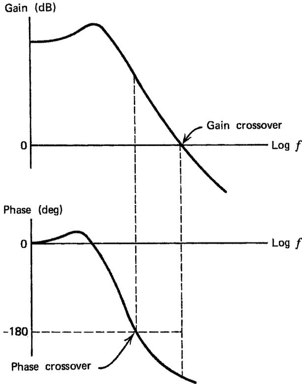
Figure 3.9 Example Bode plot of an unstable loop.
