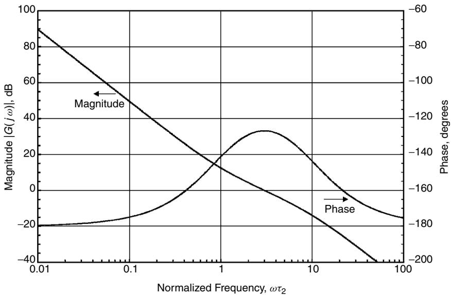
**Figure 3.14** Bode plot of a third-order type 2 PLL with  $b = 9$ ,  $K\tau_2 = 3$ , and a phase margin of  $53^\circ$ ; the same parameters as in the frequency-response graph of Fig. 2.9 and the root-locus plots labeled “ $b = 9$ ” in Figs. 3.3 and 3.4.
