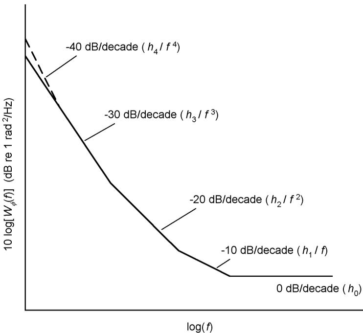
**Figure 7.9** Typical spectral components of oscillator phase noise.
