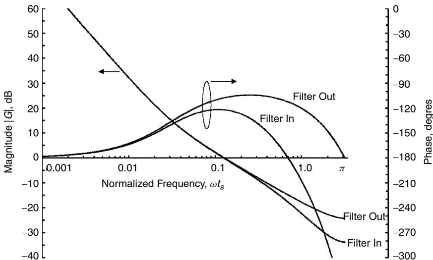
**Figure 4.10** Bode plot of a type 2 DPLL with an IIR lowpass filter in the loop. The filter pole is at  $z = 1 - a$ .  $D = 1$ ,  $\kappa = \frac{1}{8}$ ,  $\kappa_2 = \frac{1}{32}$ ,  $a = \frac{1}{2}$ .
