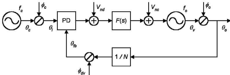
**Figure 15.11** Various noise sources in a PLL synthesizer.
