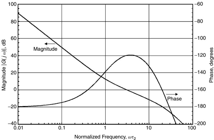
**Figure 3.15** Bode plot of a fourth-order type 2 PLL with two high-frequency poles coincident at  $s\tau_2 = -b$ , gain  $K\tau_2 = 3$ ,  $b = 30$ , phase margin =  $60^\circ$ , and gain margin  $\approx 25$  dB; the same parameters as in the root-locus plot labeled “ $b = 30$ ” in Figs. 3.6 and 3.7.
