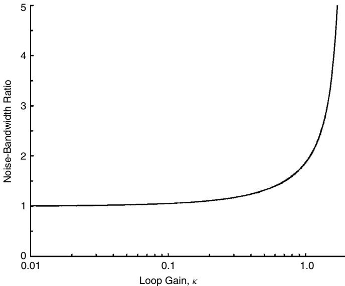
**Figure 6.3** Comparison of the noise bandwidth of the type 2 digital PLL of Table 6.1 to the time-continuous approximation of Section 4.7 ( $D = 1$ ,  $\kappa_2 = \kappa/2$ , equivalent to  $\zeta = 0.707$ ).
