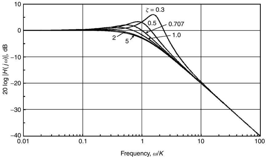
**Figure 2.6** Response  $|H(j\omega)|$  for a second-order type 2 PLL. Frequency normalized to loop gain  $K$ .
