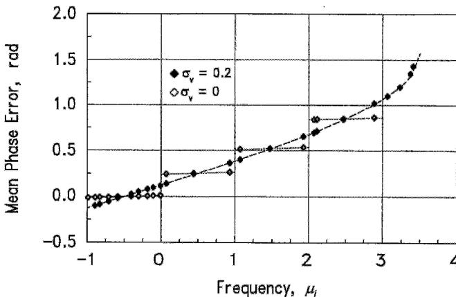
**Figure 13.19** Static phase error:  $b = 8, D = 1, L = 1, \kappa_1 = 2^{-6}, \kappa_2 = 0$ . (From [13.31]; © 1996 IEEE.)
