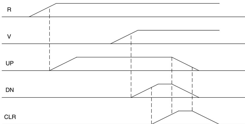
**Figure 10.10** Waveforms in a PFD; expanded time scale to show propagation delays.
