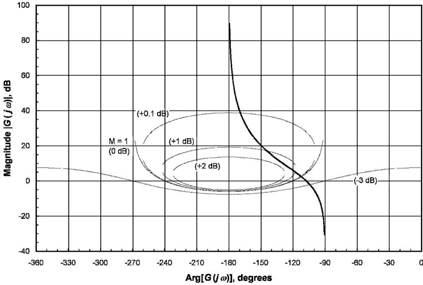
**Figure 3.18** Nichols chart of a second-order type 2 PLL with  $K\tau_2 = 3$  ( $\zeta = 0.866$ ); the same parameters as in the Bode plot of Fig. 3.13 and the frequency-response graphs of Figs. 3C.1 and 3C.2. The heavy curve is  $|G(j\omega)|$  in dB plotted against  $\text{Arg}[G(j\omega)]$  in degrees. Light oval curves are  $M$ -contours. Gaps at the ends of the ovals are due to computational quantization of the abscissa.
