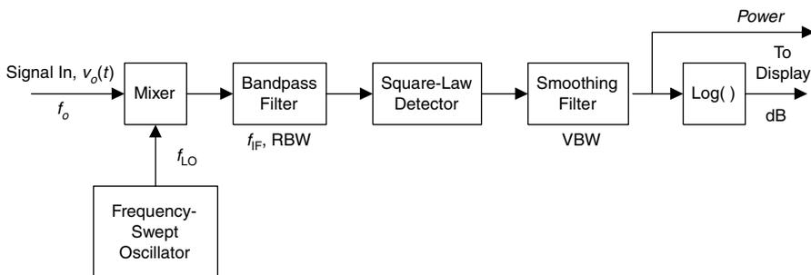
**Figure 7.2** Simplified block diagram of a spectrum analyzer.
