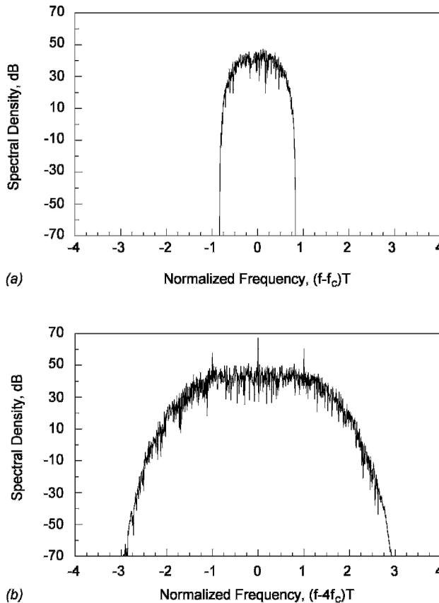
**Figure 14.2** Simulated spectra of a 4PSK signal: (a) filtered received signal  $s(t)$ ; (b) signal  $u(t)$  after  $\times 4$  frequency multiplication. Note the regenerated lines in (b): carrier at zero and symbol-rate sidelines at  $\pm 1$ . (Adapted from [14.11].)
