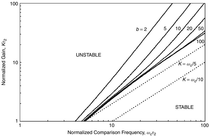
**Figure 12.2** Stability boundaries for a third-order charge-pump PLL.
