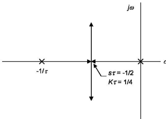
**Figure 3.1** Root locus of a second-order type 1 PLL with lag filter  $F(s) = 1/(\tau s + 1)$ .
