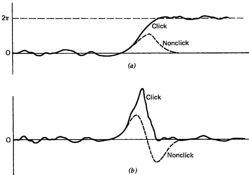
**Figure 16.7** Illustrative click waveforms: (a) phase; (b) frequency.
