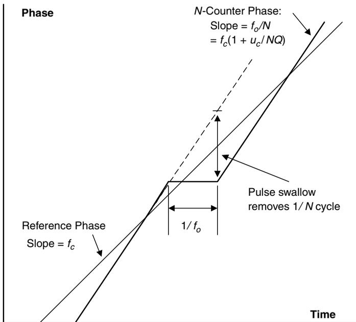
**Figure 15.6** Irregular counting in a fractional- $N$  synthesizer.
