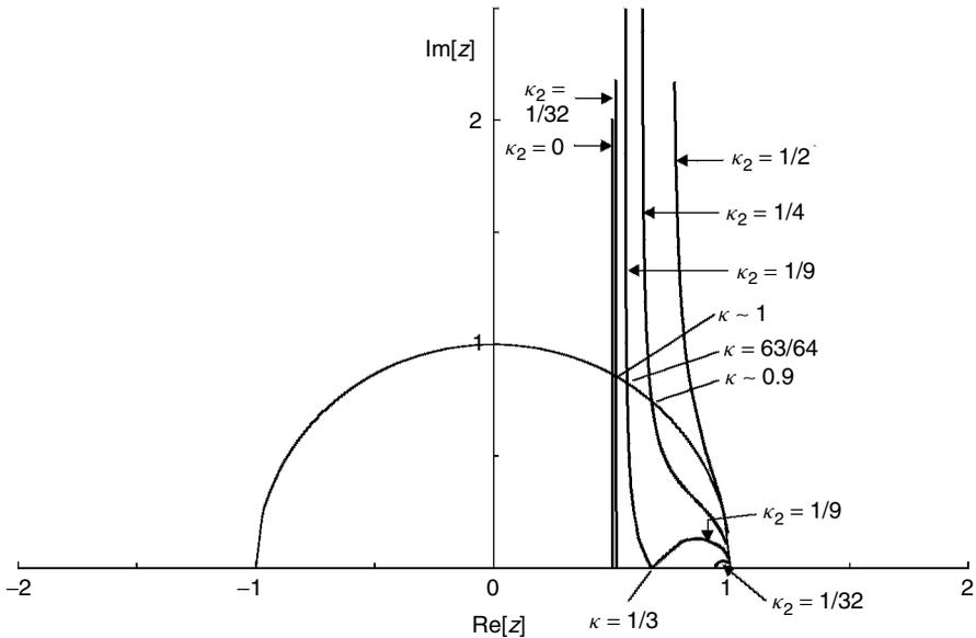
**Figure 4.3** Root-locus plots of a type 2 DPLL with  $D = 2$  and various  $\kappa_2$ . Real poles and the lower half plane are omitted.
