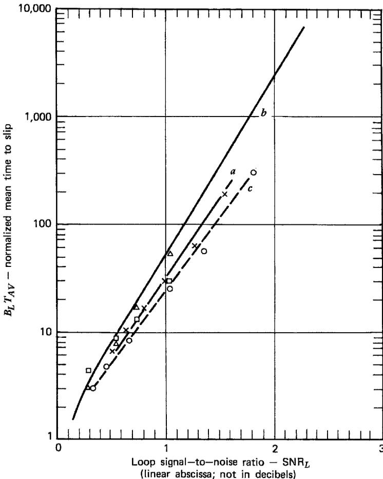
**Figure 6.5** Mean time to first slip. (a) Experimental data [6.4] for a second-order type 2 PLL with  $\zeta = 0.707$ , x-marker. (b) Exact result for a first-order PLL, eq. (6.30). (c) Simulation results [6.10] for a second-order type 2 PLL with  $\zeta = 0.707$ , circle-marker. (d) Simulation results [6.9] for a second-order type 2 PLL with  $\zeta = 1.4$ , triangle-marker. (e) Simulation results [6.9] for a second-order type 2 PLL with  $\zeta = 0.35$ , square-marker.
