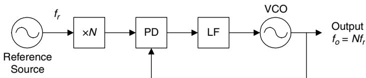
Figure 17.1 Harmonic-locked oscillator.
