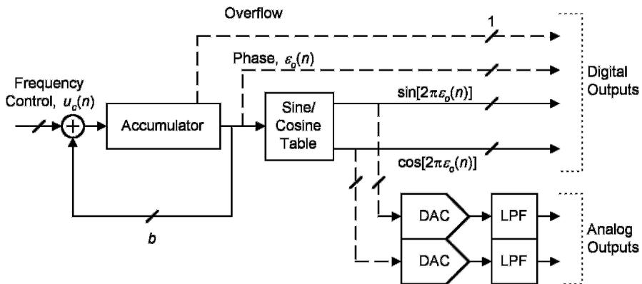
Figure 9.3 Number-controlled oscillator (NCO), illustrating various output options.
