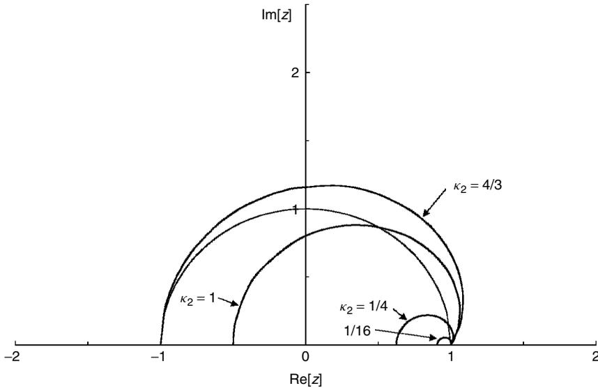
**Figure 4.4** Root-locus plots of a type 3 DPLL with  $D = 1$ , various  $\kappa_2$ , and  $\kappa_3 = \kappa_2/4$ . Zeros are coincident by the choice of  $\kappa_3$ . Real poles and the lower half plane are omitted.
