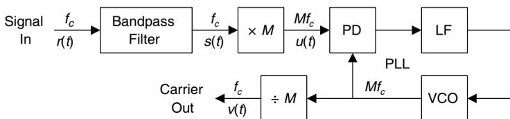
**Figure 14.1** Carrier regenerator.
