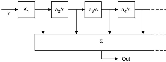
**Figure 3B.2** Cascade integrators, parallel adder configuration for the P + I portion of a loop filter.
