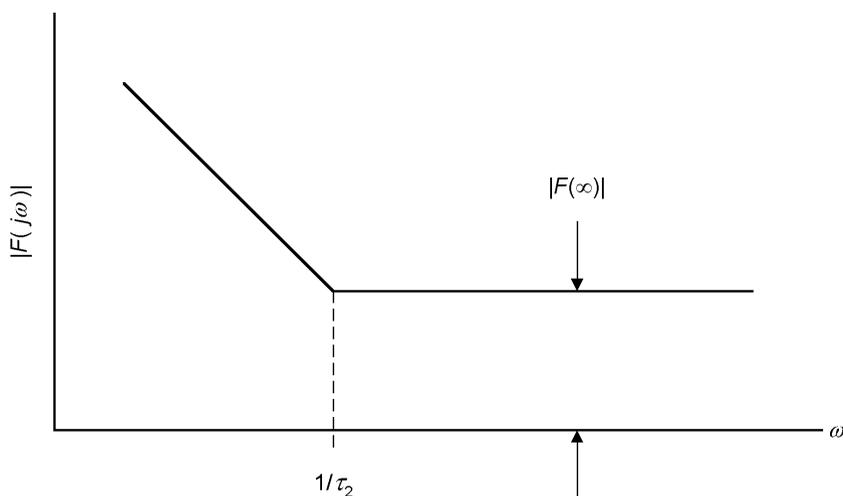
**Figure 8.3** Amplitude response of a proportional-plus-integral loop filter.
