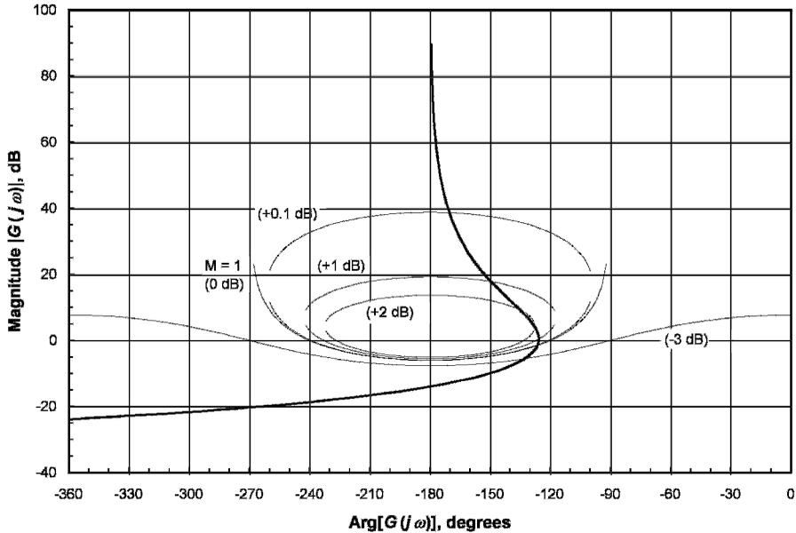
**Figure 3.20** Nichols chart of a second-order type 2 PLL with an in-loop delay of  $\tau_d = \tau_2/10$ , gain  $K \tau_2 = 3$ , phase margin  $\approx 54^\circ$ , and gain margin  $\approx 14$  dB; the same parameters as in the Bode plot of Fig. 3.16 and the frequency-response graphs of Figs. 3C.3 and 3C.4.
