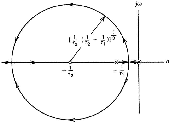
**Figure 3.2** Root locus of a second-order type 1 PLL with lag-lead filter  $F(s) = (s\tau_2 + 1)/(s\tau_1 + 1)$ .
