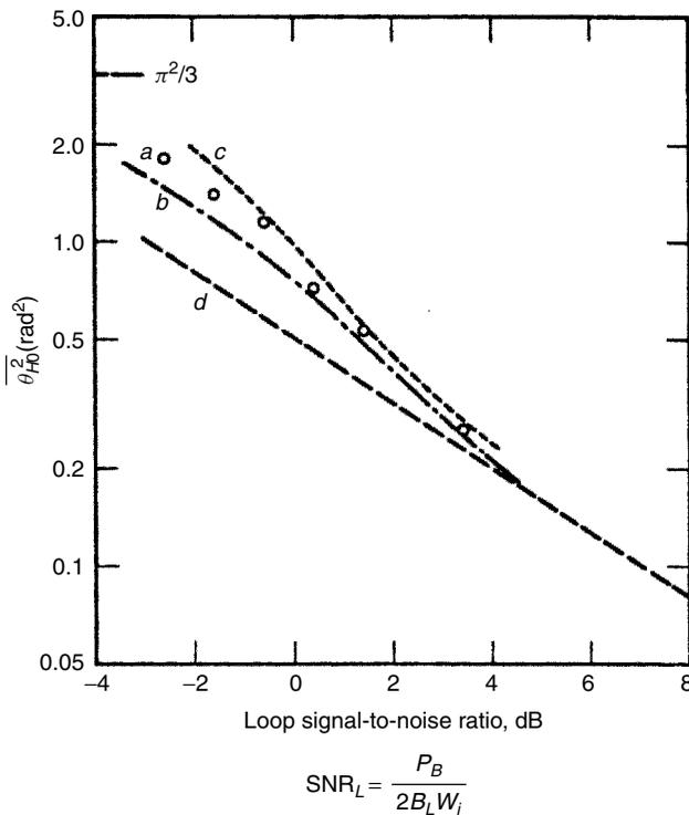
**Figure 6.4** Phase-error variance. (a) Experimental data [6.4] for a second-order type 2 PLL with  $\zeta = 0.707$ . (b) Exact nonlinear analysis [6.2] for a first-order PLL. (c) Approximate nonlinear analysis [6.3, 6.8] for a type 2 PLL,  $\zeta = 0.707$ . (d) Linear approximation, eq. (6.25).
