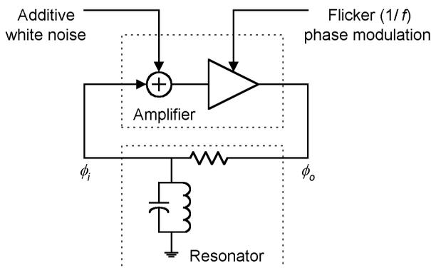
Figure 9.1 Oscillator block diagram illustrating Leeson’s model.
