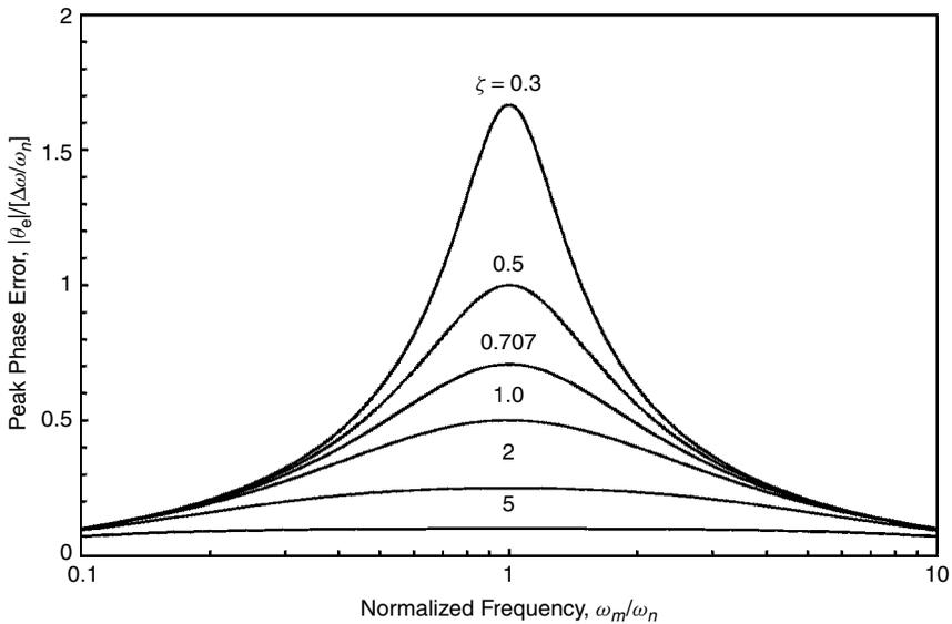
**Figure 5.12** Peak steady-state phase error of a second-order type 2 PLL due to sinusoidal FM with peak deviation  $\Delta\omega$  and modulation frequency  $\omega_m$ .
