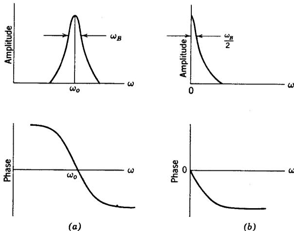
**Figure 14.6** Transfer characteristics of a bandpass filter: (a) bandpass transfer function; (b) equivalent modulation transfer function.
