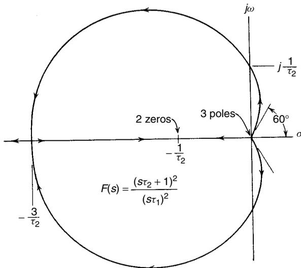
**Figure 3.5** Root locus of a third-order type 3 PLL with two zeros coincident at  $s\tau_2 = -1$ . Intersection with the imaginary axis occurs for  $K\tau_2 = \frac{1}{2}$ , and intersection with the real axis occurs for  $K\tau_2 = \frac{27}{4}$ .
