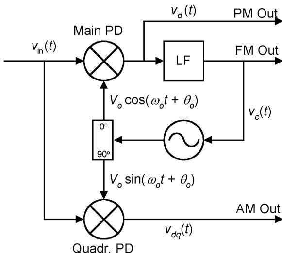
Figure 16.2 Demodulation options for a PLL.
