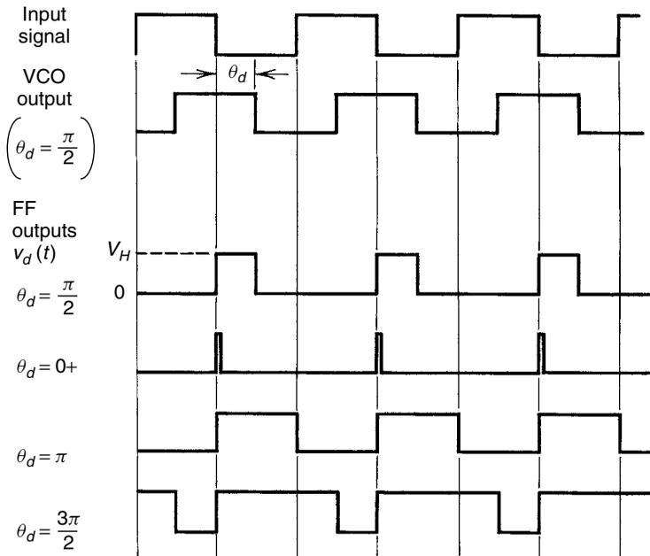
Figure 10.6 Waveforms in an RS flip-flop phase detector.
