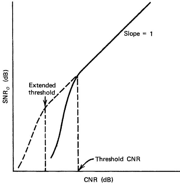
Figure 16.5 FM threshold effect on  $SNR_o$ .
