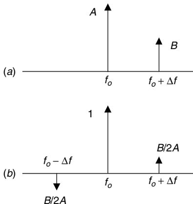
**Figure 7.11** Interference-to-phase conversion in a limiter.
