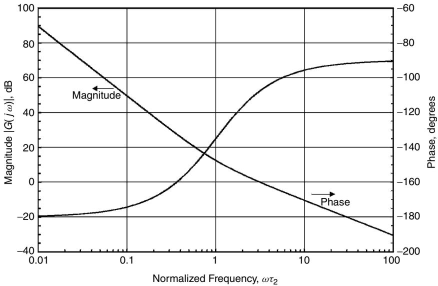
**Figure 3.13** Bode plot of a second-order type 2 PLL with a zero at  $s\tau_2 = -1$ , gain  $K\tau_2 = 3$  ( $\zeta = 0.866$ ), and a phase margin of  $72^\circ$ ; the same parameters as in the Nichols chart of Fig. 3.18 and the frequency-response graphs of Figs. 3C.1 and 3C.2.
