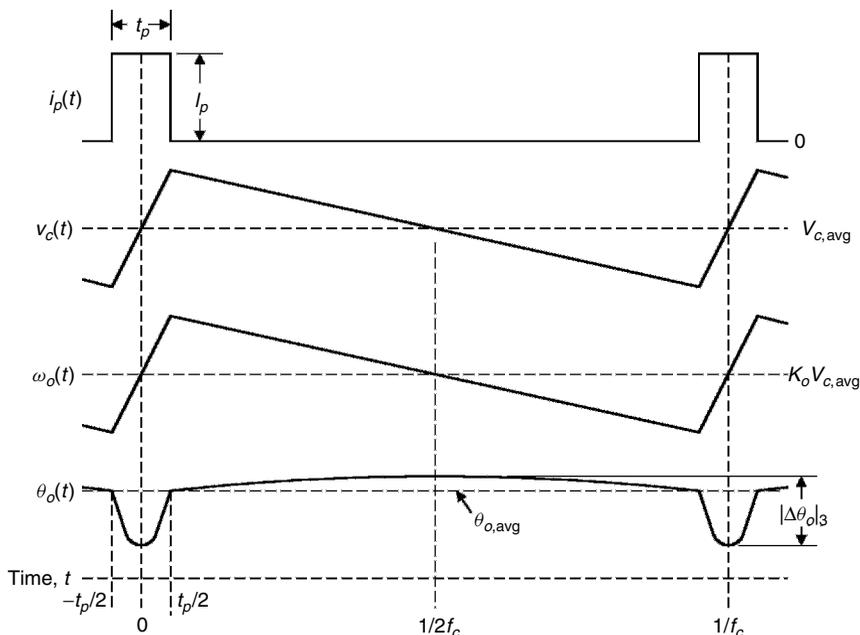
**Figure 12.4** Ripple waveforms in a third-order charge-pump PLL.
