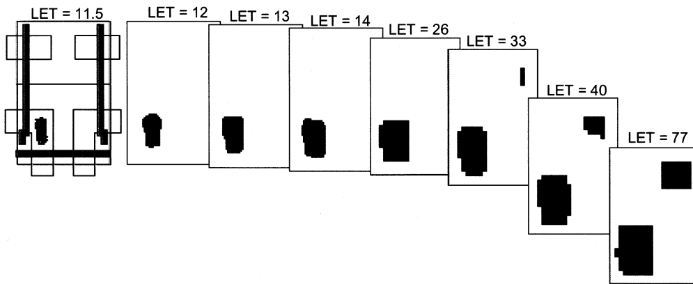
Fig. 11. Evolution of the soft-error sensitive area (black regions) of a 256K SRAM unit cell without feedback resistors as a function of increasing ion LET. Note increasing sensitive area of reverse-biased NMOS drain. At an LET of 33 MeV-cm 2 /mg, the reverse-biased PMOS drain also becomes SEU-susceptible.
