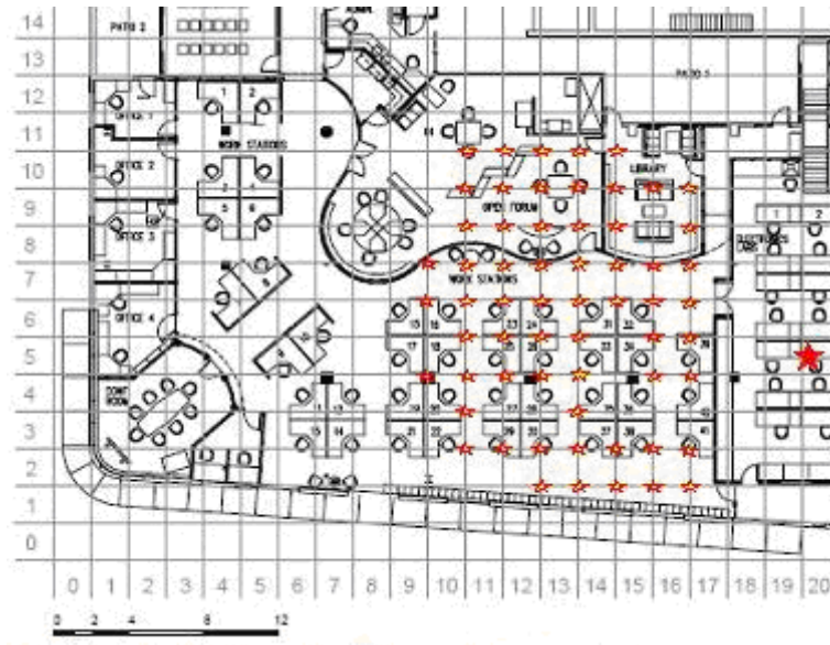
Figure 6.1: BWRC floor plan with transmitter and receiver locations
