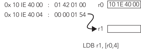
FIGURE 4-6: Loading a register from pointer with offset
