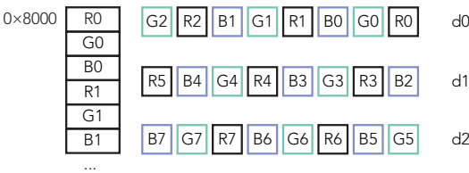
FIGURE 8-1: Loading RGB data with a linear load
