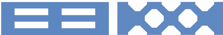
Fig. 4.2 Differently slotted wires, left rectangular slots, right octagonal cutouts, that support the bamboo effect [KRS+97, KWA+13]
