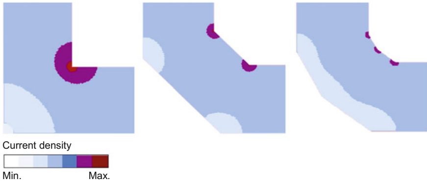
Fig. 2.8 Current-density visualization of different corner-bend angles of a wire on an analog integrated circuit, left 90°, middle 135°, and right 150°. It shows that 90° corner bends must be avoided, since the current density in such a bend is significantly higher than that in oblique angles of, for example, 135°
