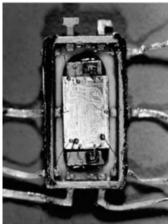
Figure 1.1 First integrated circuit chip. (Courtesy of Texas Instruments, Inc.)
