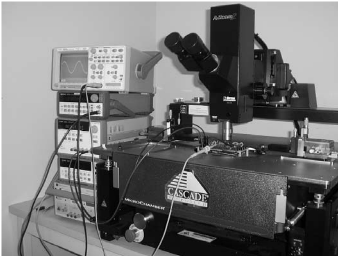
Figure 8.16 The equipment used for testing the imager with polystyrene microsphere cells.
