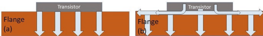
Fig. 8.7 Modeling heat conducting via die contact area (a), and via whole flange area (b)
