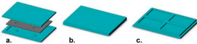
Fig. 10.4 TPG composites are made by encapsulating TPG in metal cladding. The composites can be machined for specific applications. Steps from left to right are (a) cutting TPG and inserting into metal clad; (b) bonding; (c) post-bonding machining
