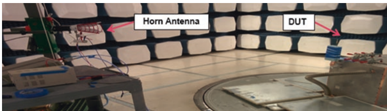
Fig. 4.11 Semi-anechoic chambers lab for far-field electromagnetic measurements. Courtesy of Missouri University of Science and Technology
