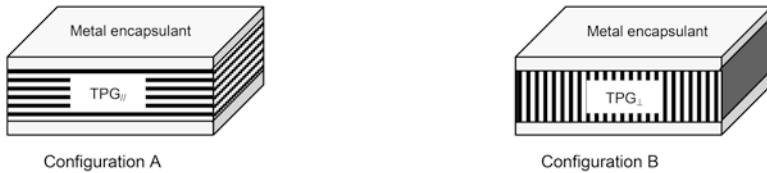
Fig. 10.8 Sketches of two common TPG tile orientations with graphene basal planes parallel to metal layers ( Configuration A ) and perpendicular to the metal layers ( Configuration B ), respectively
