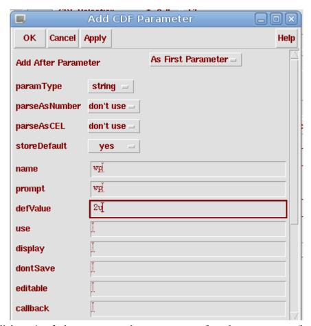
Then click on **Apply** button, repeat the same process for other parameters (lp,wn and ln) also and finally click OK. Now your **Component parameters** should like shown below(of-course the values may be different).
