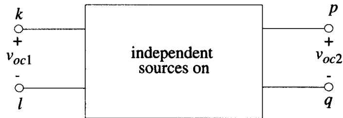
Figure 8.21 Measuring the open circuit voltages at two ports.
