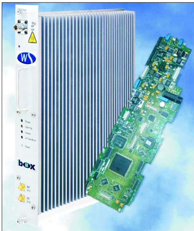
Figure 58 · A multi-carrier S-band transmitter with digital predistorter (courtesy WSI).
