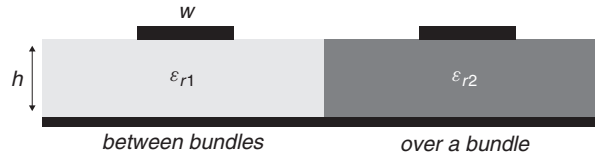
Figure 6-17 Two-dimensional fiber-weave modeling structure.
