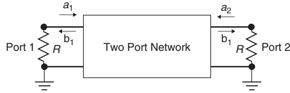
Figure 9-7 Two-port model used to define S -parameters.
