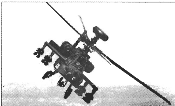
Figure 1.13 The Longbow K a band (35 GHz) fire control radar for the U.S. Army's Apache helicopter shown mounted in a radome on top of the helicopter mast that rotates the blades. | (Courtesy of Northrop Grumman Corporation.)
