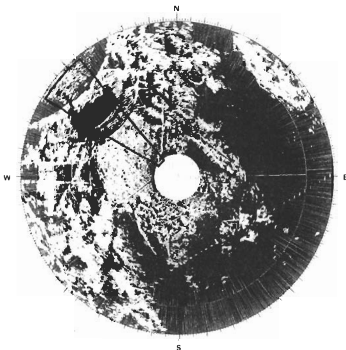
Figure 7.7 PPI clutter map at Gull Lake West, Manitoba, Canada. Cells with \sigma^0 F^4 \geq -40 dB are shown in white.
