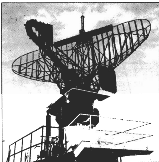
Figure 9.8 Signaal LW08 2D (Jupiter) L-band fan-beam air and surface surveillance radar with an elliptical shape fan-beam antenna fed by a horn (on the left). The reflector surface is a mesh, the horizontal antenna mounted on the top is for IFF (identification friend or foe). At the middle right can be seen a fin which is added to the back of the antenna to counterbalance the wind forces on the reflector in the position of the worst yawing moment.
