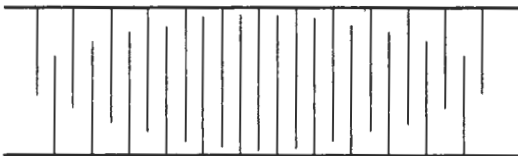
Figure 6.16 Interdigital transducer (nondispersive) showing overlap of the comb fingers to provide an amplitude weighting along the pulse.
