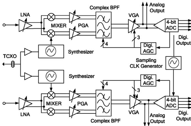
Fig. 2. Block diagram of the GNSS receiver.
