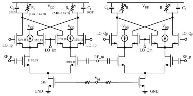
Fig. 6. Schematic of the mixer.
