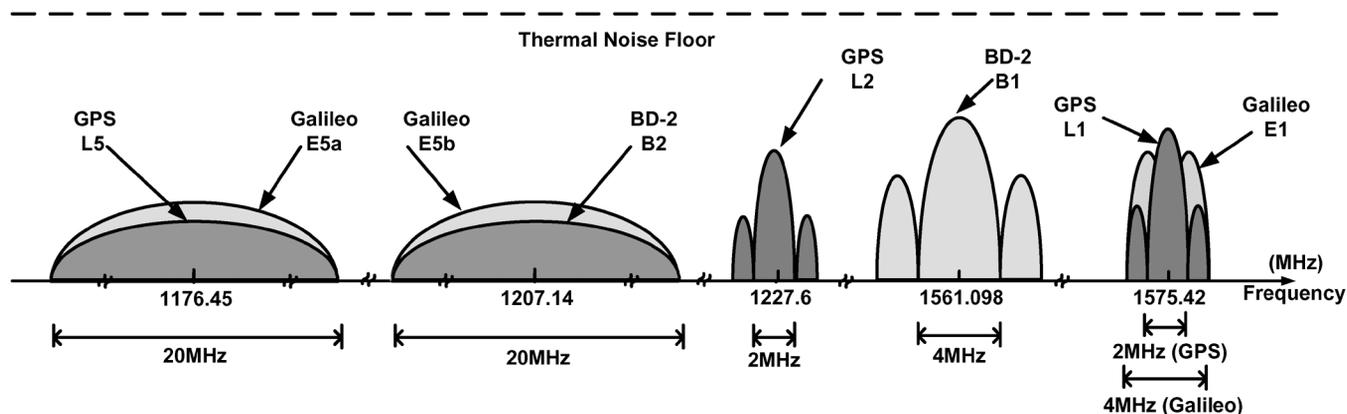
Fig. 1. Band spectrum of the GNSS signals.
