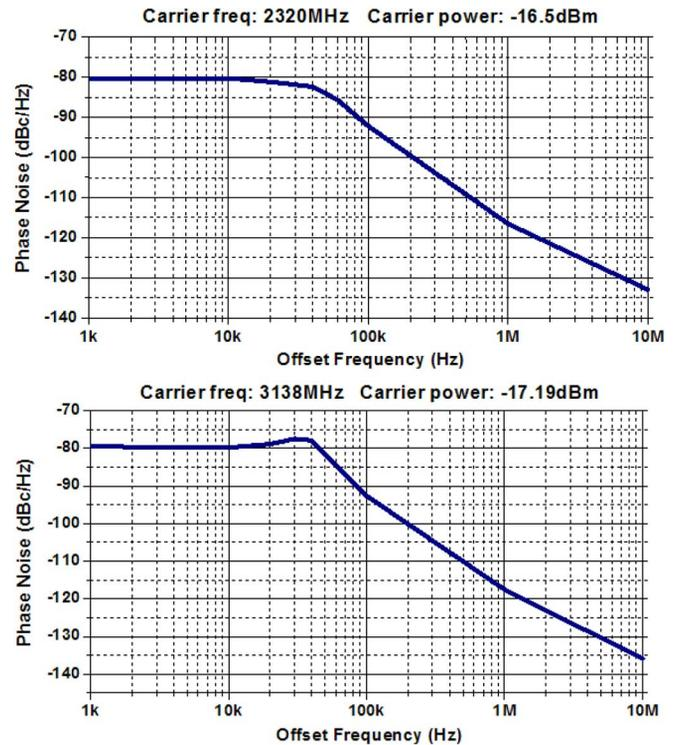
Fig. 14. Measured phase noise (frequency =  $2 \times$  LO).
