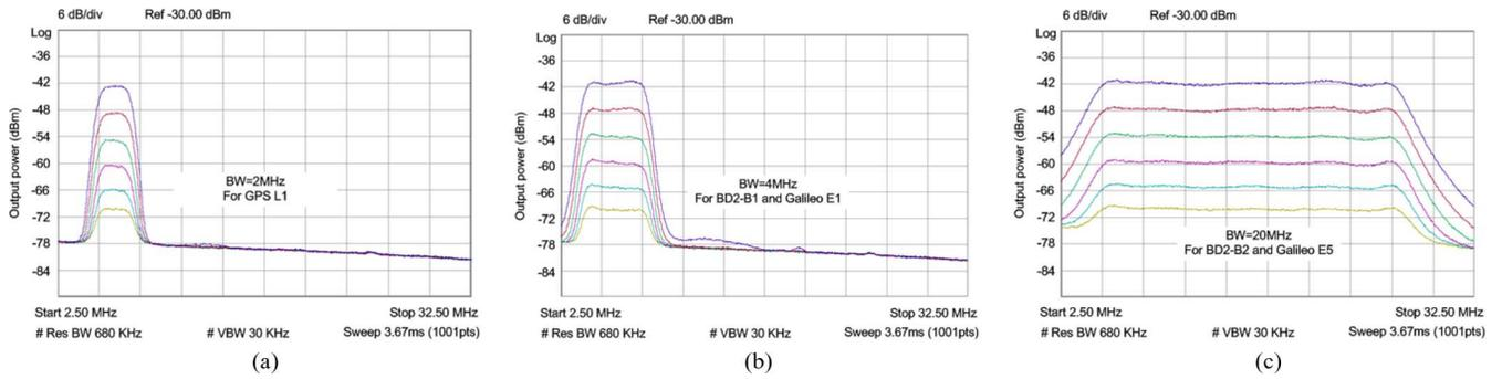
Fig. 15. Measured output spectrum of ABB with the tuning of IF, BW and gain. (a) GPS L1 mode. (b) BD-2 B1 or Galileo E1 mode. (c) BD-2 B2 and Galileo E5 mode.
