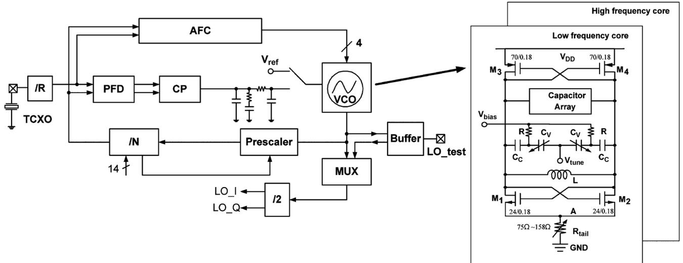
Fig. 11. Block diagram of the integer- $N$  PLL and schematic of the dual-core VCO.
