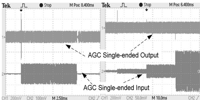
Fig. 18. Measured transient response of the digital AGC loop.
