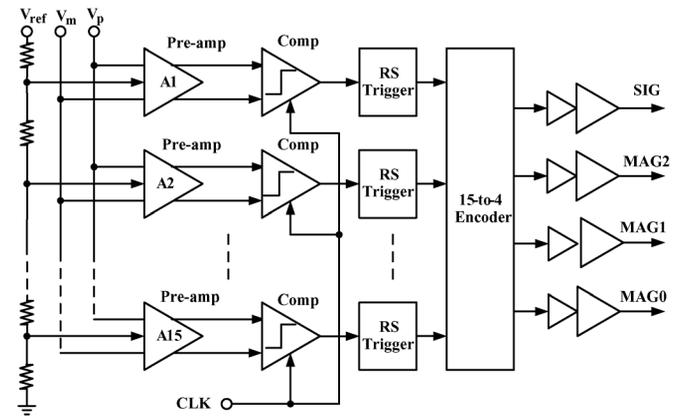
Fig. 10. Block diagram of the 4-bit flash ADC.
