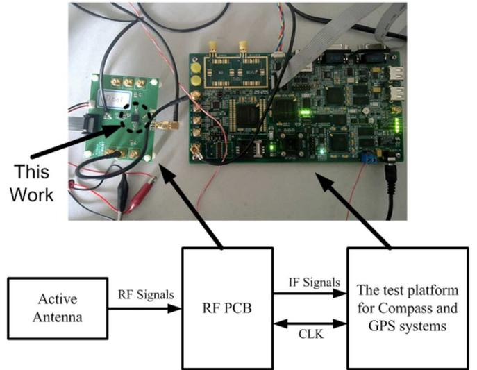
Fig. 21. Test bench of the GNSS RF receiver.
