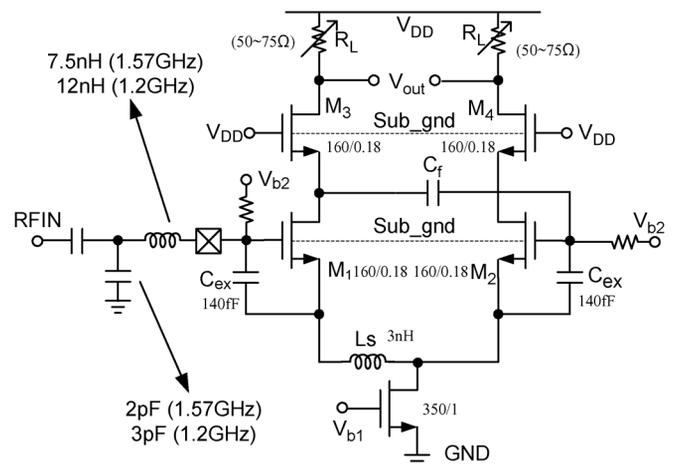
Fig. 5. Schematic of the dual-band LNA and matching network.
