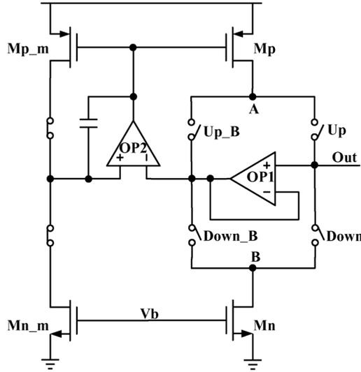
Fig. 12. Schematic of the CP.
