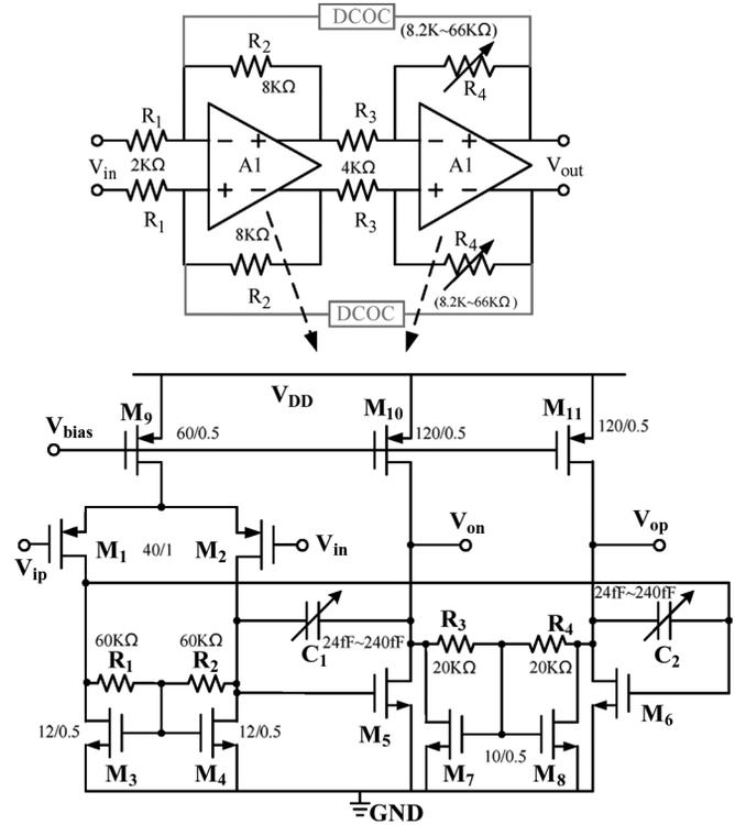
Fig. 7. Schematic of the PGA.
