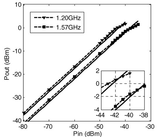
Fig. 20. Input-referred 1-dB compression point at minimum gain setting.
