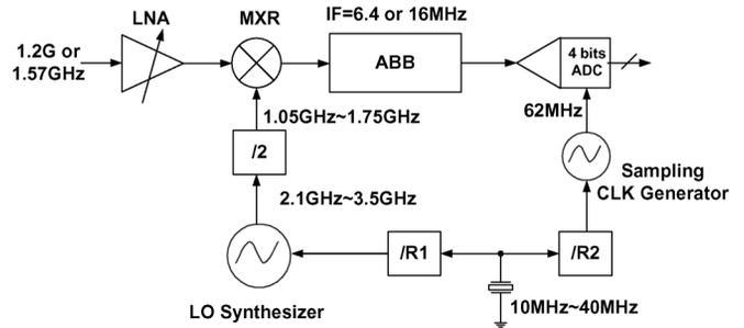
Fig. 3. Frequency plan of the proposed GNSS RF receiver.
