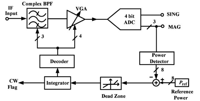
Fig. 9. Block diagram of the digital AGC.
