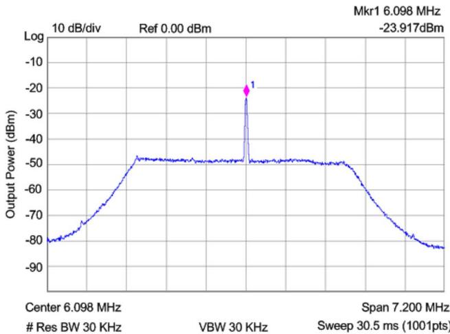
Fig. 16. Measured IF output spectrum of the GNSS RF receiver with  $-100$ -dBm RF input signal in BD-2 B1 mode.
