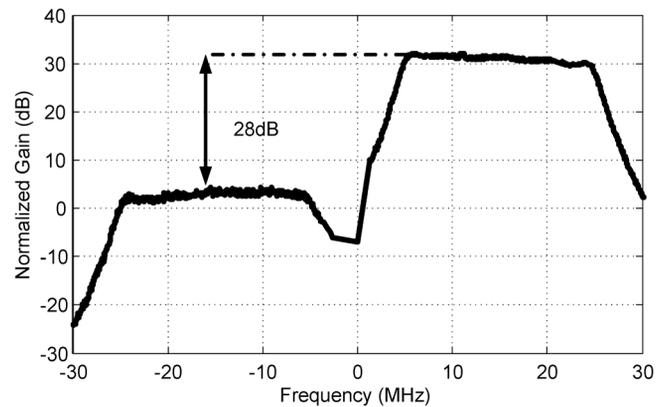
Fig. 19. Measured IMRR at BW of 20 MHz.
