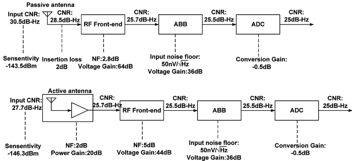
Fig. 4. Noise and gain lineup of the proposed RF receiver in the case of a passive or an active antenna.
