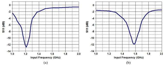
Fig. 17. Measured input S11. (a) 1.2-GHz band. (b) 1.57-GHz band.
