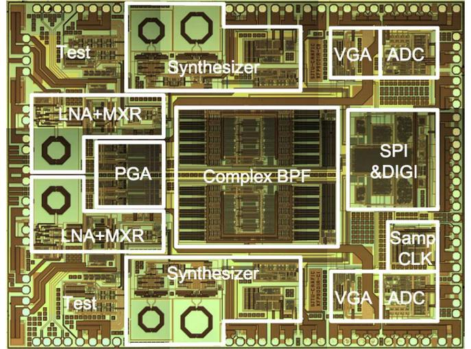
Fig. 13. Chip microphotograph of the dual-channel GNSS receiver.
