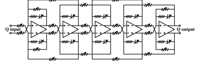
Fig. 8. Schematic of the complex BPF.
