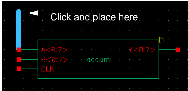
Figure 3-14 Placing the First Position Of The Wide Wire
