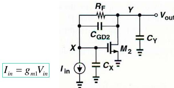
$$(I_{in} + V_X C_X s) \left( R_F \parallel \frac{1}{C_{GD2} s} \right) + V_X = V_{out} \text{ and } -V_{out} C_Y s - g_{m2} V_X = I_{in} + V_X C_X s$$
