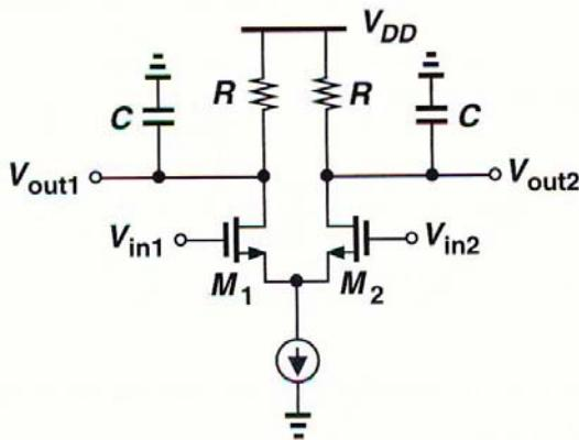
For moderate input swings, the V-to-I characteristic of the differential pair is:
