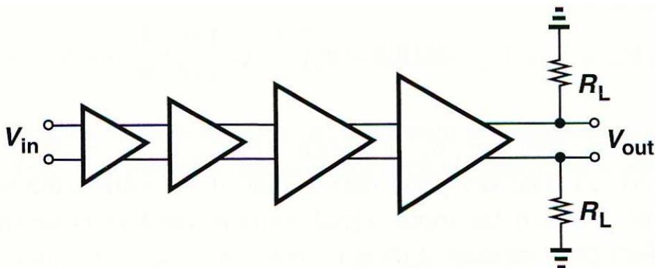
For 50- $\Omega$  loads, it must employ high currents and large output transistors in the last stage. ➔ Large input capacitance
