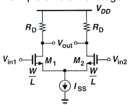
$$V_{out} = g_m (V_{in1} - V_{in2}) R_D$$
