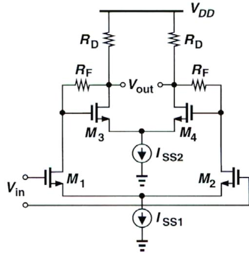
$$V_{DD,\min} = \frac{I_{ss1} + I_{ss2}}{2} R_D + \frac{I_{ss1}}{2} R_F + V_{GS3,4} + V_{ISS2}$$
