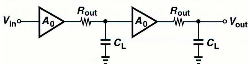
Overall transfer function:  $H(s) = \left( \frac{A_0}{1 + \frac{s}{\omega_0}} \right)^2$        $\omega_0 = \frac{1}{R_{out} C_L}$
