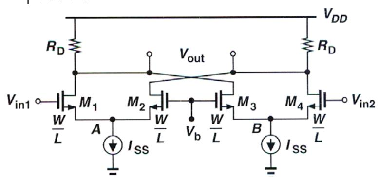
$$V_{out} = g_m (V_{in1} - V_{in2}) R_D$$
