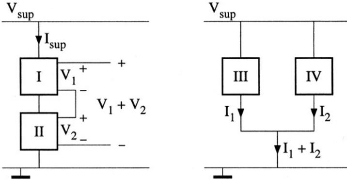
Figure 3.1: The change from series-connected blocks to parallel-connected blocks for the addition of two signals for low-voltage design.
