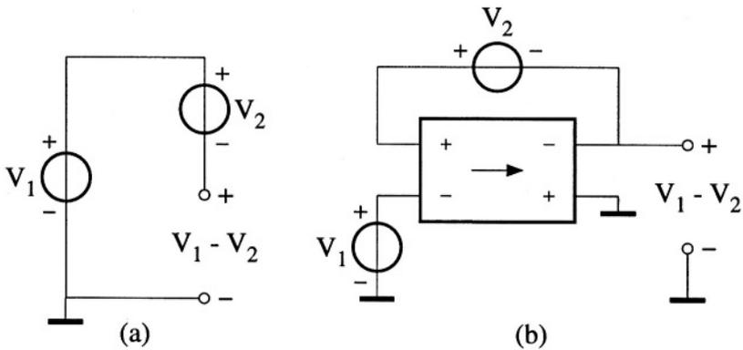
Figure 6.12: a) Passive and b) active addition of two voltages.
