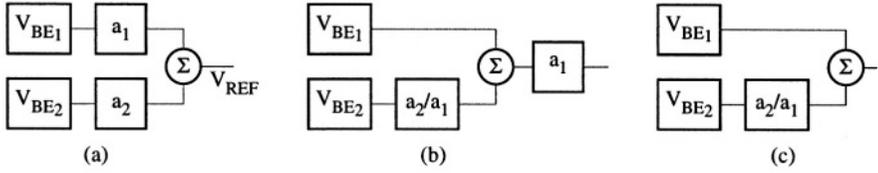
Figure 6.26: Simplification of a second-order compensated bandgap reference.
