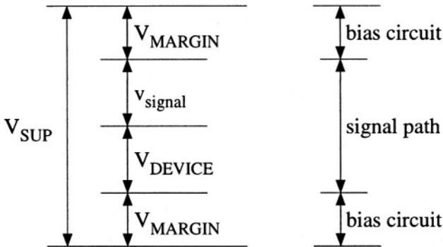
Figure 3.2: The division of the available supply voltage between the signal-path and bias circuit.
