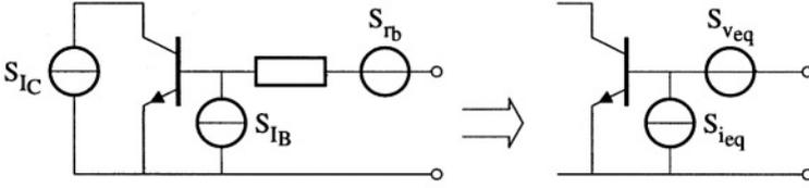
Figure 6.9: The noise sources of a bipolar transistor which have to be transformed to an equivalent noise source at the output of the cell.
