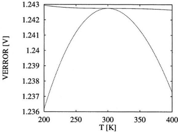
Figure 6.6: The remaining temperature dependency for a first-order (lower function) and a second-order (upper function) compensated bandgap reference with reference voltage equal to  $V_G'(0)_1$ .
