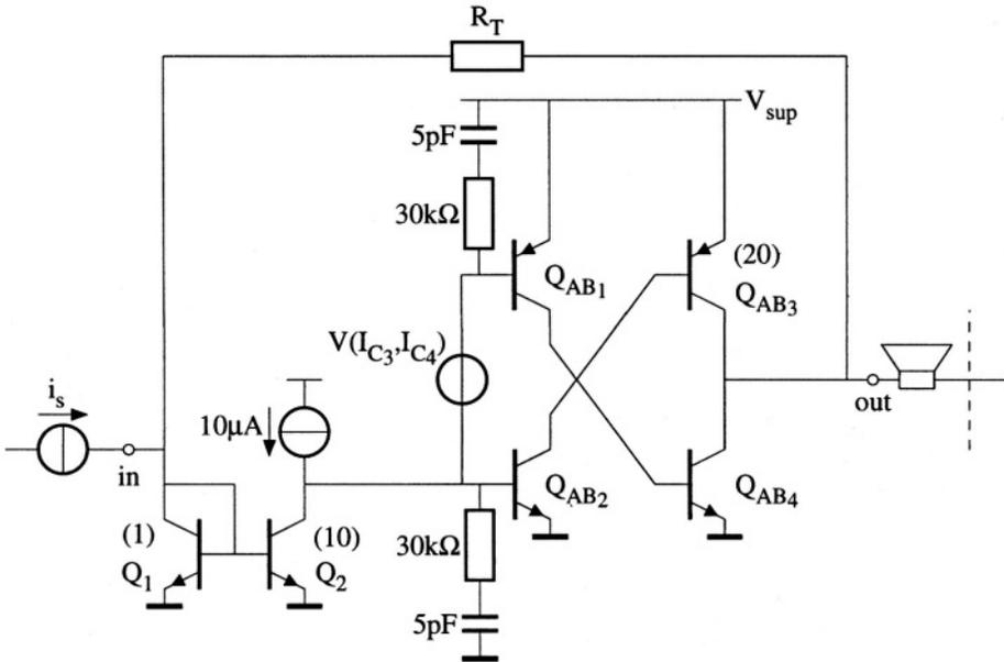
Figure B.9: The implementation of the input stage to obtain acceptable loop gain
