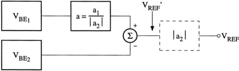
Figure F.1: Block diagram of a simplified first-order compensated bandgap reference
