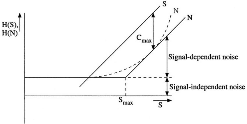
Figure 2.9: The effect of a limited dynamic range on the entropy of the noise,  $H(N)$ , in the channel.
