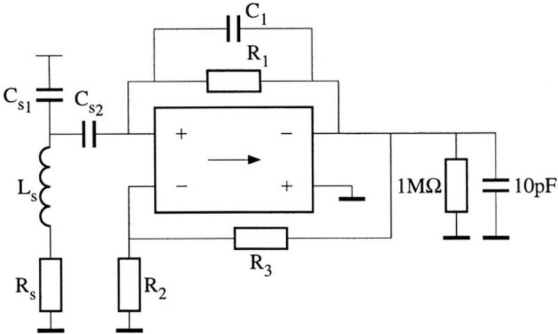
Figure 5.28: The configuration of the tapped-resonator oscillator.
