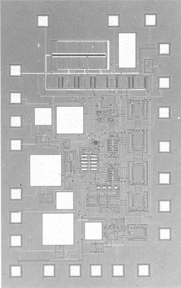
Figure D.12: A chip photo of the bandgap reference
