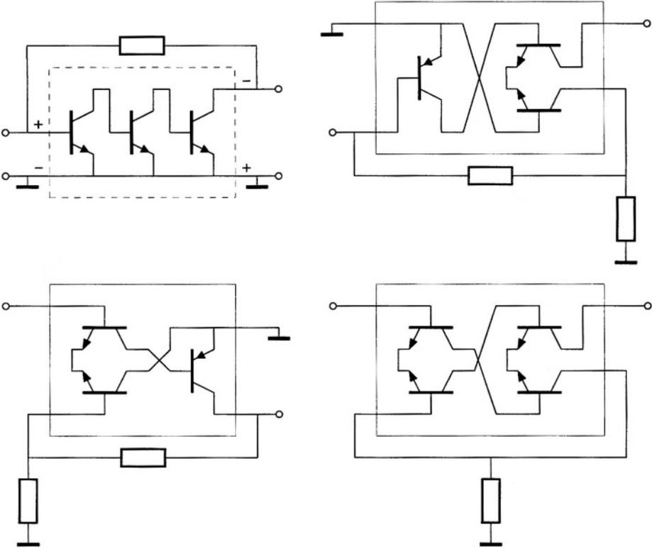
Figure A.1: The four possible single-loop amplifiers.
