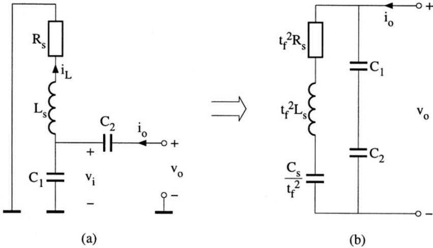
Figure 5.9: a) A capacitively tapped resonator and b) its equivalent circuit diagram,  $C_s = C_1 + C_2$ .
