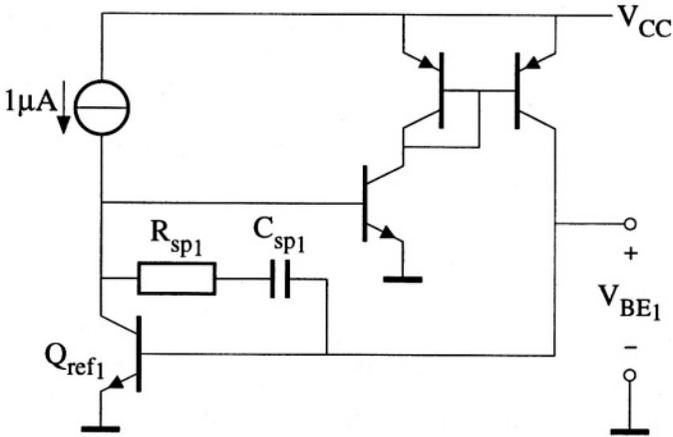
Figure F.3: Implementation of the first base-emitter voltage generator
