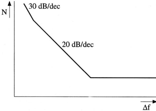
Figure 5.6: A log-log plot of a typical output spectrum of an oscillator.
