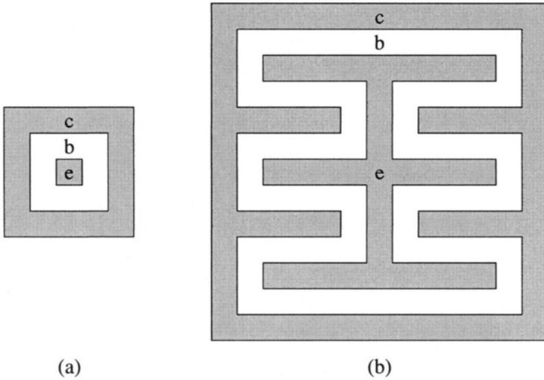
Figure 6.18: Two lateral PNP transistors. a) a small one with  $A_{col}/A_{eff} \approx 2$  and b) a large one with  $A_{col}/A_{eff} \approx 1$ .
