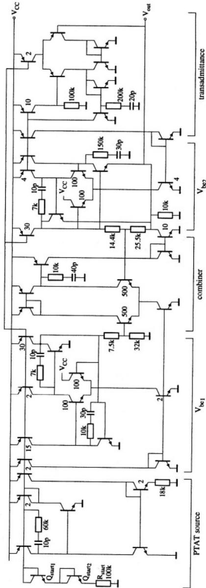
Figure D.11: The total circuit of the second-order compensated bandgap reference
