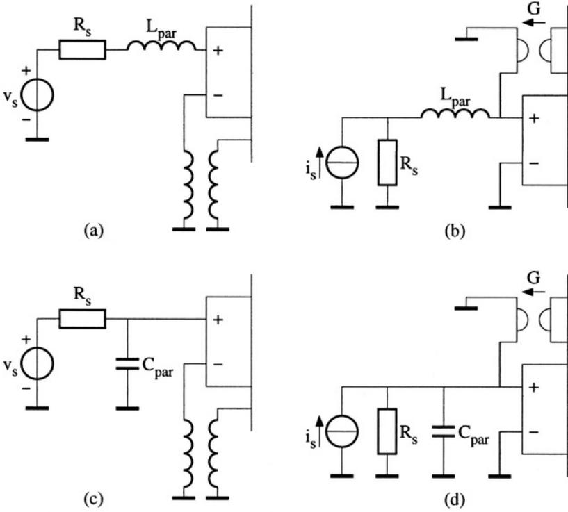
Figure 3.12: A voltage and a current input each with a parasitic capacitance or a parasitic inductance.
