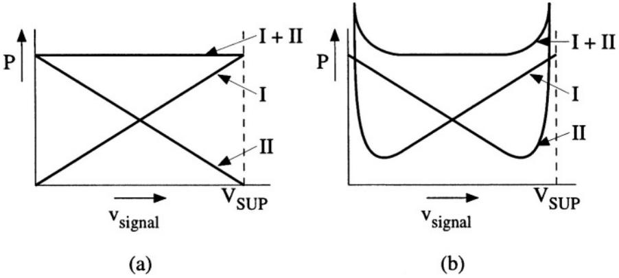
Figure 3.3: Schematic representation of the power consumption for a given signal current:  $I$ , the power used for the signal and  $II$ , the power used for the signal-path devices plus the bias circuit. a) In the ideal case and b) the non-ideal case.
