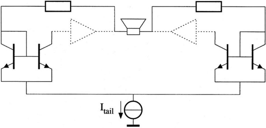
Figure B.11: Solution to the common-mode instability
