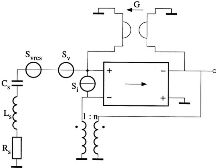
Figure 5.8: The equivalent noise sources,  $S_v$  and  $S_i$ , of the nullor implementation.
