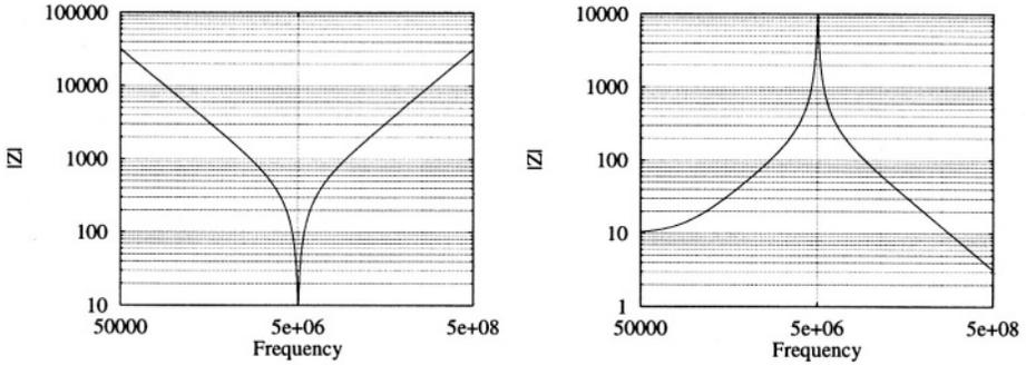
Figure 5.5: Typical plots of the impedance versus frequency of a series and a parallel resonator,  $C_s = 100$  pF,  $L_s = 10$   $\mu$ H and  $R_s = 10$   $\Omega$ .
