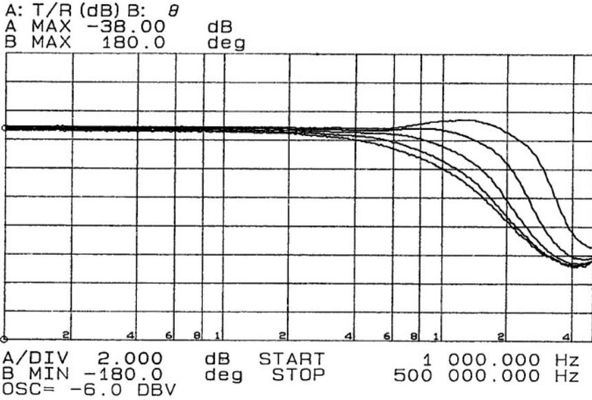
Figure B.13: The transfer as a function of the frequency with the amplitude of the input signal as a parameter
