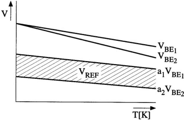
Figure 6.5: The principle of a first-order compensation using two base-emitter voltages.
