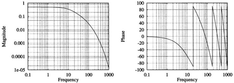
Figure 3.19: The transfer of a distributed-network voltage divider.
