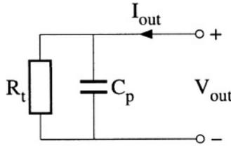
Figure 5.17: The equivalent circuit diagram of the tapped resonator at  $\omega = \omega_{osc}$ .
