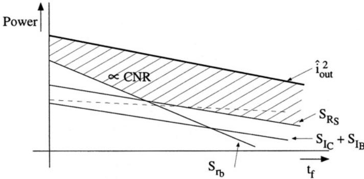
Figure 5.13: The CNR of an oscillator as a function of the tap factor.
