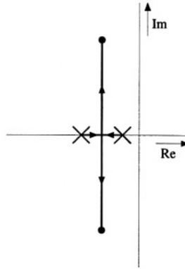
Figure 4.6: A typical root locus of a non-compensated amplifier.
