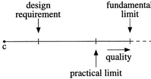
Figure 2.4: The quality of a design aspect related to requirements and limits.
