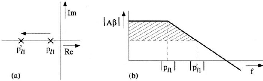
Figure 4.8: The basic idea of resistive broadbanding. The influence on a) the pole-zero plot and b) the loop gain.
