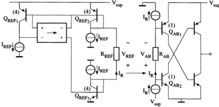
Figure B.4: The principle of the AB control voltage
