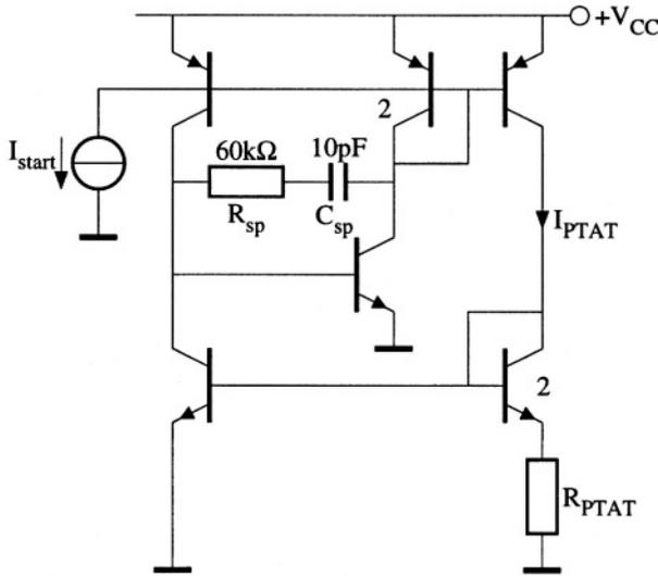
Figure D.10: A PTAT current source
