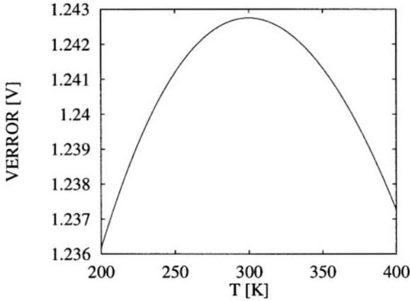
Figure 6.4: The remaining temperature dependency for a first-order compensated bandgap reference.
