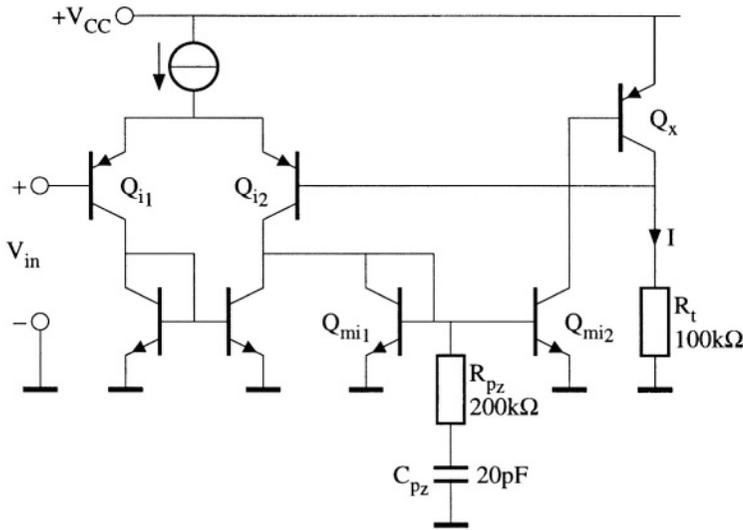
Figure D.9: The transadmittance amplifier
