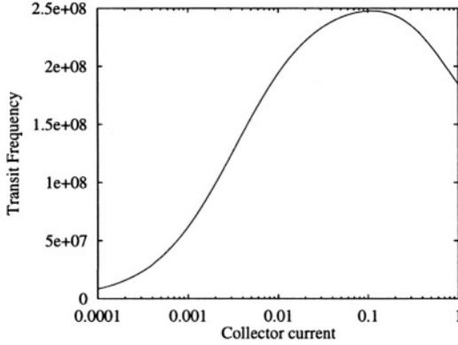
Figure 3.14: The  $f_{T_{eff}}$  of a transistor as functions of its collector current.
