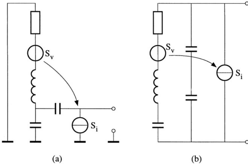
Figure 5.11: Transformation of the noise of the tapped resonator to an equivalent noise current. a) for the actual circuit diagram and b) for the equivalent circuit diagram.
