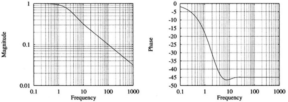
Figure 3.17: The Bode plots of a resistor, used as a one port, with a distributed parasitic capacitance.
