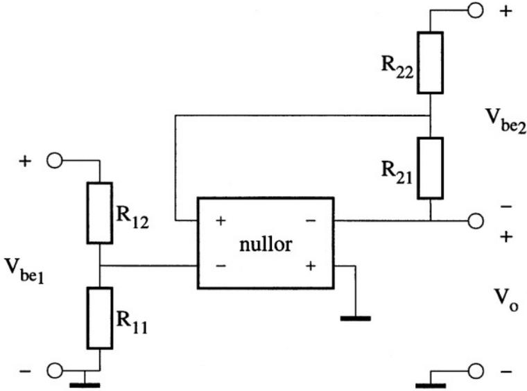
Figure D.4: The combiner for the scaling and addition of the two  $V_{be}$ s
