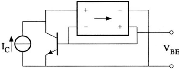
Figure 6.8: An ideal base-emitter voltage generator.
