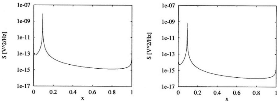
Figure 6.11: The noise power density of a bandgap reference as a function of the collector bias current  $I_{C1}$  with  $I_{S1} = 16$  aA,  $I_{S2}/I_{S1} = 10$  and a)  $I_{max} = 1$   $\mu$ A, b)  $I_{max} = 10$   $\mu$ A [ $x = I_{C1}/I_{MAX}$ ].
