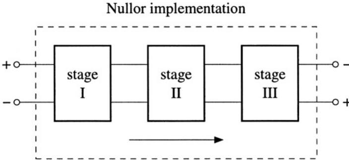
Figure 3.4: A nullor implemented by a cascade of stages.
