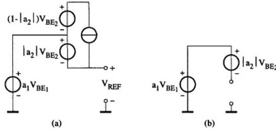
Figure 6.16: Two basic structures for bandgap references in the voltage domain. a) Structure with  $|a_2| \leq 1$  and b) with  $|a_2| > 1$ .
