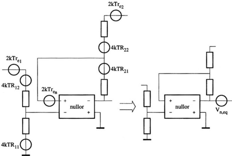
Figure D.6: The relevant noise sources of the bandgap reference
