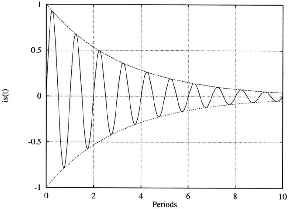
Figure 5.3: The output signal of a resonator as a function of time (normalized to the period time) for  $Q_s = 10$ ; the dotted line indicates the envelope.
