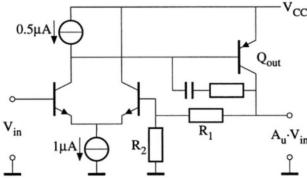
Figure F.5: The negative-feedback voltage amplifier
