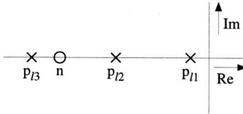
Figure 4.19: The pole-zero plot of pole splitting with  $R_{SP} > \frac{1}{g_{m1}}$ .
