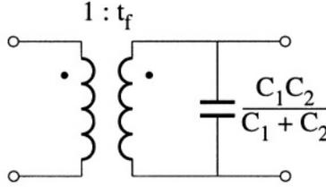
Figure 5.10: The circuit equivalent of capacitive tapping.
