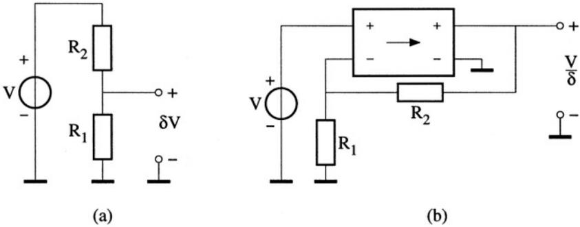
Figure 6.13: Two voltage scalers, a)  $a < 1$  and b)  $a > 1$ .
