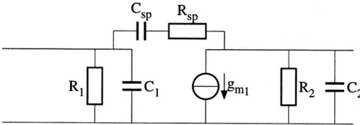
Figure 4.18: The compensation of the right-half plane zero by a resistor.
