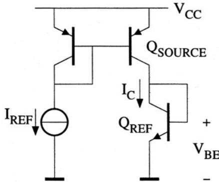
Figure 6.24: A simplified base-emitter voltage generator.
