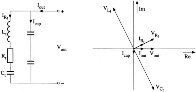
Figure 5.16: The tapped resonator and its vector diagram.
