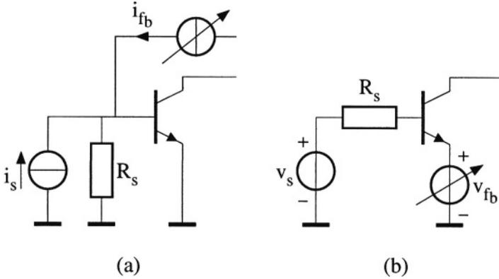
Figure 3.11: Input configurations: a) current input and b) voltage input.
