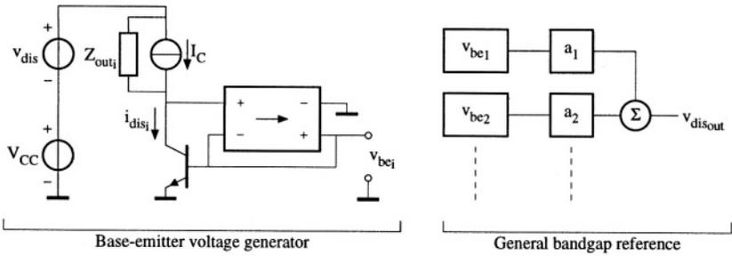
Figure 6.15: An idealized bandgap reference with non-ideal current sources.
