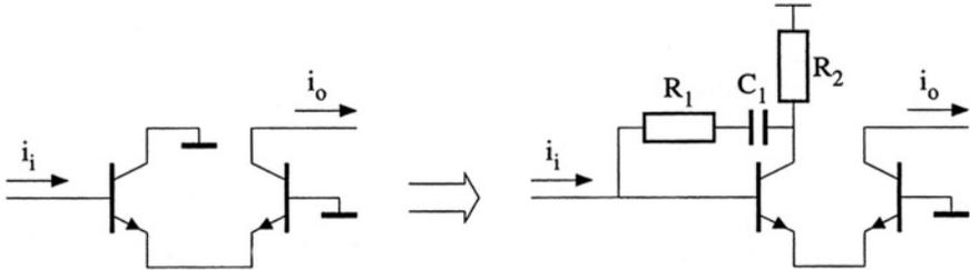
Figure 4.14: Pole-zero cancellation by means of local feedback.
