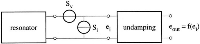
Figure 5.19: Block diagram of the oscillator for studying the noise floor
