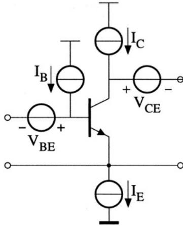
Figure 3.6: A more practical configuration for realizing the bias of a bipolar transistor.
