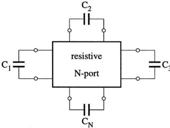
Figure 4.3: The circuit represented by a N-port with N external capacitors.
