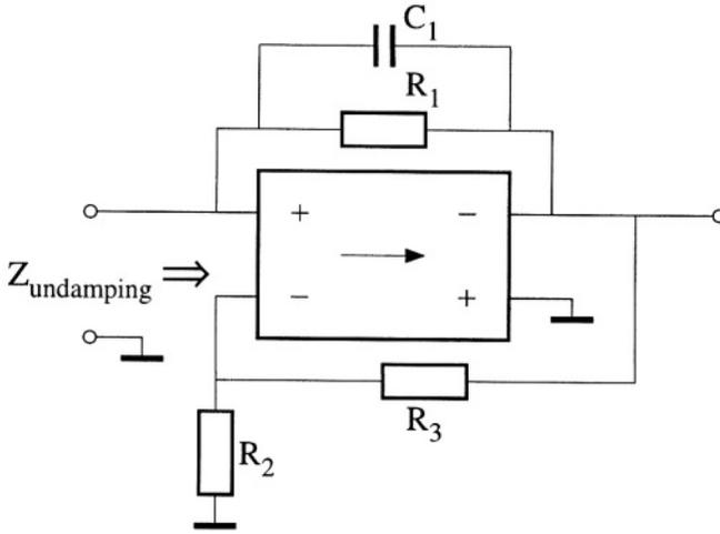
Figure 5.21: An implementation of the negative R and C, combined in one double-loop amplifier.
