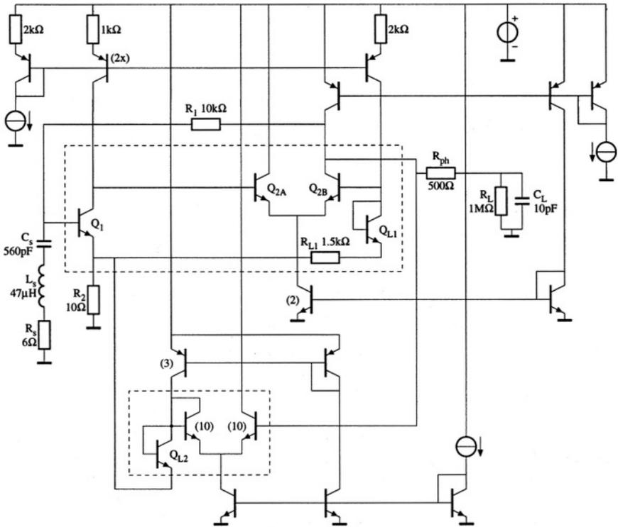
Figure 5.26: The complete schematic of the non-tapped-resonator oscillator.
