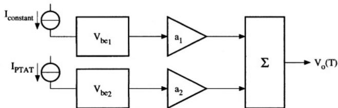
Figure D.1: A linear combination of two base-emitter voltages,  $a_1$  and  $a_2$  are the two scaling factors
