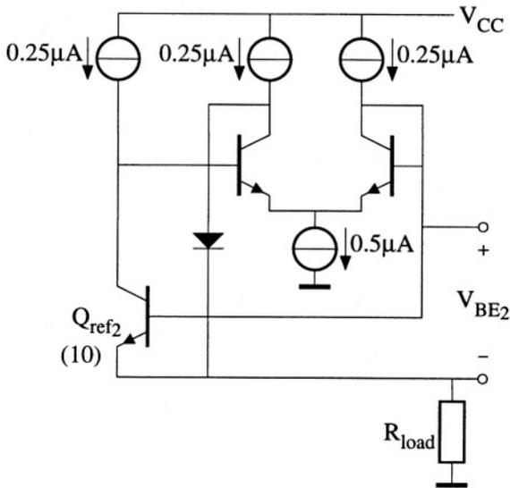
Figure F.4: Implementation of the second base-emitter voltage generator
