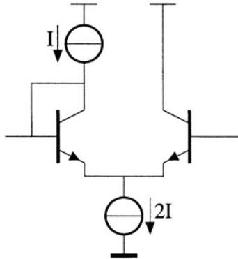
Figure 5.25: The limiter implemented by a differential pair.
