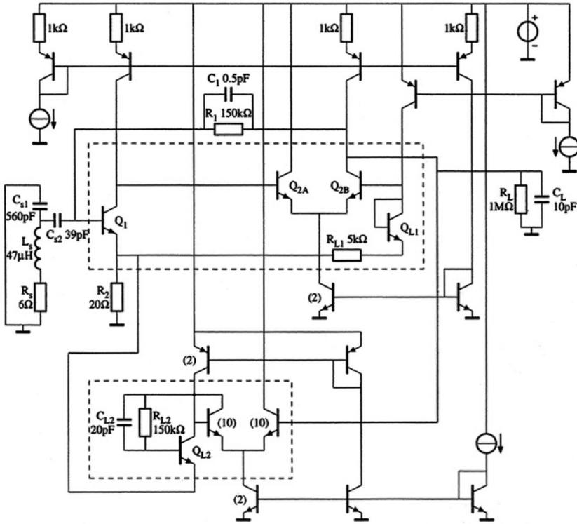
Figure 5.29: The circuit diagram of the tapped-resonator oscillator.
