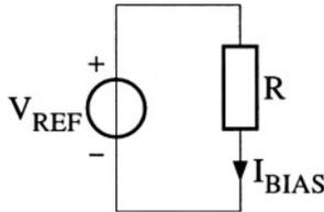
Figure 3.9: The derivation of a bias current from a reference voltage.
