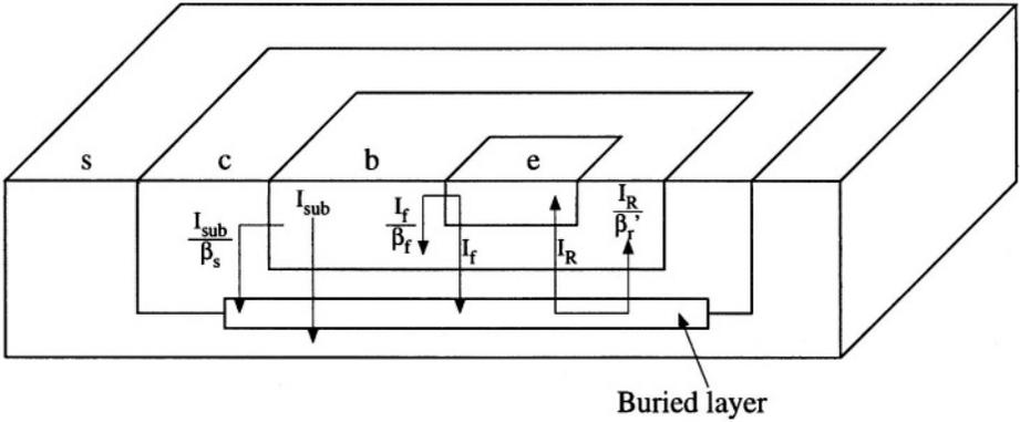
Figure 6.21: A typical structure for a vertical NPN transistor.
