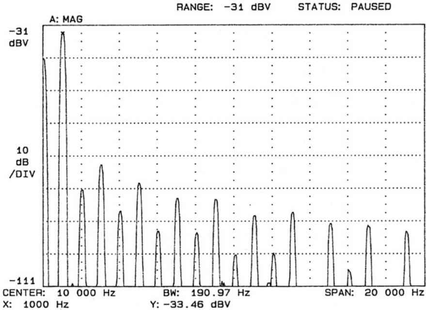
Figure B.12: The spectrum of a 1 mA output current at 1 kHz
