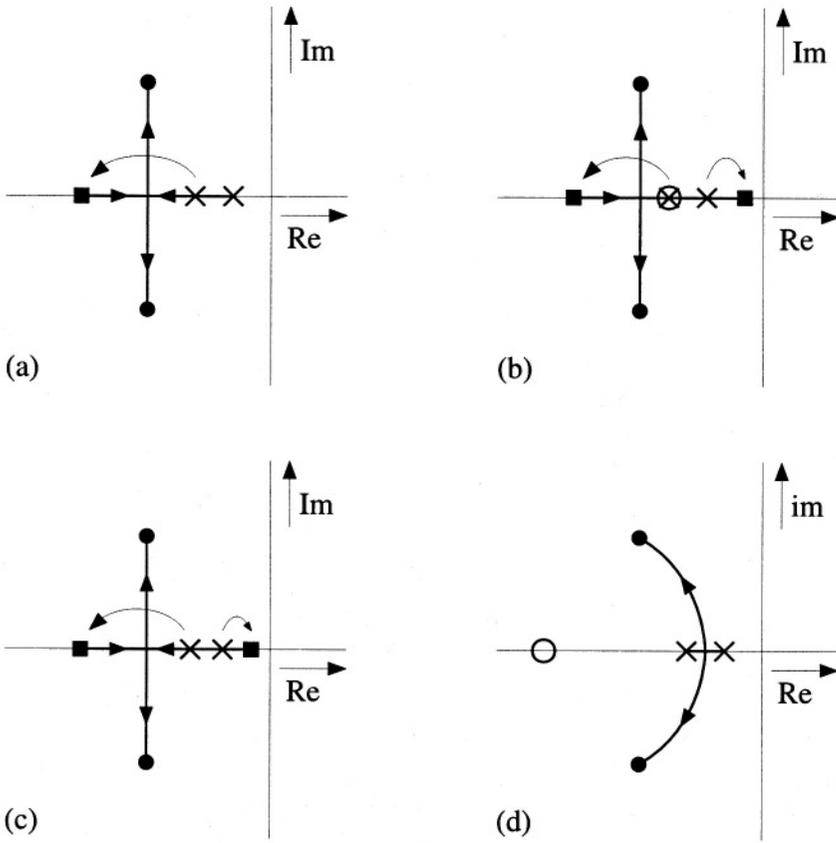
Figure 4.7: Four methods to alter the pole pattern of an amplifier.
