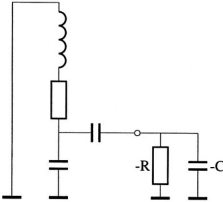
Figure 5.20: Undamping the tapped resonator with both a negative  $R$  and a negative  $C$
