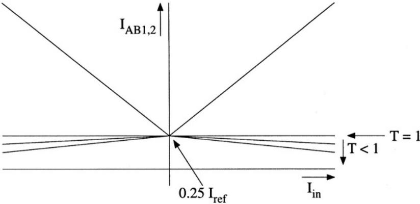
Figure B.7: The currents of the first AB-stage as a function of the input current, with  $T$  as a parameter, when the harmonic-mean control is used (only the asymptotes are depicted)
