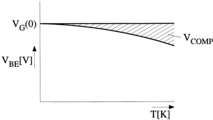
Figure 6.2: The principle realization of a bandgap reference.
