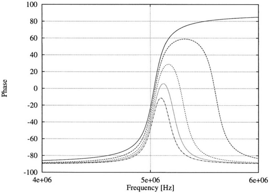
Figure 5.14: The phase shift as a function of the frequency with  $t_f = 1$ ,  $\frac{1}{8}Q_s$ ,  $\frac{1}{3}Q_s$ ,  $\frac{1}{2}Q_s$ ,  $\frac{2}{3}Q_s$  corresponding to the functions ordered from the upper one to the lower one.
