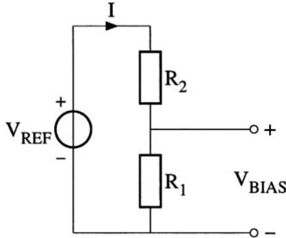
Figure 3.8: The realization of a bias voltage by dividing a larger voltage.
