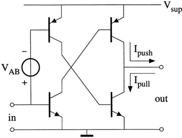
Figure B.3: The two last stages are chosen to be class-AB biased
