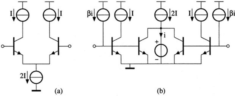
Figure 3.7: Realizing a balanced CE stage. a) In the voltage domain and b) in the current domain.
