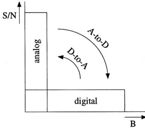
Figure 2.11: Digital and analog signals in the S/N-versus-B plane.
