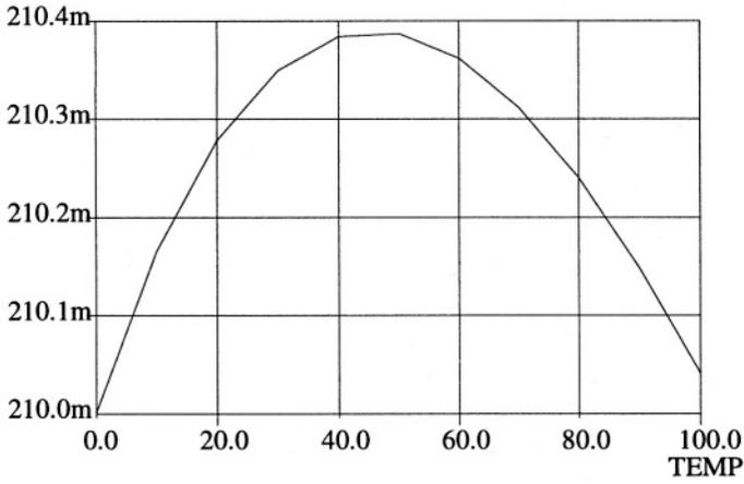
Figure F.7: Simulation of the temperature behavior of the total bandgap reference
