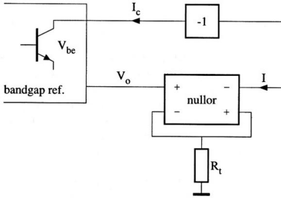
Figure D.7: Bias loop for the biasing of the ( $V_{be}$ ) transistor with a constant collector current ( $\theta = 0$ )
