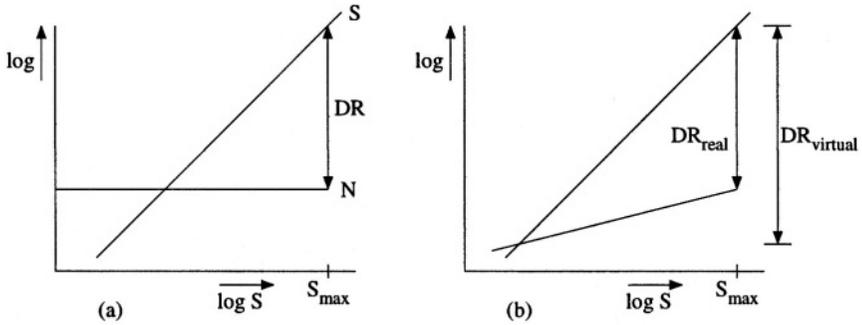
Figure 2.10: The influence of automatic gain control. a) The system without and b) the system with automatic gain control.
