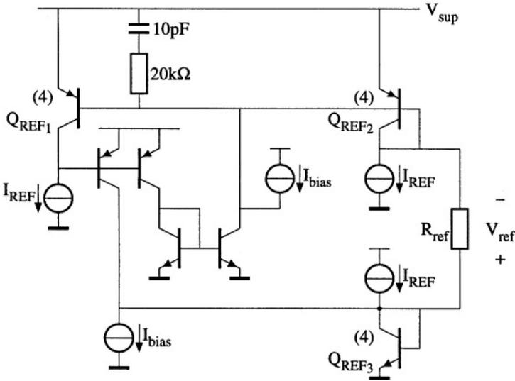
Figure B.5: The implementation of the nullor forcing  $I_{REF}$  through  $Q_1$
