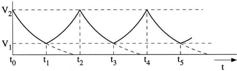
Figure 2.15: An oscillator realized by switching between two poles.
