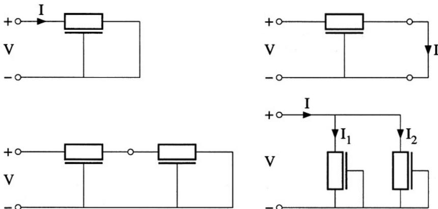
Figure 3.16: The four ways in which resistors can be used.
