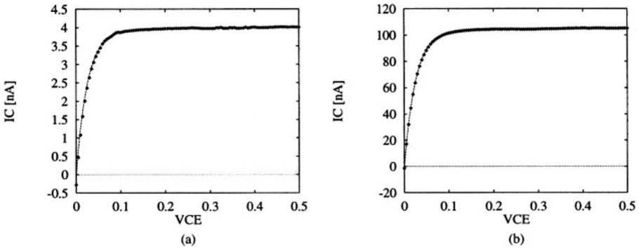
Figure 6.23: The calculated (drawn line) and the measured (dotted line) saturation behavior for a) a transistor with a relatively small emitter ( $6 \times 6 \mu\text{m}^2$ ) and b) a relatively large transistor ( $30 \times 30 \mu\text{m}^2$ )
