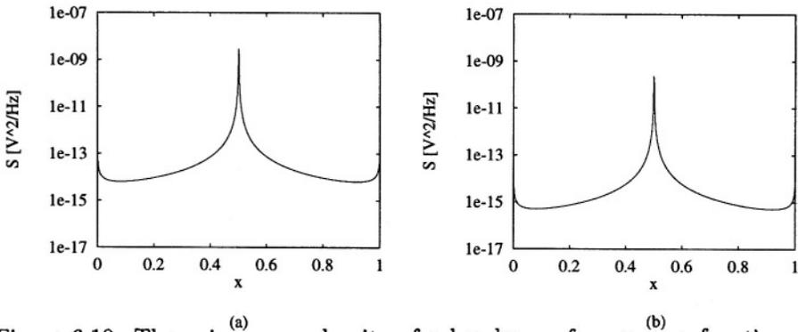
Figure 6.10: The noise power density of a bandgap reference as a function of the collector bias current  $I_{C1}$  with  $I_{S1} = 16$  aA,  $I_{S2}/I_{S1} = 1$  and a)  $I_{max} = 1$   $\mu$ A, b)  $I_{max} = 10$   $\mu$ A [ $x = I_{C1}/I_{MAX}$ ].
