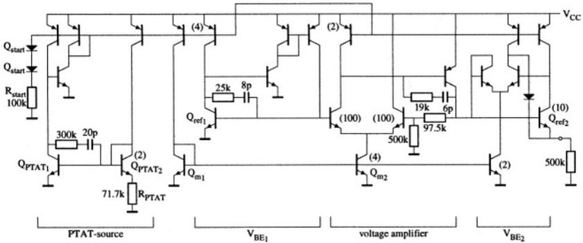
Figure F.6: The total circuit of the bandgap reference
