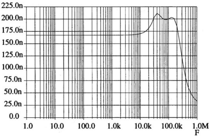
Figure F.8: Simulation of the noise at the output of the total bandgap reference
