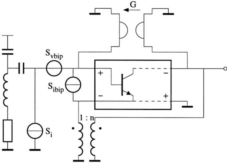
Figure 5.12: The oscillator using a tapped resonator with a bipolar transistor as the input of the nullor implementation.
