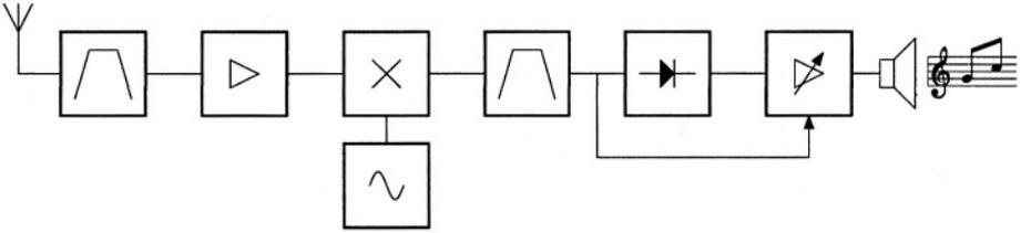
Figure 2.1: A block schematic of a radio receiver.
