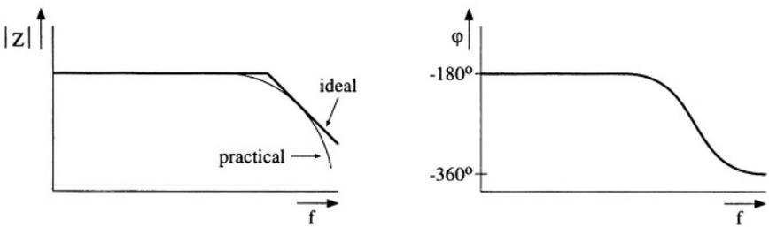
Figure 5.22: The bandwidth of the undamping impedance.
