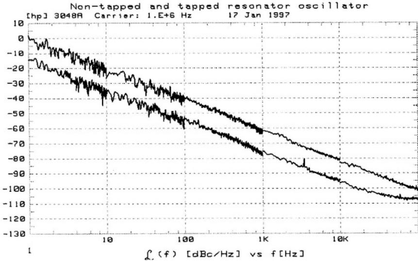
Figure 5.30: The measured  $\mathcal{L}(\Delta\omega)$  of the two oscillators. The upper and lower graph corresponds to the non-tapped and tapped-resonator oscillator, respectively.
