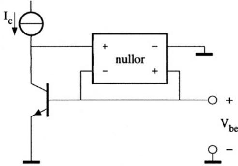
Figure D.2: The base-emitter voltage generator with a nullor for the biasing
