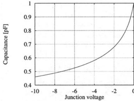
Figure 3.10: The capacitance of a reverse-biased junction as a function of the bias voltage, with  $M = 0.28$ ,  $V_J = 0.67$  V and  $C_{J0} = 1$  pF.
