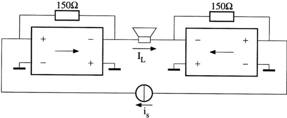
Figure B.2: The balanced transimpedance output amplifier
