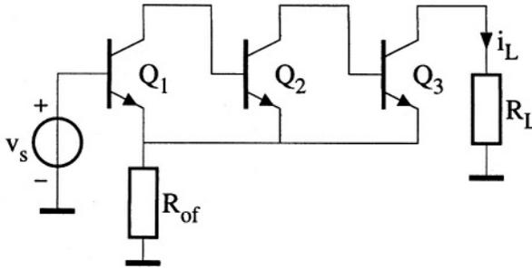
Figure 4.1: A three-stage transconductance amplifier.
