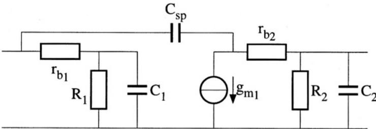
Figure 4.17: Pole splitting in a circuit.
