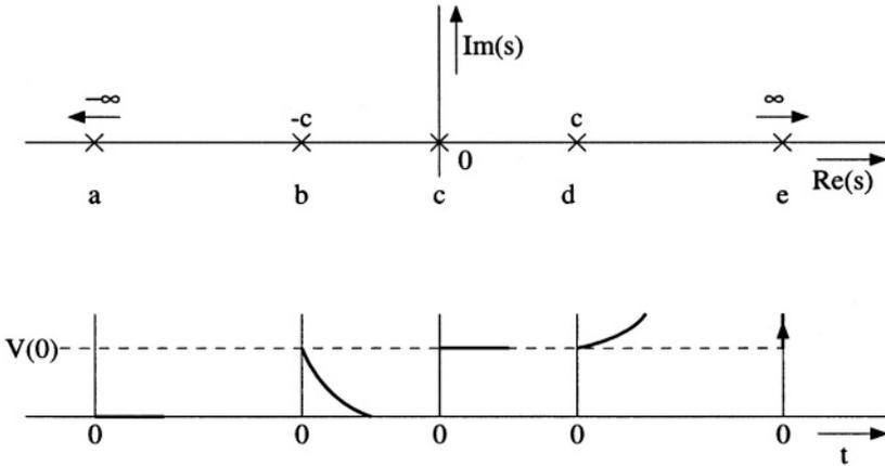
Figure 2.14: The solutions of the first-order differential equation in the Laplace domain and time domain.
