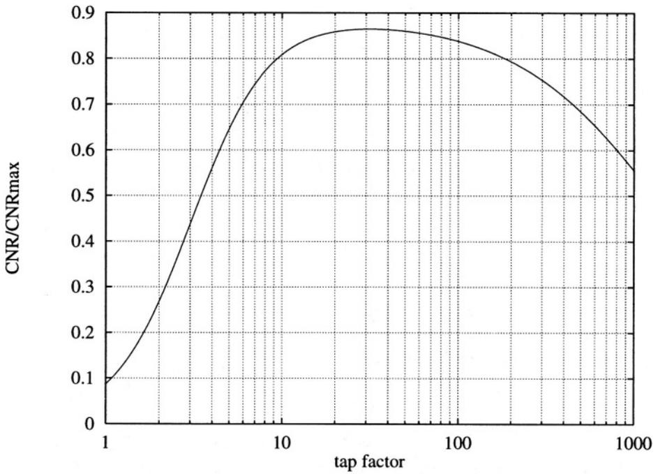
Figure 5.27: The CNR normalized to the maximum attainable CNR as a function of the tap factor.
