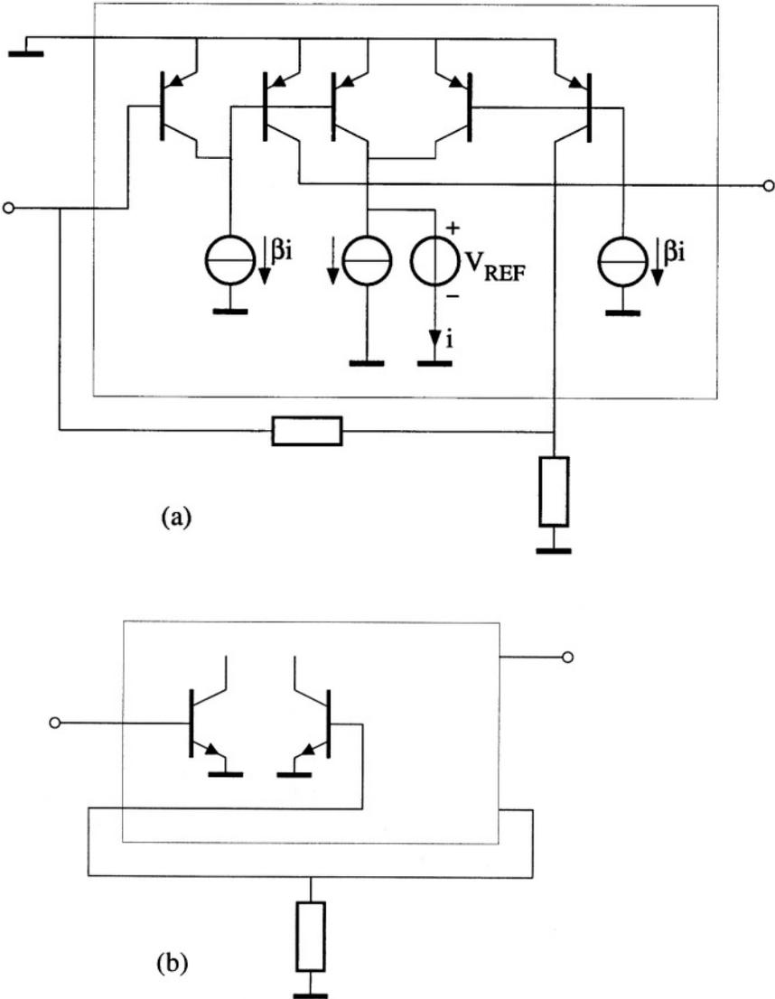
Figure A.2: Using a balanced stage in the current domain for a) a current amplifier and b) a voltage-to-current amplifier.
