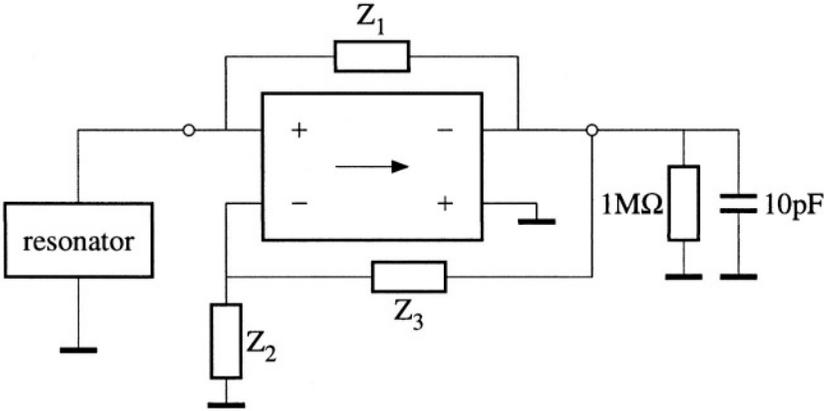
Figure 5.23: The basic configuration of the active part.
