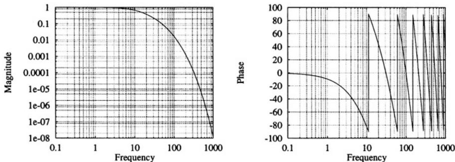
Figure 3.18: The bode plots of a resistor used as a two port.
