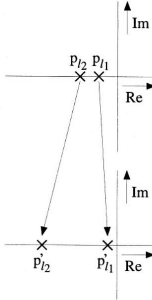
Figure 4.16: The principle of pole splitting.
