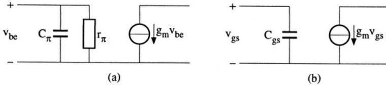
Figure 4.5: The relevant model for active devices. a) The bipolar transistor and b) the field-effect transistor.
