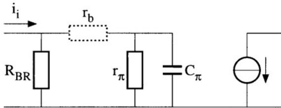
Figure 4.9: A passive implementation of resistive broadbanding.
