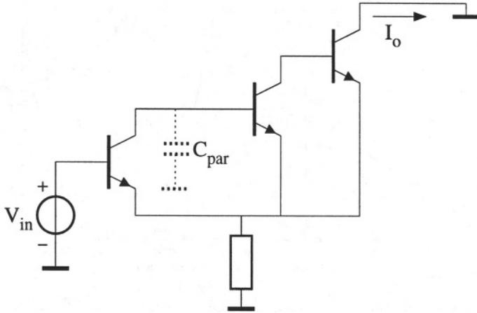
Figure 3.13: A three-stage transconductance amplifier.
