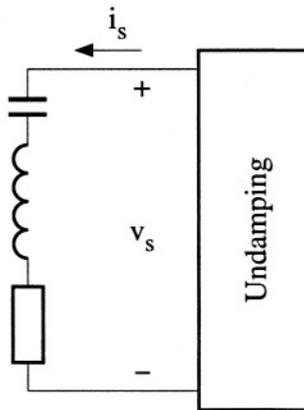
Figure 5.4: The series resonators with its undamping.
