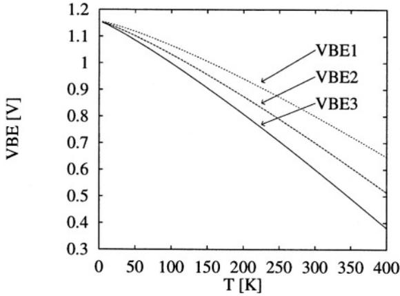
Figure 6.1: The base-emitter voltage as a function of the temperature for several values of  $V_{BE}$ ,  $V_{BE1} > V_{BE2} > V_{BE3}$ .
