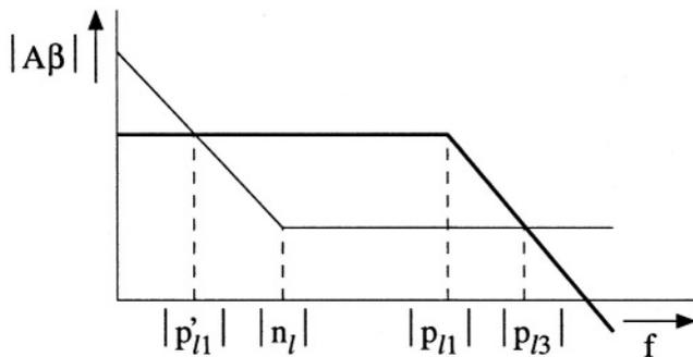
Figure 4.15: The influence of a local current feedback on the transfer of a differential pair.
