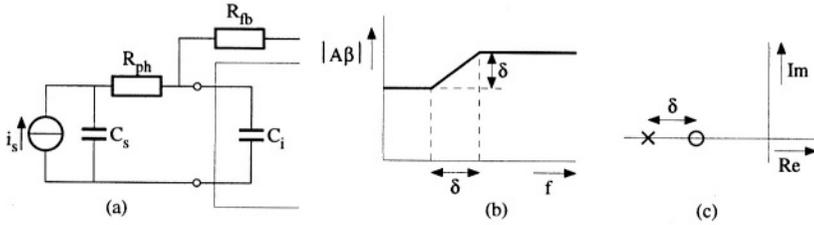
Figure 4.20: An example of the effectiveness of a phantom zero. a) The realization of a phantom zero by  $R_{ph}$ , b) the influence on the magnitude of the loop gain and c) the pole-zero plot.
