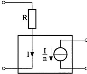
Figure 3.20: An active realization of a high resistance.
