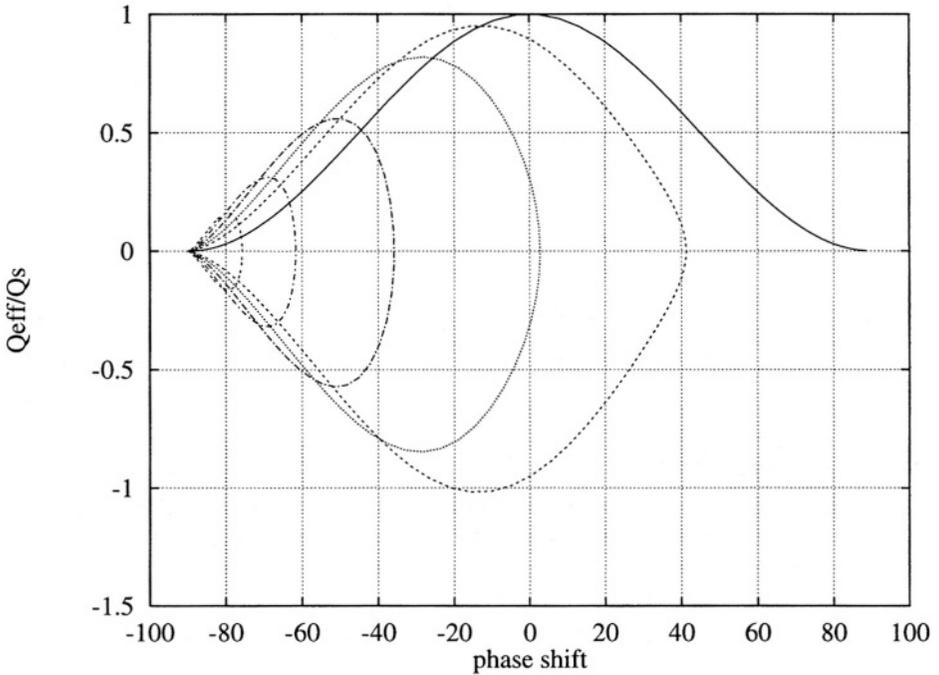
Figure 5.18: The relative change in the quality factor as a function of the phase shift with the tap factor as a parameter. For the functions the tap factor equals, from the right to the left, respectively,  $t_f = 1$ ,  $\frac{1}{4}Q_s$ ,  $\frac{1}{2}Q_s$ ,  $Q_s$ ,  $2Q_s$  and  $4Q_s$ .
