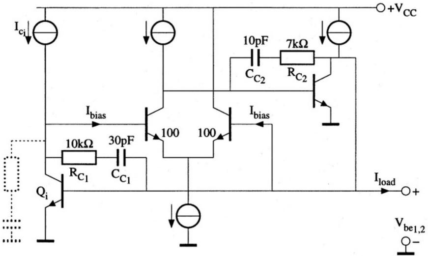
Figure D.3: The base-emitter voltage generator with a circuit implementation for the nullor
