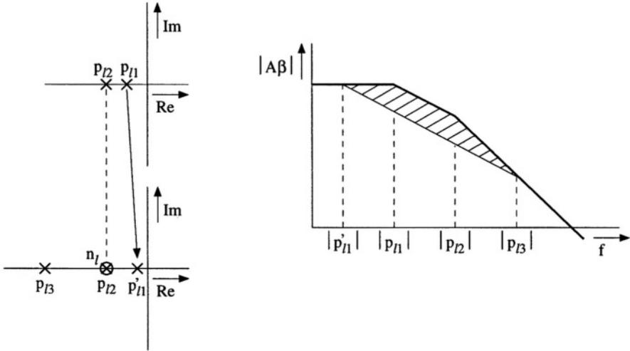
Figure 4.12: The principle of pole-zero cancellation.
