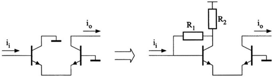
Figure 4.10: Resistive broadbanding by means of local feedback.
