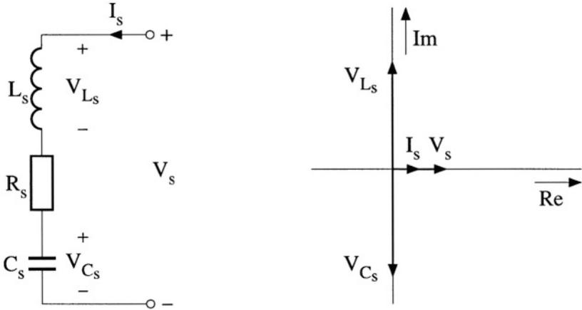
Figure 5.15: The non-tapped resonator and its vector diagram.
