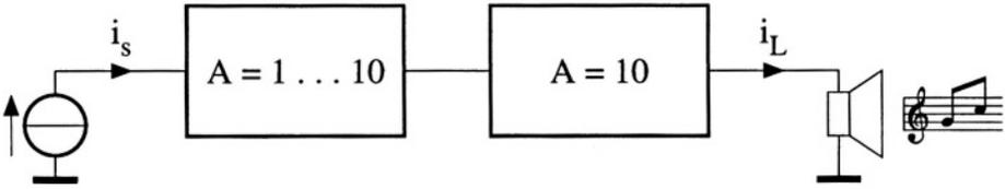
Figure B.1: The block diagram of the complete controllable output amplifier
