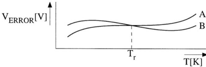
Figure 6.3: Two general ways of specifying the temperature dependency of a bandgap reference. A: maximum flat and B: lowest mean dependency.
