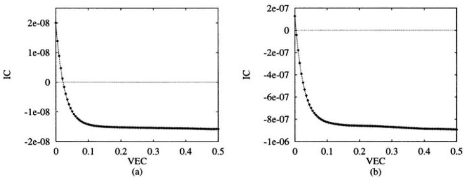
Figure 6.19: Plot of the calculated (solid line) and measured (dotted line) saturation behavior of a) the small and b) the large lateral PNP transistor.
