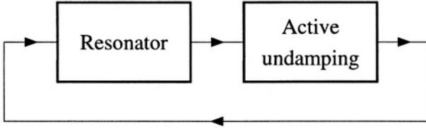
Figure 5.1: The compensation of the losses in a resonator by means of an active undamping.
