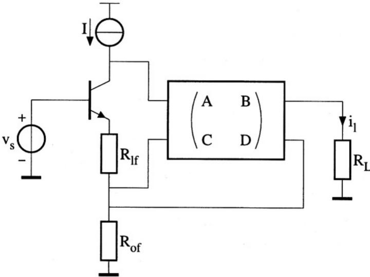
Figure 4.2: Reduction of the distortion of the input stage by means of local feedback.
