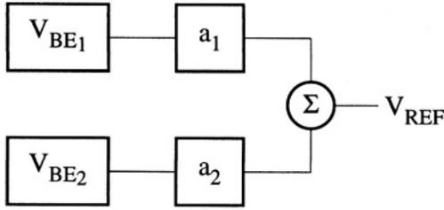
Figure 6.7: A general block diagram of a first and second-order compensated bandgap reference.
