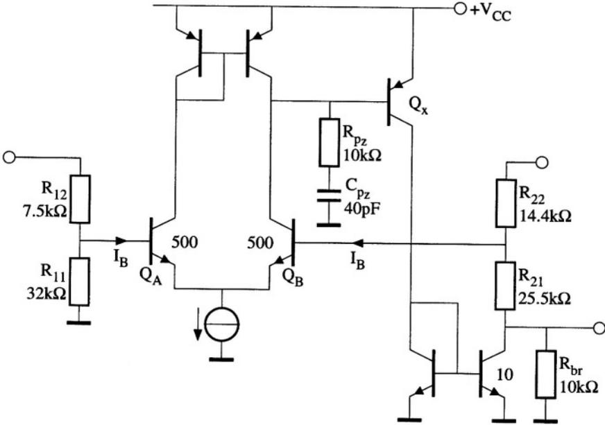
Figure D.5: The combiner with a circuit implementation for the nullor
