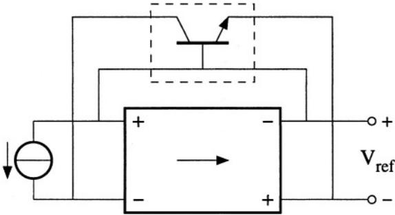
Figure 2.13: An accurate relation between collector current and base-emitter voltage by means of negative feedback.
