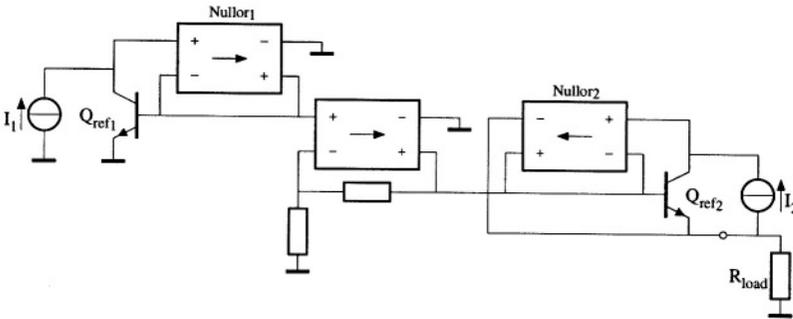
Figure F.2: Implementation of the bandgap reference at nullor level
