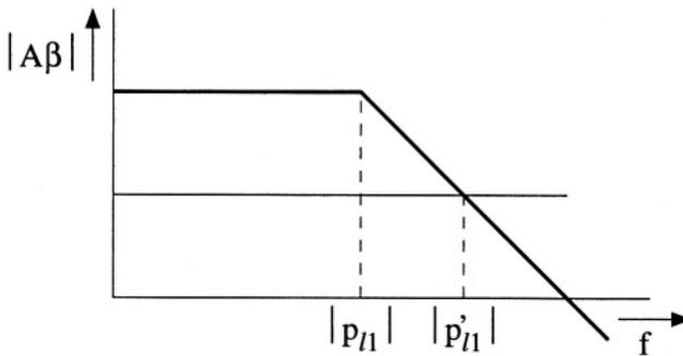
Figure 4.11: The influence of resistive broadbanding, by means of a local loop, on the bode plot.
