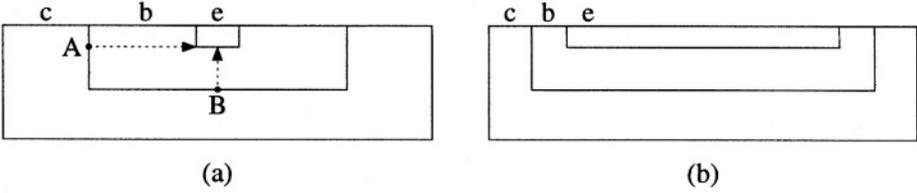
Figure 6.22: The influence of the layout on the reverse current-gain factor of a vertical transistor, a) a transistor with a relatively tiny emitter and b) a transistor with a relatively large emitter.
