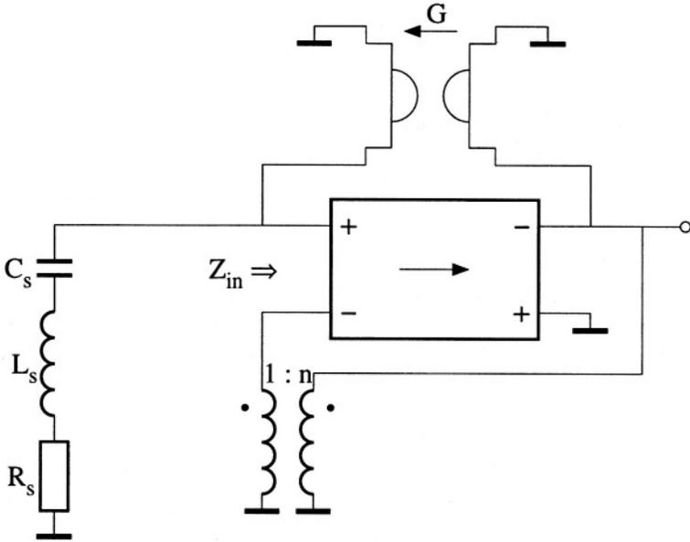
Figure 5.7: A series resonator undamped by means of a negative impedance realized by means of a nullor with a double-loop feedback.
