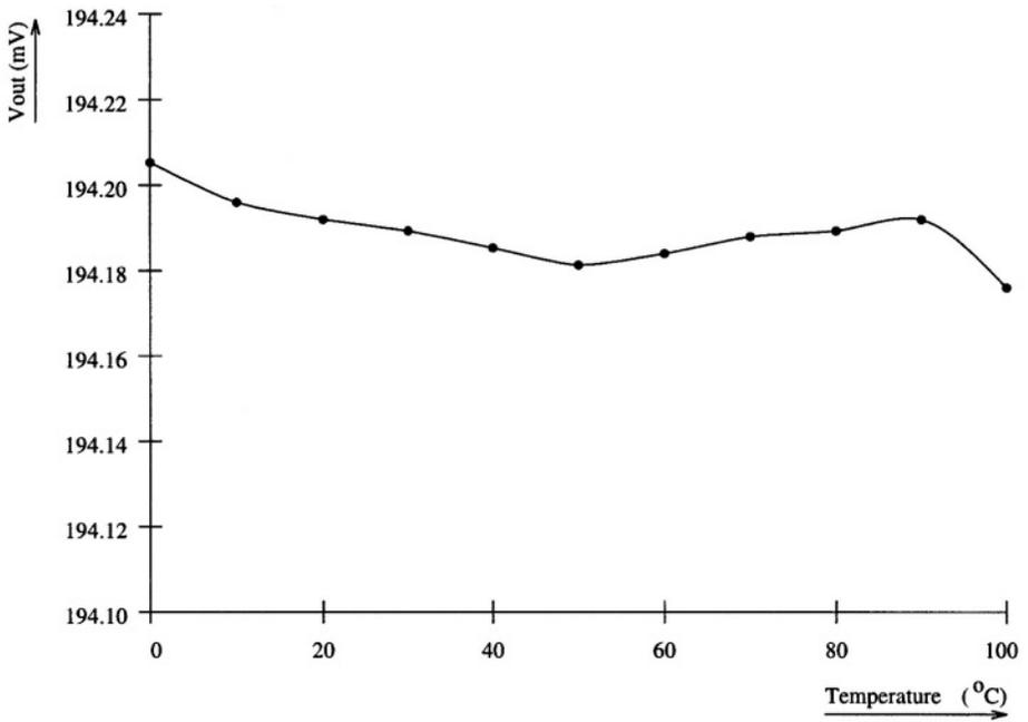
Figure D.13: The measured output voltage as a function of the temperature
