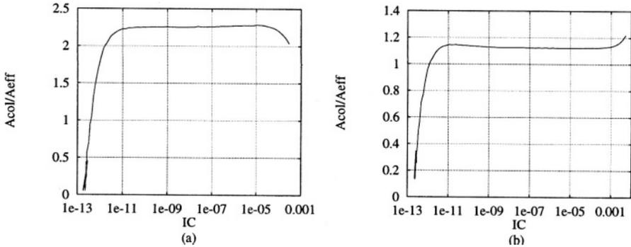
Figure 6.20:  $A_{col}/A_{eff}$  measured as a function of the collector current of the non-saturated transistor for a) the small PNP transistors and b) for the large one.
