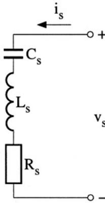
Figure 5.2: A series resonator.
