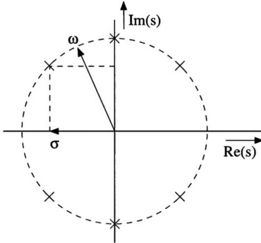
Figure 2.16: The poles in the  $s$ -plane for the three different solutions having complex conjugated poles.
