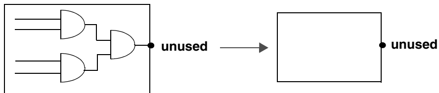
Figure 6-5 Minimizing Logic Driving an Unconnected Output Port
