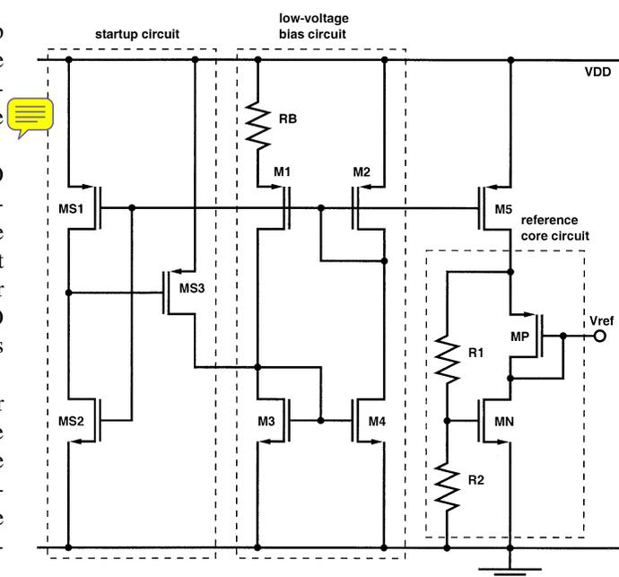
Fig. 10. CMOS voltage reference.
