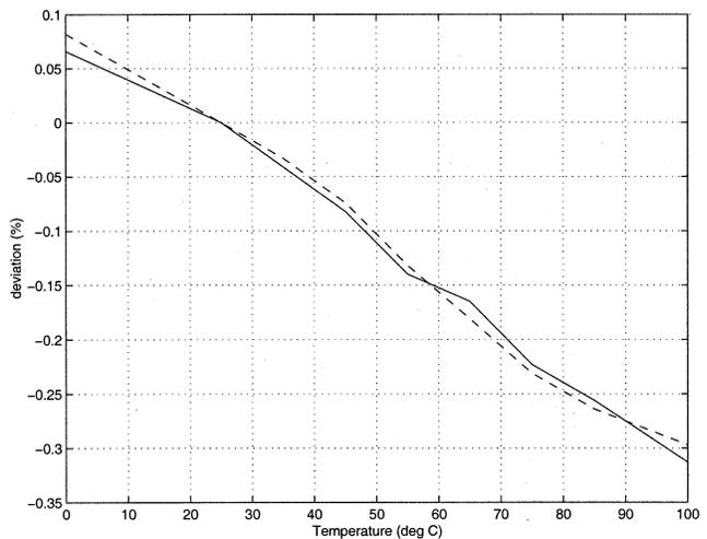
Fig. 13. Measured temperature dependence at  $V_{IN} = 1.5 \text{ V}$  (solid line:  $I_{OUT} = 100 \text{ mA}$ ; dashed line:  $I_{OUT} = 0$ ).
