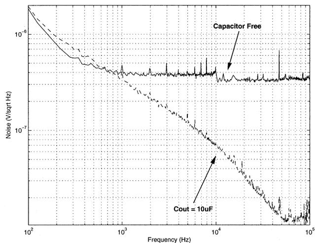
Fig. 14. Measured output spectral noise density at  $V_{IN} = 1.5 \text{ V}$  and  $I_{OUT} = 100 \text{ mA}$ .
