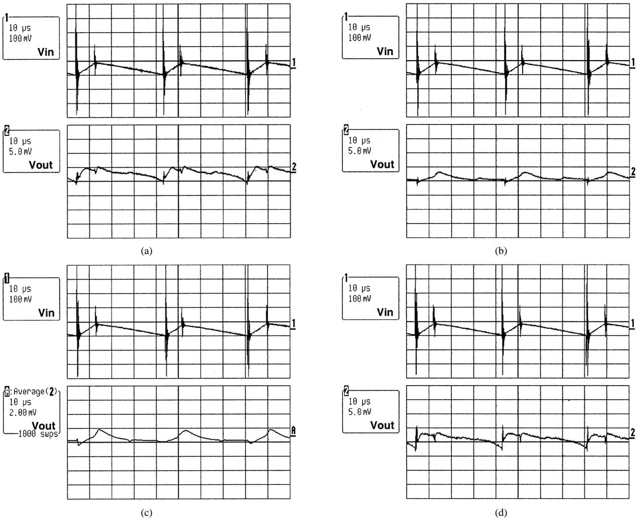
Fig. 18. Measured ripple rejection. (a)  $C_{OUT} = 10$   $\mu$ F, ESR = 1  $\Omega$ , and  $I_{OUT} = 0$ . (b)  $C_{OUT} = 10$   $\mu$ F, ESR = 1  $\Omega$ , and  $I_{OUT} = 100$  mA. (c)  $C_{OUT} = 0$  and  $I_{OUT} = 1$  mA. (d)  $C_{OUT} = 0$  and  $I_{OUT} = 100$  mA.
