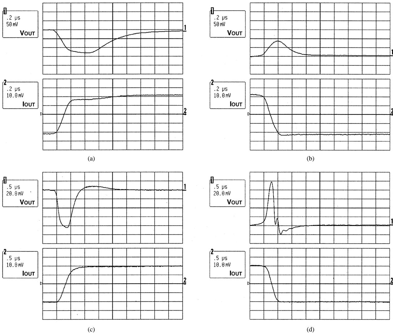
Fig. 15. Load transient responses at  $V_{IN} = 1.5$  V (a) 0 to 100 mA with  $C_{OUT} = 10 \mu F$  and  $ESR = 1 \Omega$  (b) 100 to 0 mA with  $C_{OUT} = 10 \mu F$  and  $ESR = 1 \Omega$  (c) 10 to 100 mA with  $C_{OUT} = 0$  (d) 100 to 10 mA with  $C_{OUT} = 0$ .
