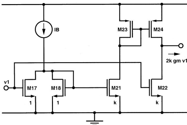
Fig. 9. Transconductance-boosting circuitry.
