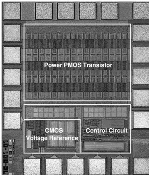
Fig. 11. Micrograph of the proposed CMOS LDO.
