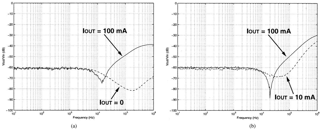
Fig. 17. Measured PSRR at  $V_{IN} = 1.5$  V. (a)  $C_{OUT} = 10$   $\mu$ F and ESR = 1  $\Omega$ . (b)  $C_{OUT} = 0$ .
