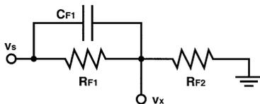
Fig. 5. Feedback-resistive network with first-order high-pass characteristic.
