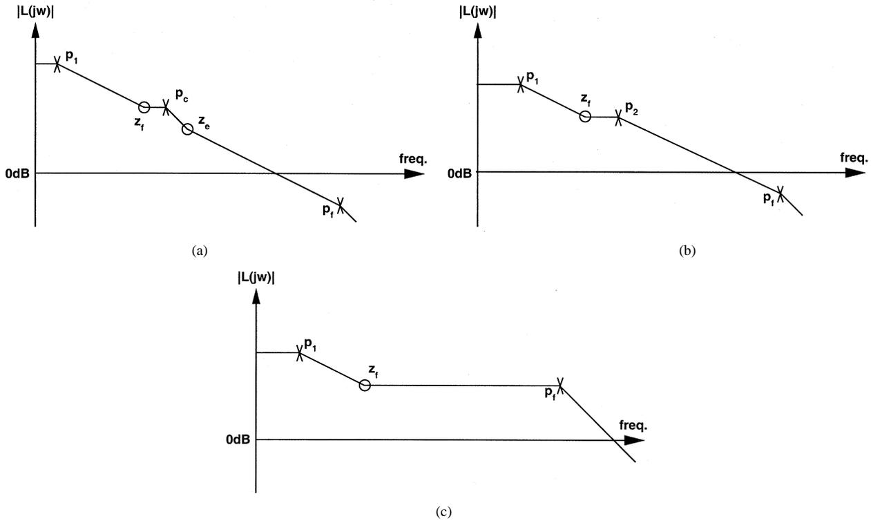
Fig. 6. Loop gain (magnitude plot only and not in scale) of the proposed LDO structure. (a)  $C_{OUT} \neq 0$  and  $I_{OUT} = 0$ . (b)  $C_{OUT} \neq 0$  and  $I_{OUT} \neq 0$ . (c)  $C_{OUT} = 0$  and  $I_{OUT} \neq 0$ .
