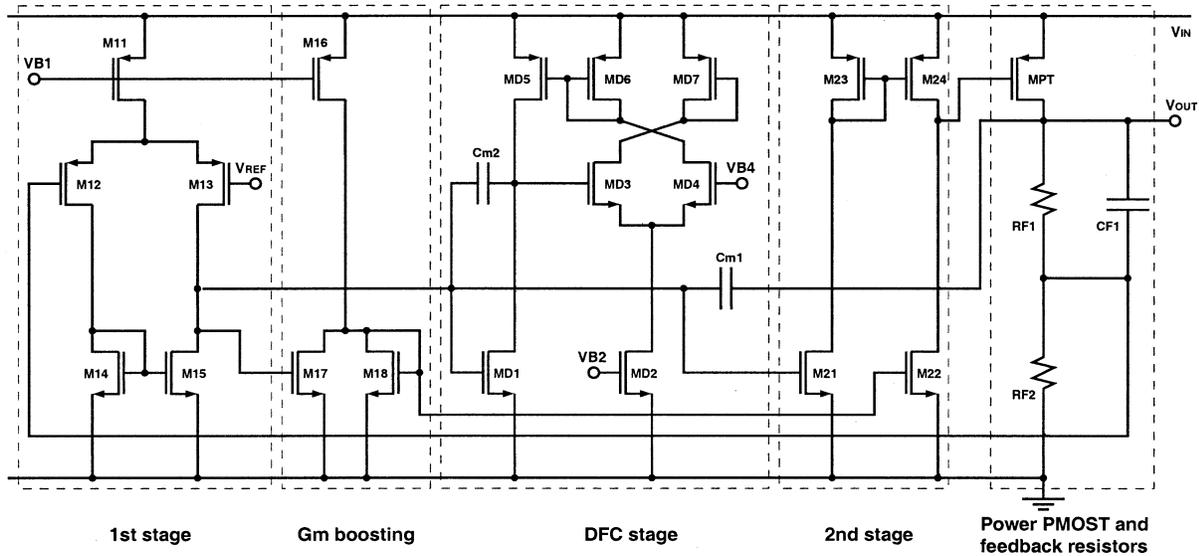
Fig. 4. Complete schematic of the proposed LDO.
