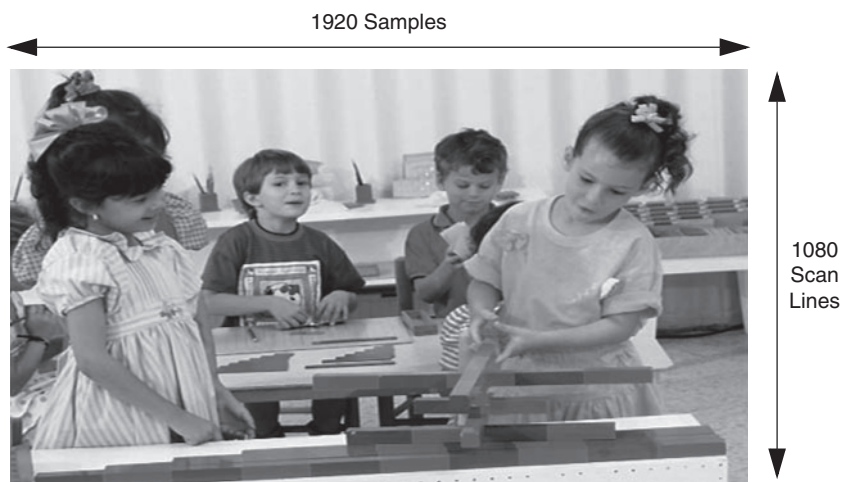
FIGURE 5.15 Scaling 4:3 Content for a 16:9 Display: “Wide” mode. Entire picture linearly scaled horizontally to fill 16:9 display, resulting in distorted picture unless used with anamorphic content.
