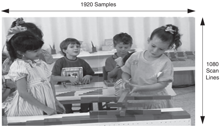
FIGURE 5.17 Scaling 4:3 Content for a 16:9 Display: “Panorama” mode. Left and right 25% edges of picture are nonlinearly scaled horizontally to fill 16:9 display, distorted picture on left and right sides.
