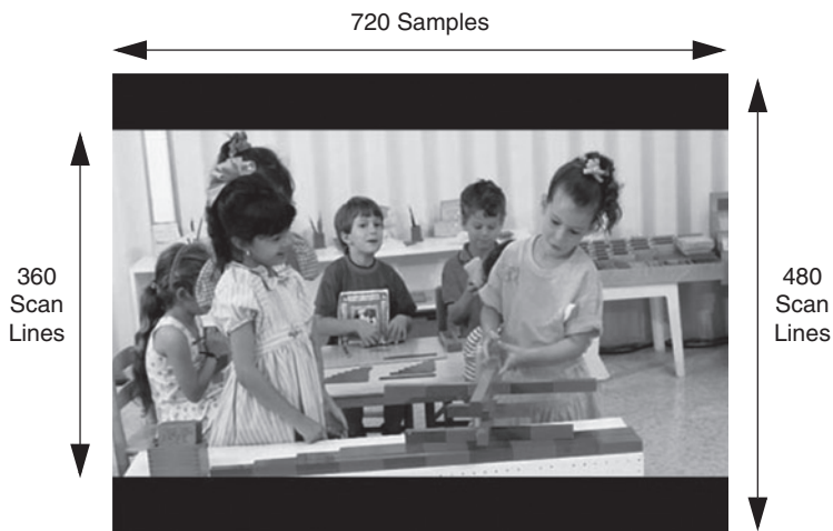
FIGURE 5.11 Scaling 16:9 Content for a 4:3 Display: “Letterbox” mode. Entire 16:9 program visible, with black bars at top and bottom of display.
