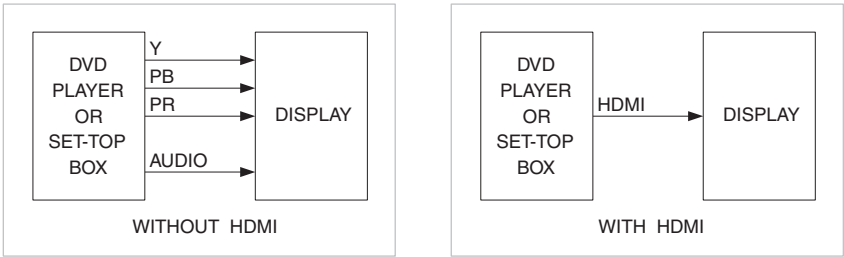
FIGURE 4.39 Using HDMI Eliminates Confusing Cable Connections for Consumers.
