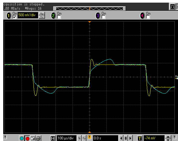
Fig. 77. Settling time measurements with and without the auxiliary loop for speed-up
