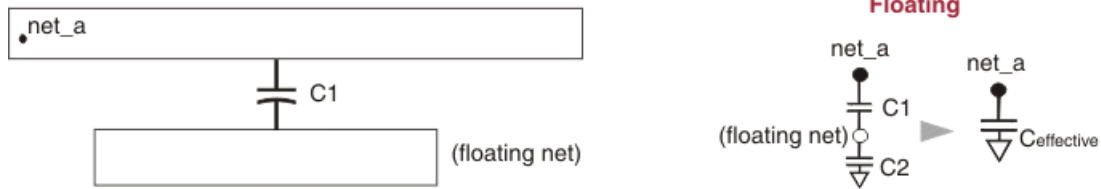
Figure 9-2. Floating-Net Coupling Floating Example
