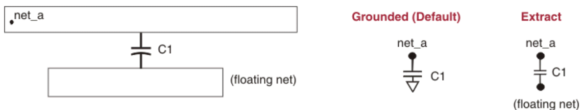
Figure 9-3. Floating-Net Coupling Extraction Example
