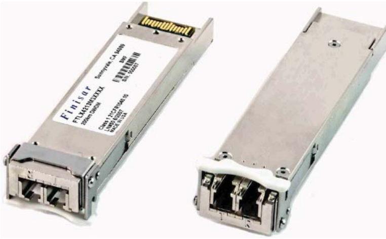
Figure 1.2 Two 10-Gb/s transceivers in small form factor packages following the XFP specification (7.8 cm × 2.2 cm × 1.3 cm). Two fibers are plugged in from the front of the package (LC connectors). Source: Reprinted by permission from Finisar Corporation.
