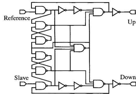
Fig. 1. Conventional phase frequency detector (conPFD) from [2].
