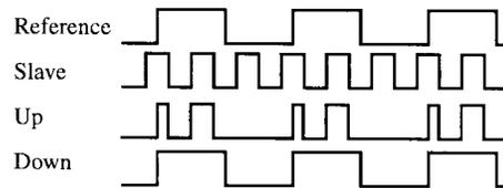
Fig. 10. Waveforms for the case when the slave has a higher frequency than the reference signal. The down signal has higher duty cycle than the up signal.
