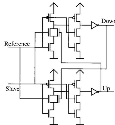
Fig. 2. Precharge type phase frequency detector (ptPFD) from [3].
