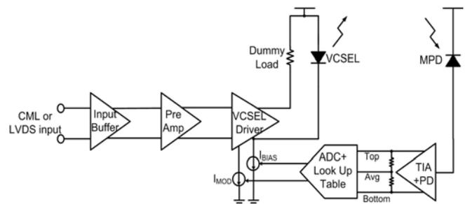
Fig. 2. Block diagram of a single-channel VCSEL driver.
