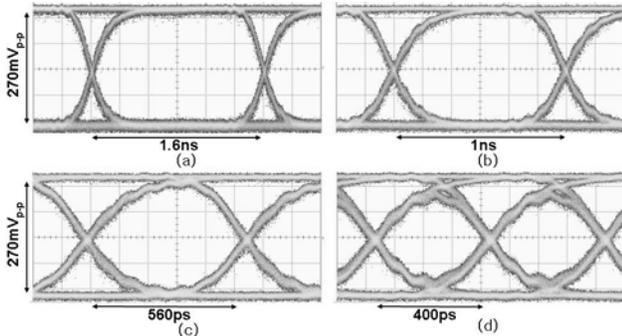
Fig. 10. Measured eye-diagrams of a single-channel CG TIA for  $2^{31}-1$  PRBS at the different data rates of : (a) 622Mb/s, (b) 1Gb/s, (c) 1.8Gb/s, and (d) 2.5Gb/s.
