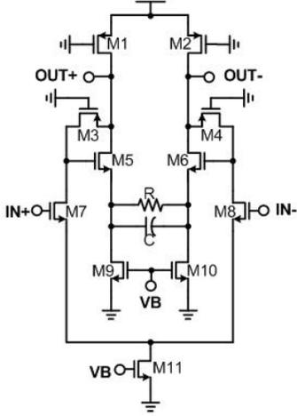
Fig. 3. Schematic diagram of the preamplifier with capacitive degeneration.
