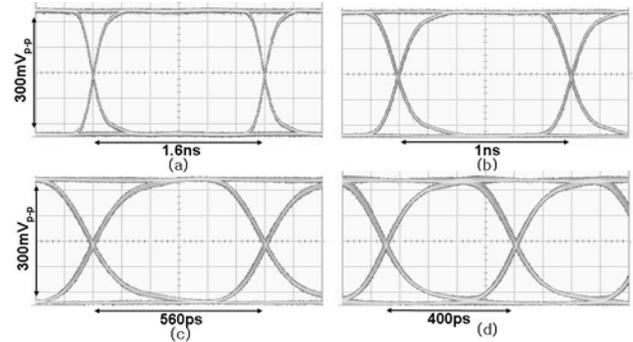
Fig. 8. Measured eye-diagrams of a single-channel VCSEL driver for 2<sup>31</sup>-1 PRBS at different data rates of : (a) 622Mb/s, (b) 1Gb/s, (c) 1.8Gb/s, and (d) 2.5Gb/s.
