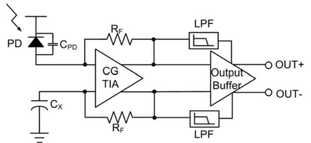
Fig. 4. Block diagram of a single-channel receiver.
