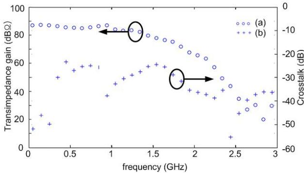
Fig. 11. (a) Measured frequency response of the CG TIA, and (b) measured crosstalk between TX and RX.
