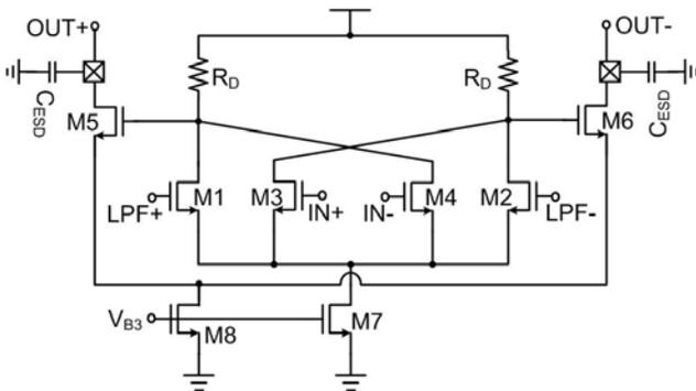
Fig. 6. Schematic diagram of the DC-balanced output buffer.
