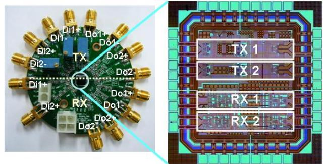
Fig. 7. Chip microphotograph of the dual-channel optical transceiver array and its evaluation board.
