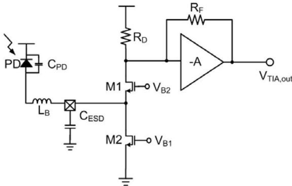
Fig. 5. Simplified schematic diagram of the CG input stage.
