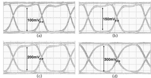
Fig. 9. Measured eye-diagrams of 2.5Gb/s VCSEL driver with AMC control loops turned on with modulation currents of : (a) 4mA<sub>pp</sub>, (b) 6mA<sub>pp</sub>, (c) 8mA<sub>pp</sub>, and (d) 12mA<sub>pp</sub>.
