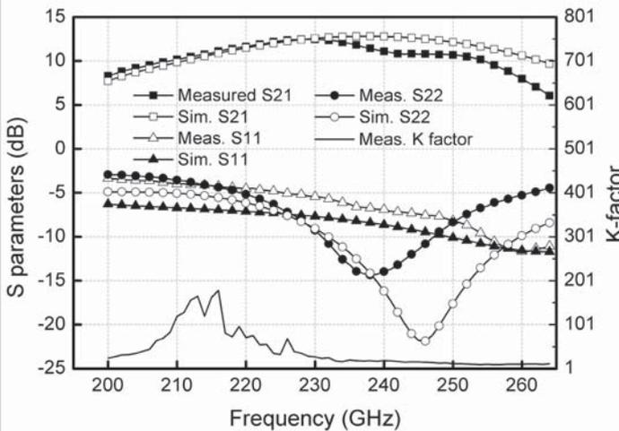
Figure 4.5.3: Simulated and measured S-parameters for the 4-way PA.
