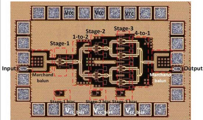
Figure 4.5.7: Die micrograph of the 4-way PA (Die area=0.83mm<sup>2</sup>).
