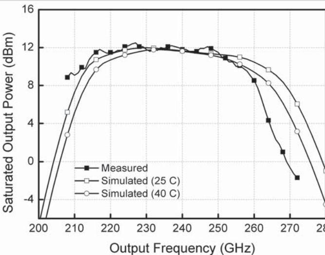
Figure 4.5.5: Simulated and measured saturated output power across frequency.
