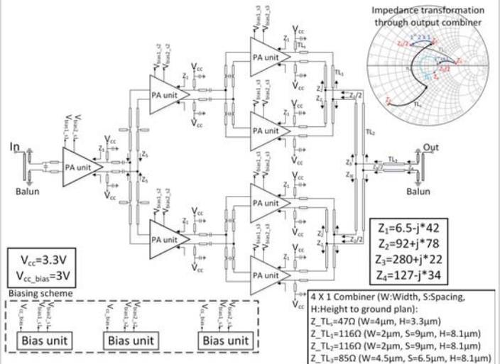
Figure 4.5.2: Block diagram of the 4-way power-combined PA.
