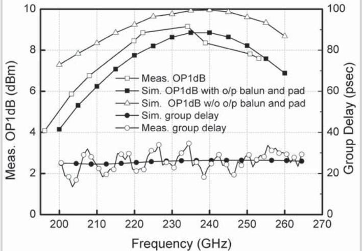
Figure 4.5.4: Simulated and measured OP1dB compression point and group delay variations across frequency.
