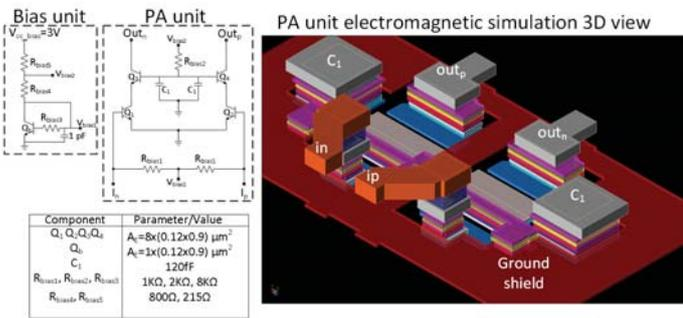
Figure 4.5.1: Schematic of the PA unit, the bias circuit, and the electromagnetic simulation view for the transistor core.
