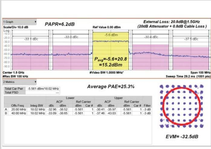
Figure 4.2.5: Measured DPA spectrum and constellation of 20MHz 64-QAM LTE signal.
