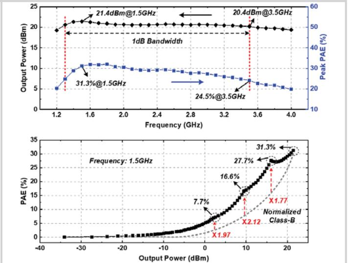
Figure 4.2.4: Measured CW results of output power, PAE (PAE=Pout/Pdc\_total), and the frequency response.
