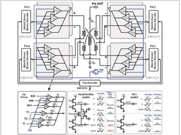
Figure 4.2.2: Detailed schematic of the proposed switched-transformer digital PA.
