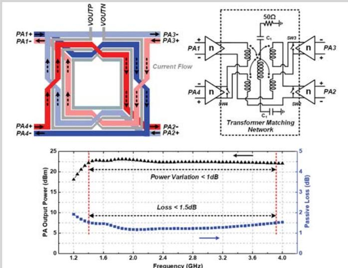
Figure 4.2.3: Implementation of the proposed switched-transformer-based matching network and its simulation results.
