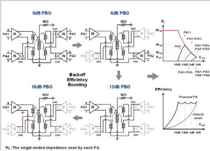
Figure 4.2.1: Operating principles of the proposed switched-transformer digital PA.
