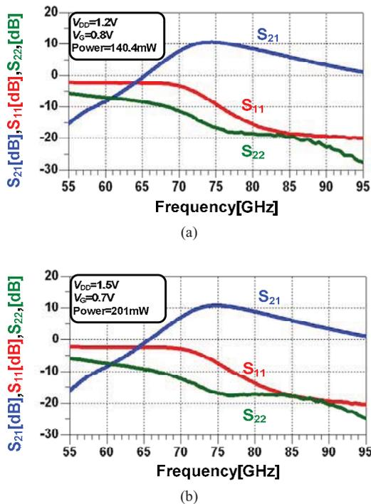
Fig. 5. Measured S-parameters of the power amplifier operating at (a) 1.2 V and (b) 1.5 V supply.
