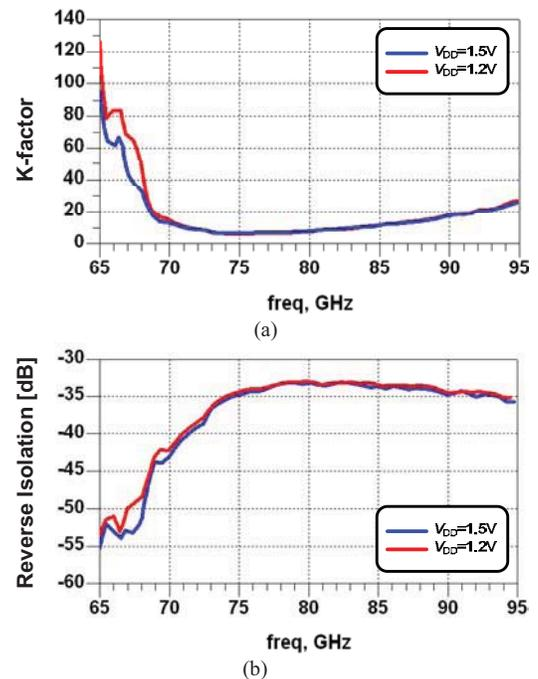
Fig. 7. Measured (a) K-factor and (b) reverse isolation of the power amplifier while  $V_{DD}$  is biased at 1.2 V and 1.5 V.
