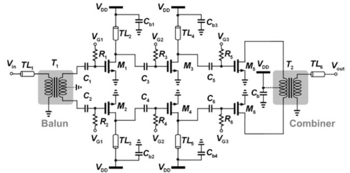
Fig. 1. Schematic diagram of the 77GHz power amplifier
