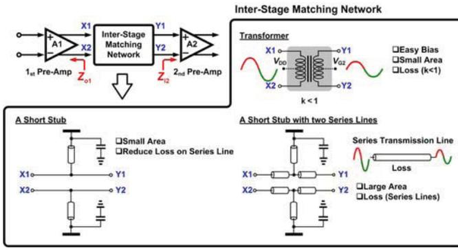
Fig. 2. Typical inter-stage matching networks.
