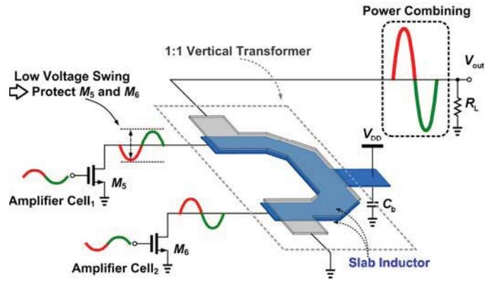
Fig. 3. The output matching network of the power amplifier.
