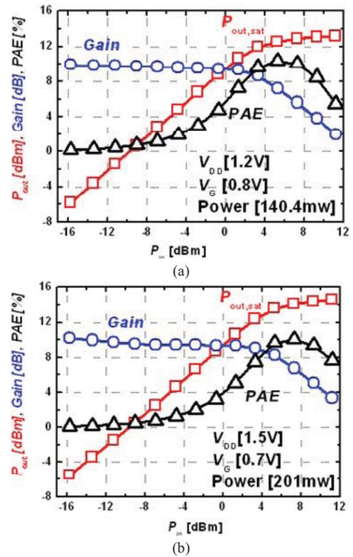
Fig. 6. Measured large-signal parameters of the power amplifier operating at (a) 1.2 V and (b) 1.5 V supply.
