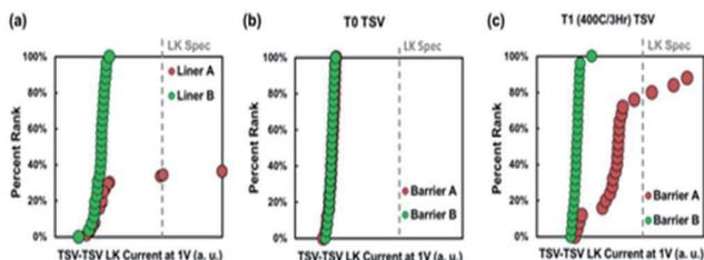
Fig. 3 TSV leakage dependent on (a) TSV liners, (b) TSV barriers, and (c) reliability dependency on the barrier after thermal torture.
