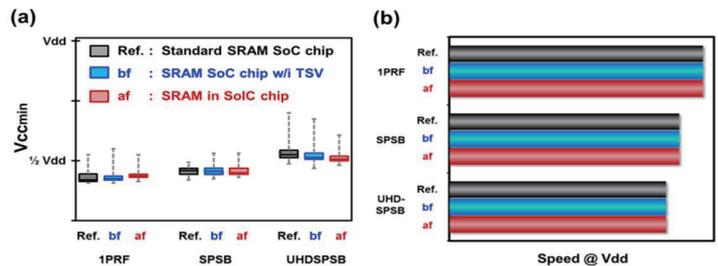
Fig. 9. (a) Vccmin and (b) Speed of SRAM compiler before and after SoIC 3D stacking. SRAM with 1PRF, SPSB, and UHDSB modes shows superior stability
