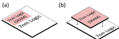
Fig. 1 Schematic pictorial view of (a) SoC before chip-partition, and (b) SoIC after chip-partition and stacking
