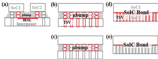
Fig. 2 Interconnect of five package structures: (a) 2.5D Interposer: uBump+1mm BEOL (b) 3D-IC F2B: uBump & TSV (c) 3D-IC F2F: uBump (d) SoIC F2B: SoIC bond & TSV (e) SoIC F2F: SoIC bond.
