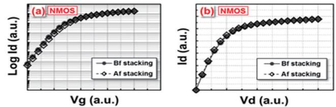
Fig. 5 NMOS (a) Id vs. Vg and, (b) Id vs. Vd before and after SoIC stacking
