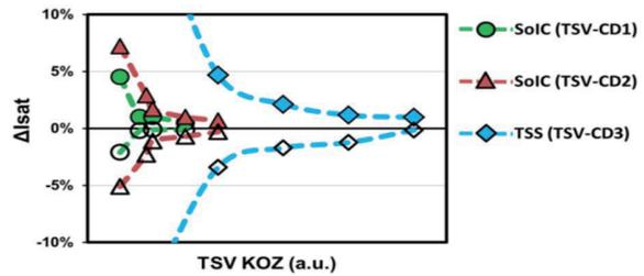
Fig. 4 Idsat characteristics of MOS device with different TSV sizes and KOZ
