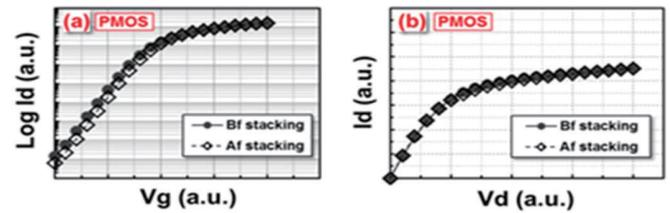
Fig. 6 PMOS (a) Id vs. Vg and, (b) Id vs. Vd not impacted by SoIC
