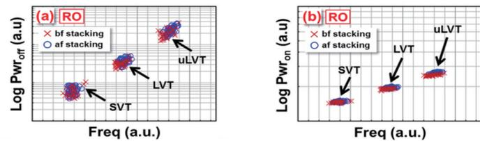
Fig. 8 (a) Off-power vs frequency (b) On-power vs frequency plot for ring oscillators are consistent before and after SoIC stacking
