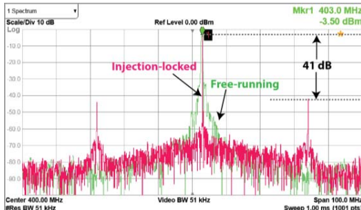
Fig. 8. Measured oscillator output spectrum in locked and unlocked states.
