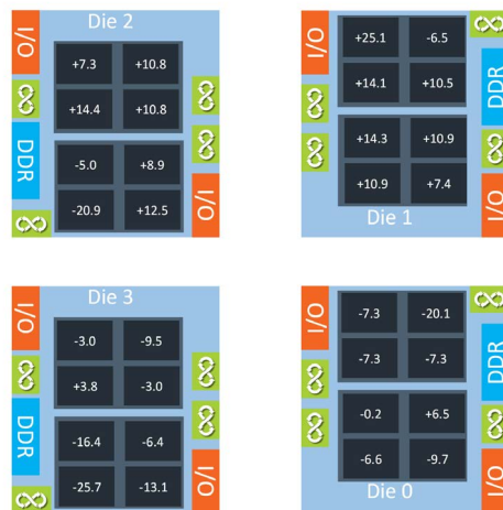
Figure 2.4.6: Measured variation in core voltage across SP3 package core locations.
