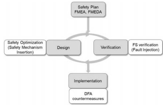
Figure 2. FS linked to the Design/Verification/Implementation flow
